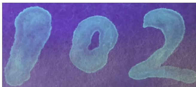
Fig. S11 The photographs writing "102" with HABr/CB[8]/0.005SR101 on the filter paper under UV light.
