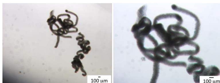
Figure S22. Optical microscopy images of DBS-CONH 2 gel filament portions (3.0% wt/vol; 30G blunt tip needle, 3.4 μL/min flow rate) after 30 days. Scale bars: 100 μm.
