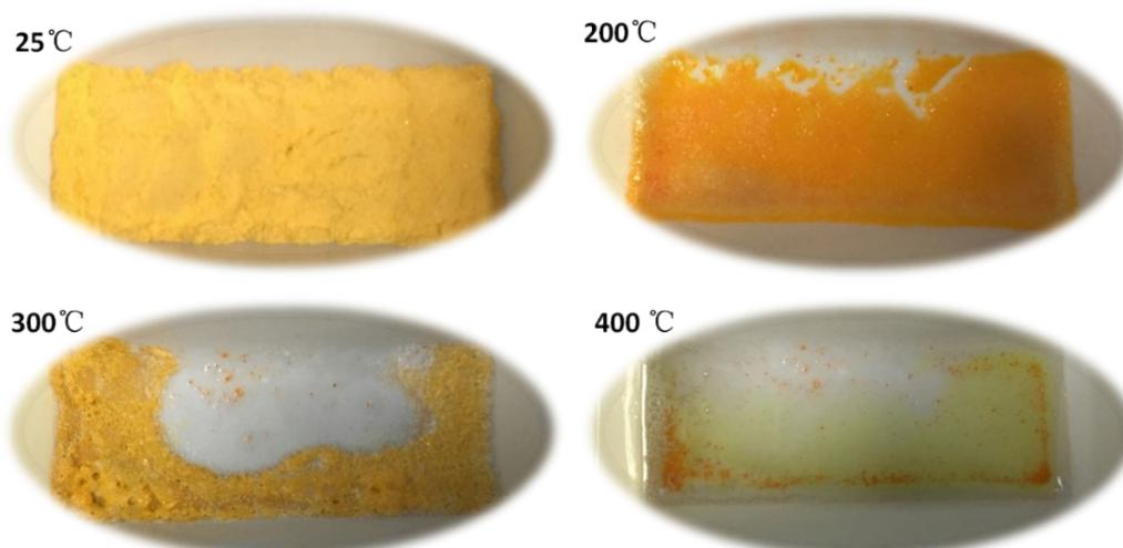
**Figure S2.** Photographs of the CsPbBr<sub>3</sub> and urea mixture under the different temperatures.
