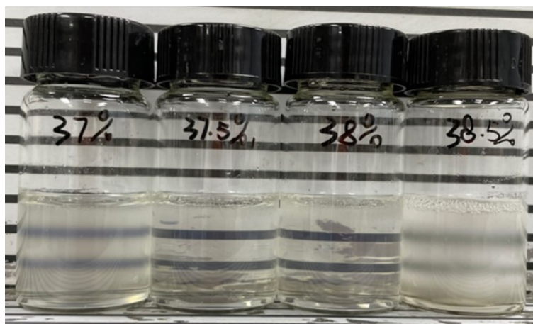
Figure S3. NaCas-stabilized transparent emulsion with different sucrose content. The refractive index of octane is about 1.3974 at 25 °C. When sucrose concentration is 37.5%, the refractive index of sucrose aqueous solution (water phase) is the same as that of octane (oil phase), so the emulsion is transparent. This finding are of interest for providing a facile strategy to fabricate biocompatible and highly transparent responsive emulsion with great potential in the food, healthcare and light-induced catalysis fields.
