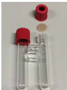
Figure S1. Small two-chamber reactor. Inner volume = 20 mL. Invented by the Skrydstrup group. [1]
