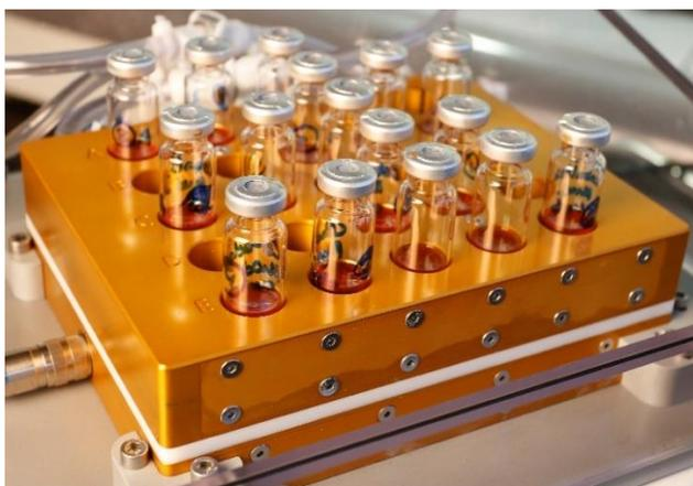
**Figure S. 1.** In-house developed parallel photoreactor.
