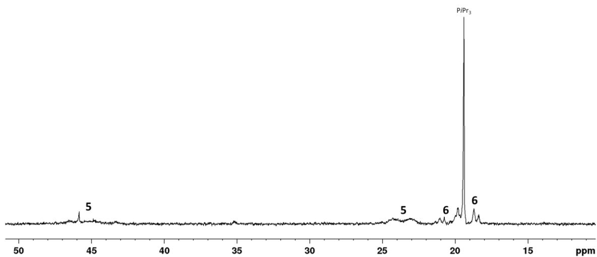
S47. ^{31}\text{P}\{^1\text{H}\} NMR spectrum of the reaction of complex [\text{Rh}(\text{F})(=\text{C}=\text{CHCF}_3)(\text{PiPr}_3)_2] ( 16 ) with \text{PEt}_3 in \text{C}_6\text{D}_6 .
