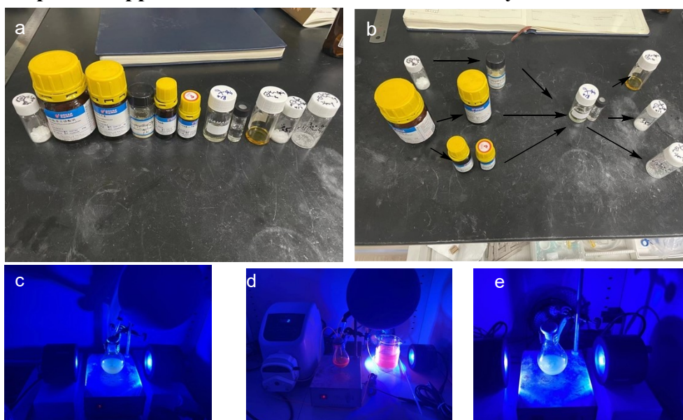
a)&b) Reagents and products in reactions; c) Gram-scale synthesis of 3i ; d) Gram-scale synthesis of 4a (continuous-flow); e) Gram-scale synthesis of 5a .
