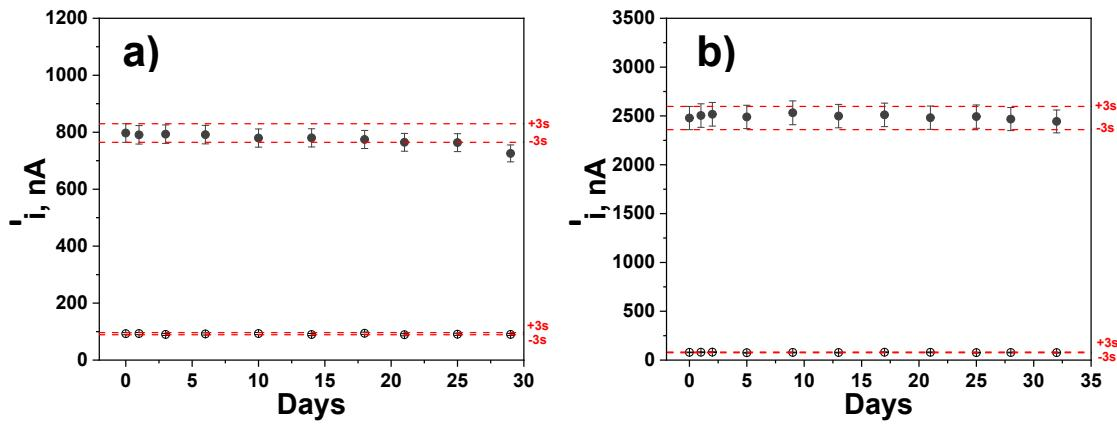
Fig. S4 Amperometric responses provided with the bioplatforms prepared from the stored OVA-MBs (at 4 °C in filtered PBS pH 7.4) in the absence (empty circles) and in the presence of 0.30 kU L<sup>-1</sup> IgE (a) and 0.036 µg L<sup>-1</sup> IgG4 (b) serum standard solutions (full circles). Control limits (red dashed lines) were calculated as  $\pm 3 \times$  mean values of three amperometric responses obtained the day of OVA-MBs preparation (day 0).
