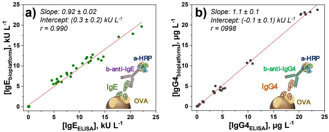
Fig. S6 Correlation plots for the concentrations of OVA-specific IgE (a) and IgG4 (b) in the analysed serum samples (replicates included in the plot) obtained with the developed electrochemical bioplatforms and the ELISA method. Red lines: regression lines with  $r$  = Pearson regression coefficient.
