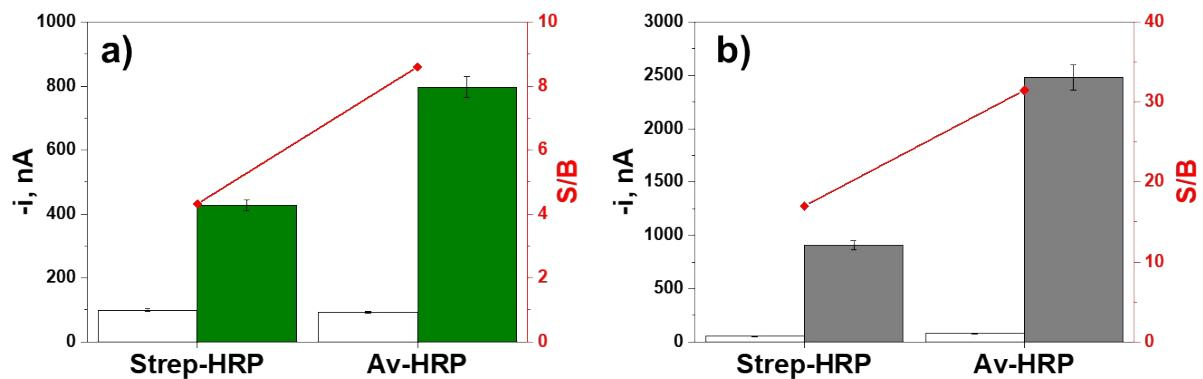
Fig. S3 Amperometric responses (and corresponding S/B ratios) measured with the prepared bioplatforms for the single determination of IgE (a) or IgG4 (b) in the absence (empty bars, B) and in the presence of  $0.30 \text{ kU L}^{-1}$  IgE or  $0.036 \mu\text{g L}^{-1}$  IgG4 (full bars, S) serum standard solutions using enzyme labelling of the magnetic bioconjugates with Strep-HRP or Av-HRP.
