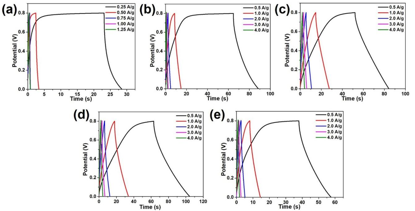
**Figure S5:** GCD curves of (a) NFO (b) MS (c) MN1 (d) MN5 and (e) MN10
