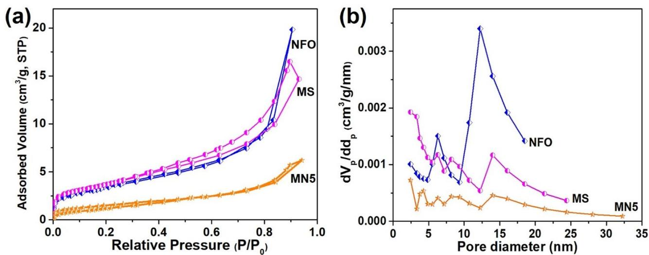
**Figure S3:** (a) Typical nitrogen adsorption-desorption isotherms (b) pore size distributions obtained using BJH method
