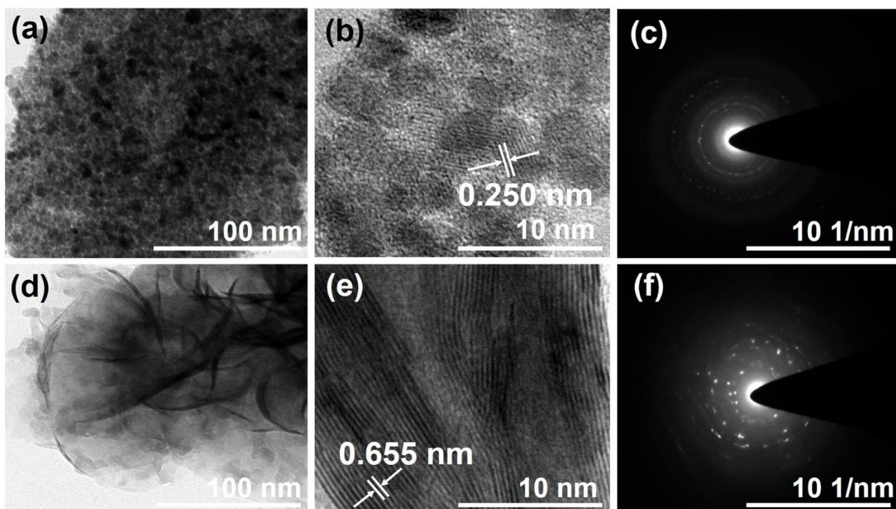
**Figure S2:** (a) Low (b) High resolution TEM images and (c) SAED pattern of NFO nanoparticles (d) Low (e) High resolution TEM images and (f) SAED pattern of MS nanoflowers
