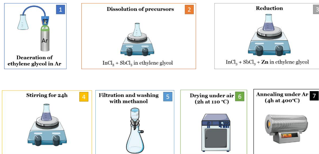
Figure S1. Schematic description of the reduction synthesis process for the InSb or Sb powders.
