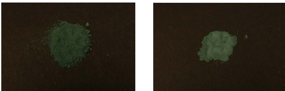
Fig. S5. Photographs of P25/Pt/1 before (left) and after (right) 30 h of photoirradiation.
