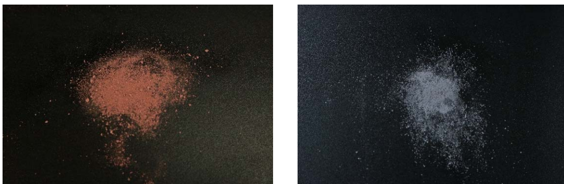
Fig. S6. Photographs of P25/Pt/2 before (left) and after (right) 10 h of photoirradiation.
