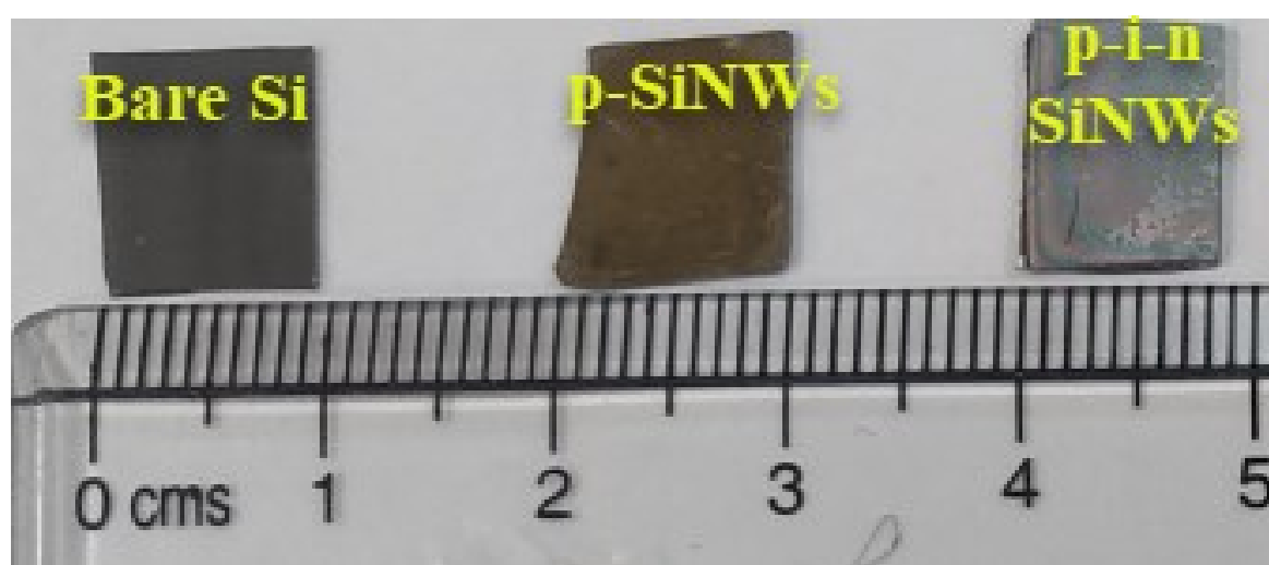
Fig. S1 The optical photograph of bare Si, p-SiNWs, and p-i-n SiNWs which have been further utilized for the fabrication of Photocathodes having a dimension of \sim (1 \times 1) \text{ cm}^2 .
