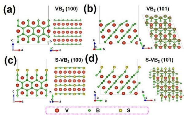
**Fig. S2.** Top and side views of the  $\text{VB}_2$  (100) facets (a), and (101) facets (b), respectively. Top and side views of the passivated  $\text{VB}_2$  (100) facets with sulfur atoms (c), and (101) facets with sulfur atoms (d), respectively.
