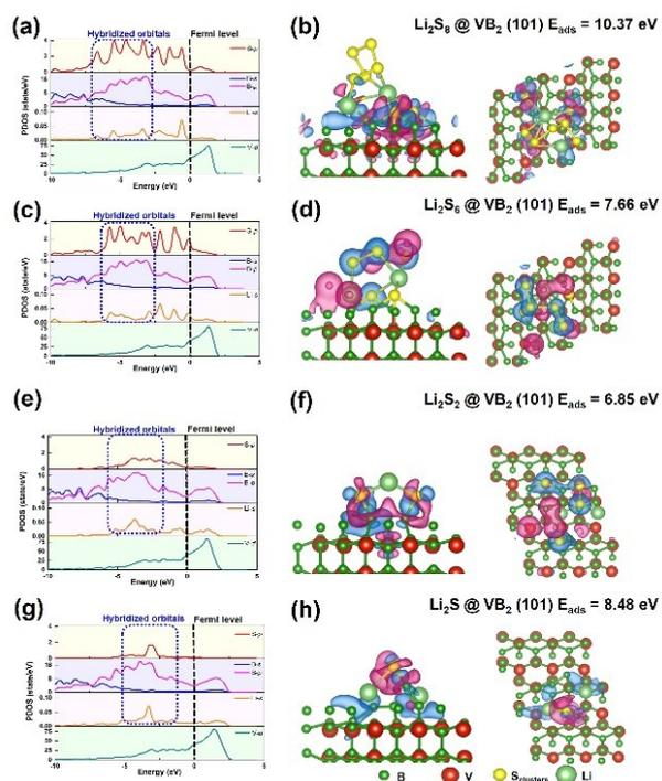
**Fig. S3.** Density functional theory calculations of the PDOS, side and top views of charge density difference of  $\text{Li}_2\text{S}_8$  (a, b),  $\text{Li}_2\text{S}_6$  (c, d),  $\text{Li}_2\text{S}_2$  (e, f) and  $\text{Li}_2\text{S}$  (g, h) molecules adsorbed on the pure  $\text{VB}_2$  (101) facets. The blue and pink areas are the regions of trapped and lost charge.
