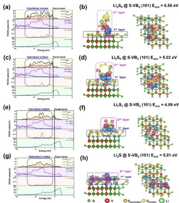
**Fig. S4.** Density functional theory calculations of the PDOS, side and top views of charge density difference of  $\text{Li}_2\text{S}_8$  (a, b),  $\text{Li}_2\text{S}_6$  (c, d),  $\text{Li}_2\text{S}_2$  (e, f) and  $\text{Li}_2\text{S}$  (g, h) molecules adsorbed on the passivated  $\text{VB}_2$  (101) facets. The blue and pink areas are the regions of trapped and lost charge.
