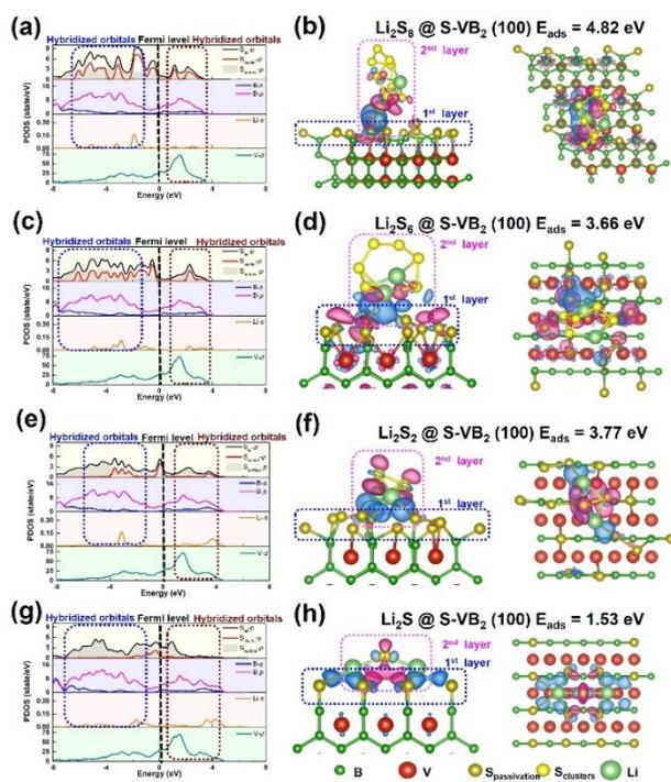
**Fig. S6.** Density functional theory calculations of the PDOS, side and top views of charge density difference of  $\text{Li}_2\text{S}_8$  (a, b),  $\text{Li}_2\text{S}_6$  (c, d),  $\text{Li}_2\text{S}_2$  (e, f) and  $\text{Li}_2\text{S}$  (g, h) molecules adsorbed on the passivated  $\text{VB}_2$  (100) facets. The blue and pink areas are the regions of trapped and lost charge.
