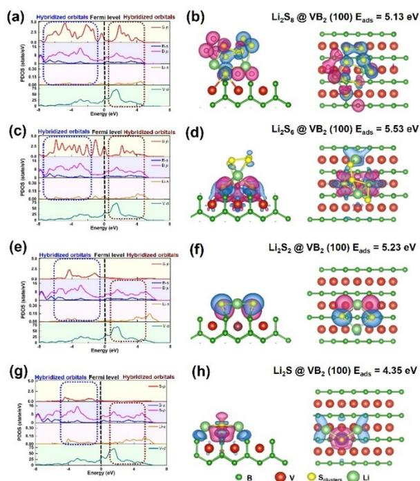
**Fig. S5.** Density functional theory calculations of the PDOS, side and top views of charge density difference of  $\text{Li}_2\text{S}_8$  (a, b),  $\text{Li}_2\text{S}_6$  (c, d),  $\text{Li}_2\text{S}_2$  (e, f) and  $\text{Li}_2\text{S}$  (g, h) molecules adsorbed on the pure  $\text{VB}_2$  (100) facets. The blue and pink areas are the regions of trapped and lost charge.
