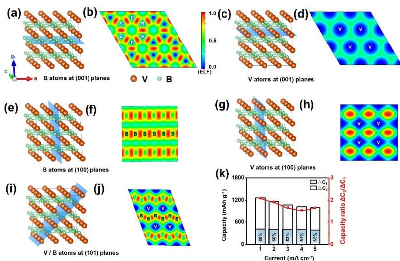
**Fig. S1.** Crystal structure and electron location function of  $\text{VB}_2$  with B atoms at (001) planes (a-b), V atoms at (001) planes (c-d), B atoms at (100) planes (e-f), V atoms at (100) planes (g-h), and V and B atoms at (101) planes (i-j), respectively. The corresponding ratios (k) of  $\Delta C_2/\Delta C_1$  from 1 to 5  $\text{mA cm}^{-2}$
