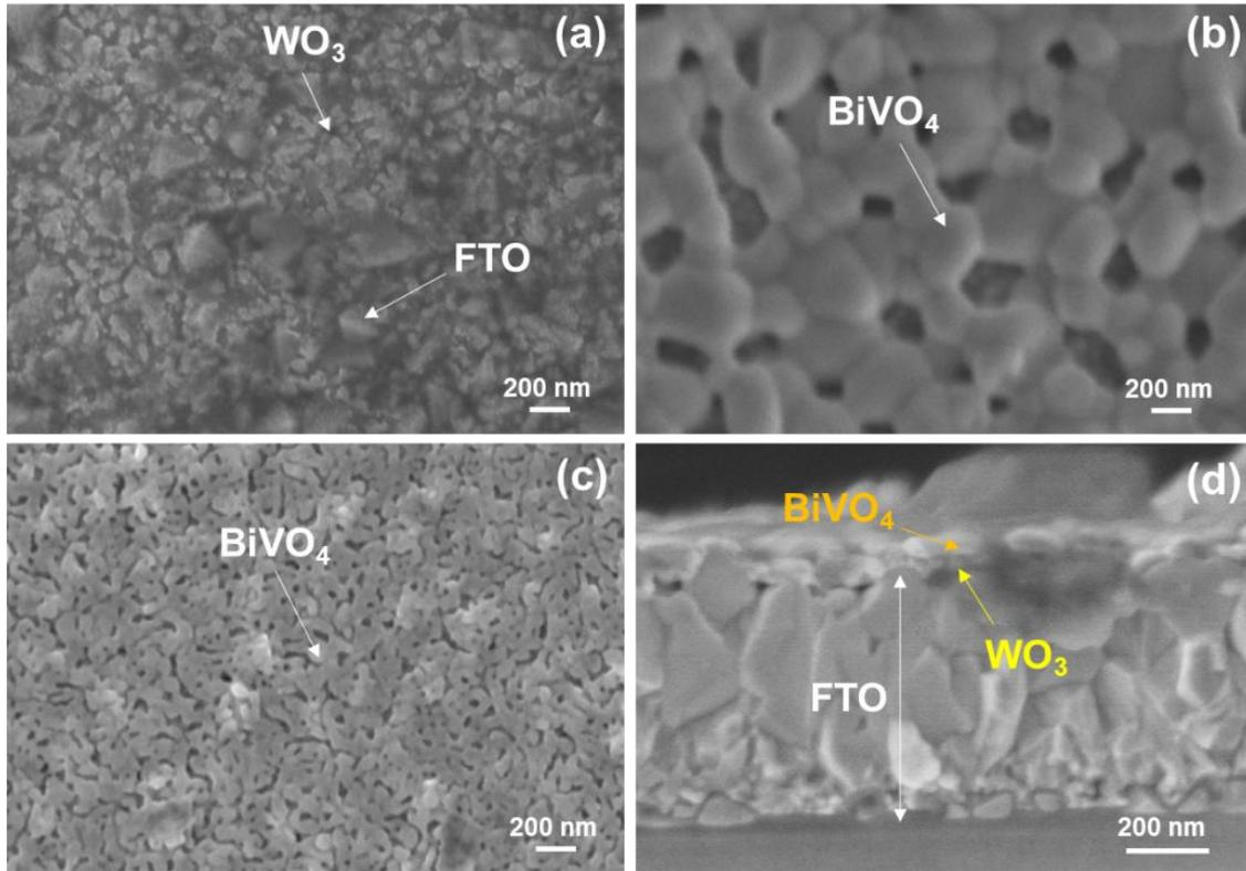
**Fig. S12.** SEM images of (a) WO<sub>3</sub>/FTO, (b) BiVO<sub>4</sub>/FTO and (c) BiVO<sub>4</sub>/WO<sub>3</sub>/FTO; (d) cross-section SEM image of BiVO<sub>4</sub>/WO<sub>3</sub>/FTO prepared using spin coating method.
