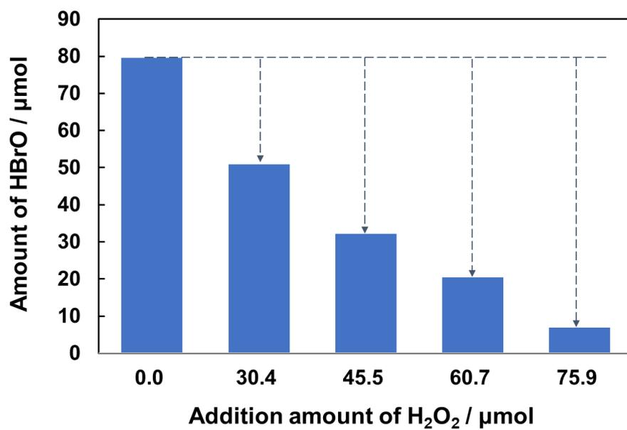
**Fig. S4.** Amount of HBrO after adding various amount of H<sub>2</sub>O<sub>2</sub> under dark condition. The
