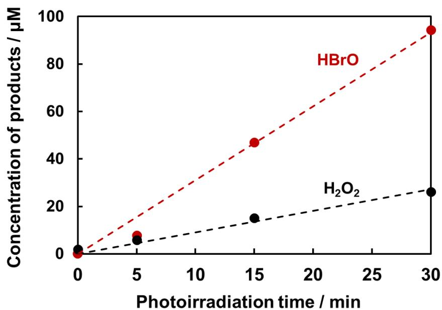
**Fig. S6.** Concentration of HBrO produced on the  $\text{BiVO}_4/\text{WO}_3/\text{FTO}$  photoanode and  $\text{H}_2\text{O}_2$  produced on the Pt/FTO cathode in a two-compartment cell without applied voltage under solar light irradiation. System: two-electrode system; electrolyte: 0.5 M NaBr aqueous solution, 35 mL; light source: simulated solar light (AM-1.5, 1 SUN).
