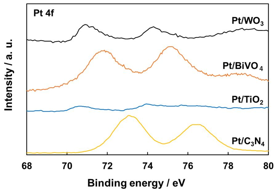
**Fig. S1.** XPS spectra of Pt 4f in various Pt/photocatalysts.
