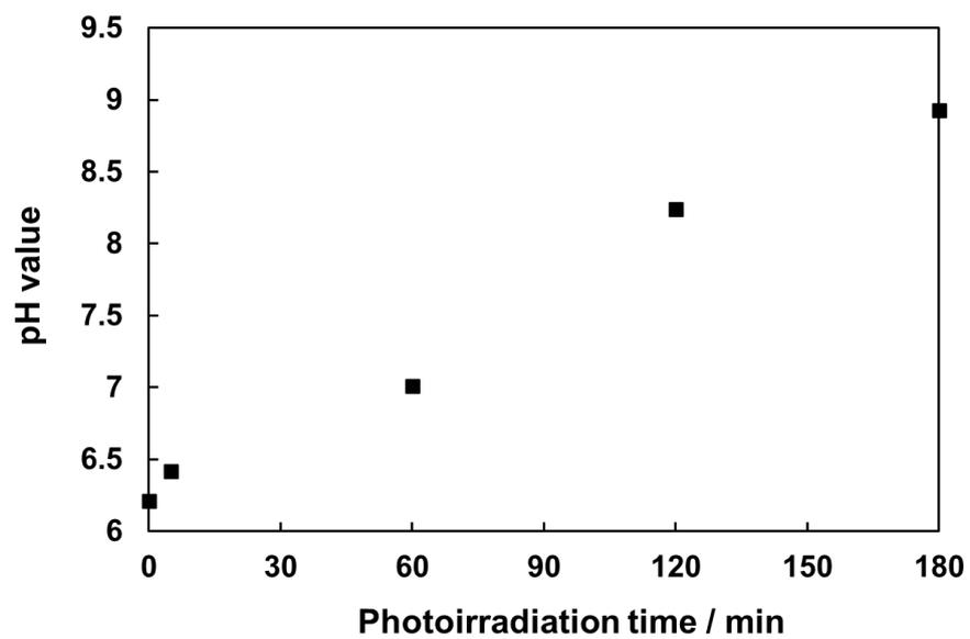
**Fig. S7.** The change of pH during the photocatalytic oxidation of Br<sup>-</sup> on the Pt-BiVO<sub>4</sub>/WO<sub>3</sub>/FTO photocatalyst sheet under simulated solar light irradiation for 180 min.
