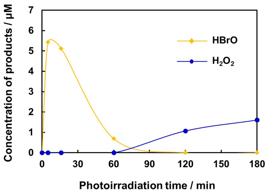
**Fig. S5.** The concentration of HBrO and  $\text{H}_2\text{O}_2$  produced over the Pt/ $\text{BiVO}_4$  in an aqueous solution of NaBr under simulated solar light for 180 min. Photocatalyst amount: 50 mg; Pt cocatalyst amount: 1.0 wt% of photocatalyst; reaction solution: 0.5 M NaBr, 50 mL;  $\text{O}_2$  flow rate:  $1 \text{ mL min}^{-1}$ ; light source: simulated solar light (AM-1.5, 1 SUN); irradiation area: approximately  $20 \text{ cm}^2$ ; temperature: 303 K.
