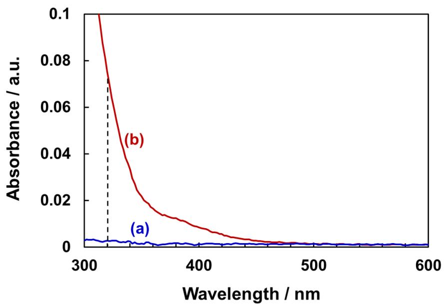
**Fig. S9.** Absorption spectra of (a) NaBr and (b) NaBr + HBrO aqueous solution. The concentrations of NaBr and HBrO are 0.5 M and 80  $\mu$ M, respectively.
