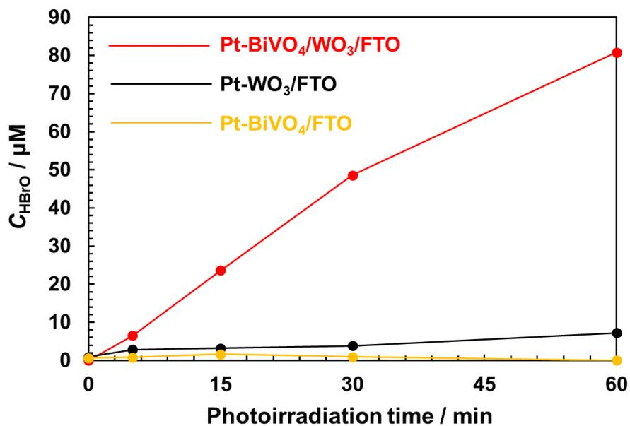
**Fig. S10.** HBrO concentration produced during the photocatalytic oxidation of Br<sup>-</sup> over the Pt-BiVO<sub>4</sub>/WO<sub>3</sub>/FTO, Pt-WO<sub>3</sub>/FTO and Pt-BiVO<sub>4</sub>/FTO photocatalyst sheets under simulated solar light irradiation. Reaction solution: 0.5 M NaBr, 50 mL; O<sub>2</sub> flow rate: 1 mL min<sup>-1</sup>; light source: simulated solar light (AM-1.5, 1 SUN); temperature: 303 K; photoirradiation time: 60 min.
