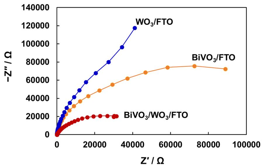
**Fig. S11.** Nyquist plots for WO<sub>3</sub>/FTO, BiVO<sub>4</sub>/FTO, and BiVO<sub>4</sub>/WO<sub>3</sub>/FTO photoelectrodes in 0.5 M NaBr aqueous solution under simulated solar light illumination.
