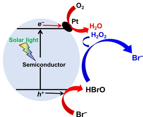
**Fig. S2.** Schematic illustration of reaction mechanism for the production and accumulation of HBrO over the Pt/semiconductor photocatalyst under solar light irradiation.
