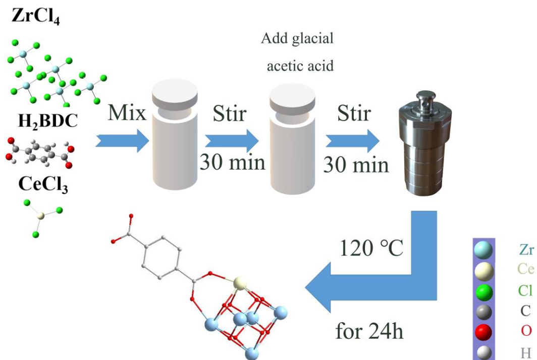
Figure S13. Synthesis of the 15%Ce-UiO-66
