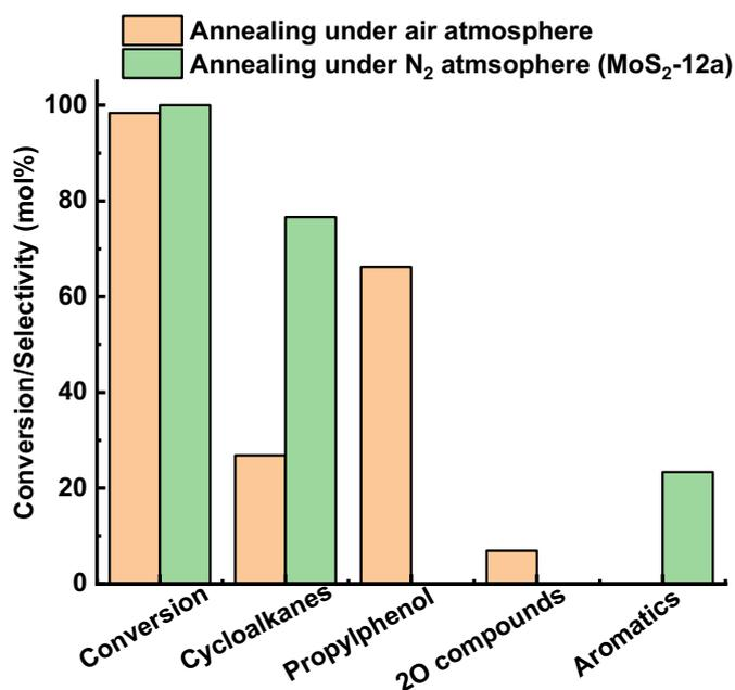
Figure S5 Comparison of PG conversion and product selectivity for HDO of PG over MoS<sub>2</sub>-24 following an annealing treatment under different atmosphere (air or N<sub>2</sub>) at 400 °C for 2 h. Reaction conditions: 50 bar total H<sub>2</sub> pressure, 300 °C, and 1000 rpm.
