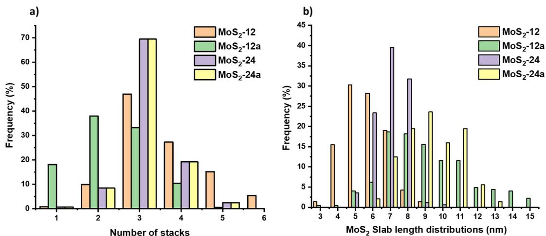
Figure S4a) Distribution of the number of stacks and b) MoS<sub>2</sub> slab length for different unsupported MoS<sub>2</sub>.
