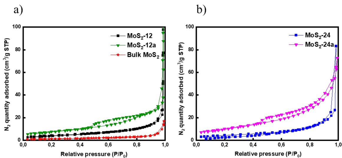
Figure S2 Nitrogen adsorption-desorption isotherms for studied catalysts.
