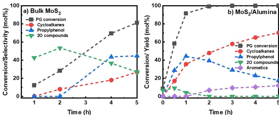
Figure S6 Reaction product distribution for HDO of PG over a) Bulk MoS<sub>2</sub> b) 13.2 wt% MoS<sub>2</sub> supported on alumina at 50 bar total H<sub>2</sub> pressure, 300 °C and 1000 rpm.
