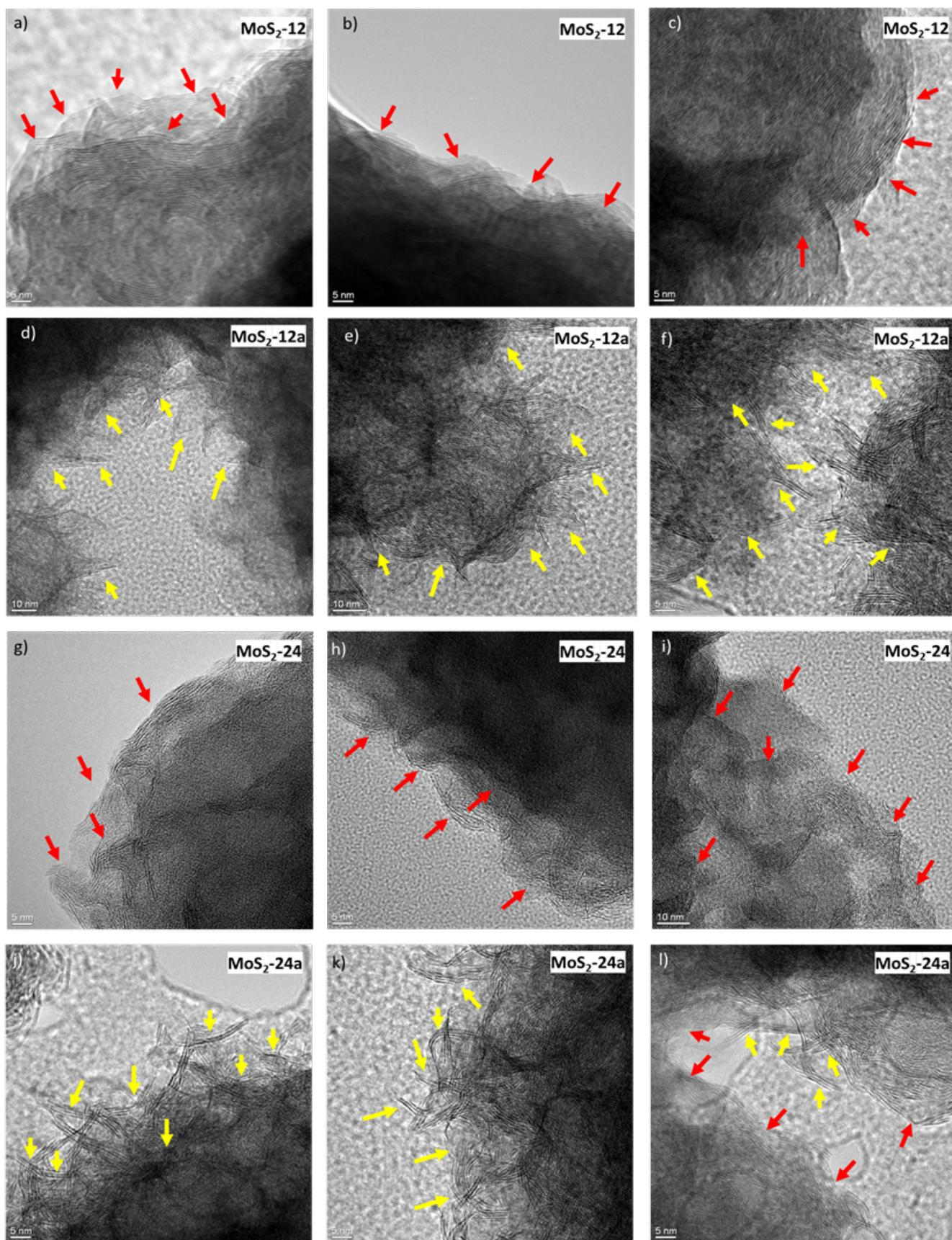
Figure S3 Additional HRTEM images of a-c) MoS<sub>2</sub>-12, d-f) MoS<sub>2</sub>-12a, g-i) MoS<sub>2</sub>-24, and j-l) MoS<sub>2</sub>-24a.
