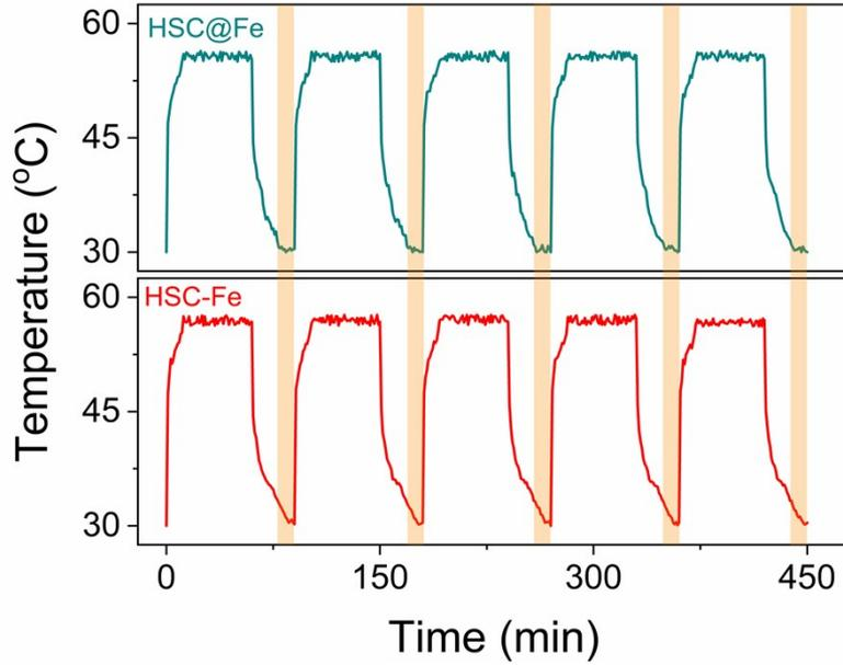
**Fig. S8** Surface temperature of HSC-Fe and HSC@Fe under 1 kW/m<sup>2</sup> solar irradiation on the water.
