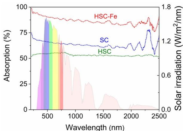
Fig. S6 UV-Vis-NIR absorption spectra of HSC-Fe, HSC and SC in wetting state.
