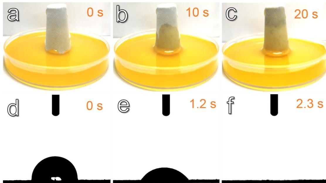
**Fig. S3** (a-c) Water transport properties of gauze wrapped PS foam, (b) hydrophilicity of LAR.
