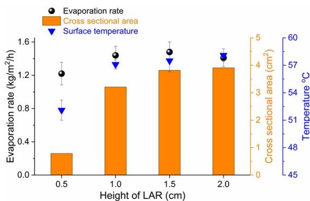
Fig. S1 Evaporation rate, cross sectional area and surface temperature during solar steam generation of generators with different height of LAR (the angle of incident light is 90 °).
