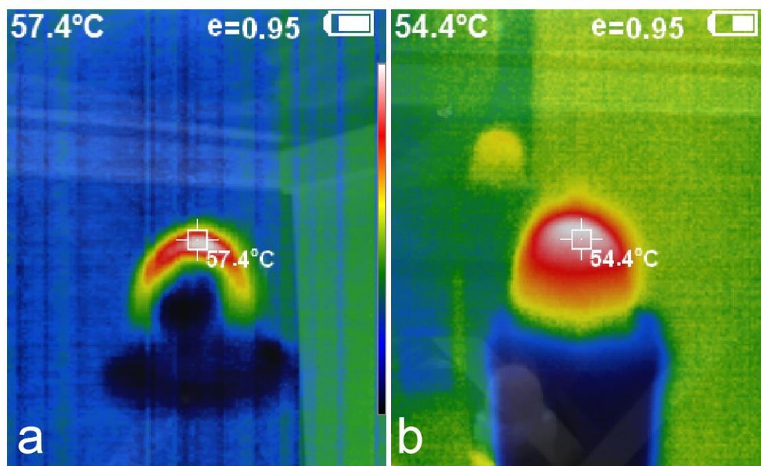
**Fig. S9** IR image of (a) HSC-Fe and (b) HSC@Fe under  $1 \text{ kW/m}^2$  solar irradiation on the water.
