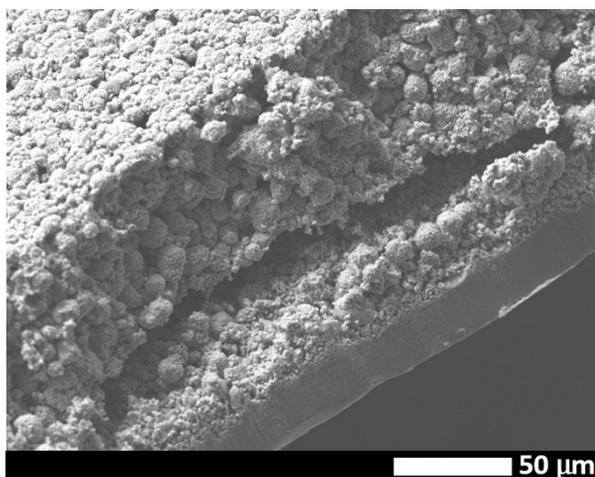
Figure S6: Cross section of the partially delaminated polycrystalline NMC622 electrode after cell failure (after 73 cycles).
