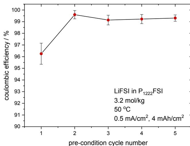
Figure S5: Coulombic efficiency vs cycle number for Li || Cu cells during pre-conditioning stage. At least 5 cycles were needed for consistent stabilisation of the copper substrate prior to measuring the average coulombic efficiency of Li metal.
