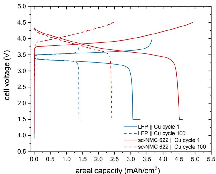
Figure S3: voltage profiles for LFP || Cu cell (blue) and sc-NMC622 || Cu cell (red) for 1st cycle (solid line) and 100<sup>th</sup> cycle (dash line)
