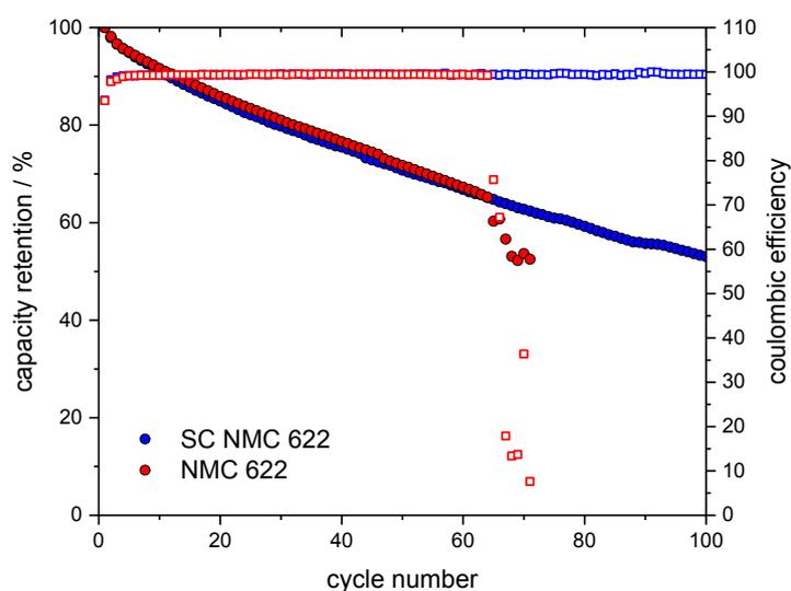
Figure S2: Capacity retention and coulombic efficiency for polycrystalline NMC 622 || p-Cu (red) and single crystal NMC 622 || p-Cu (blue) at C/2 (1.75 mA/cm<sup>2</sup>) and 100 cycles at 50 °C. Polycrystalline cells started to fail after 65 cycles.
