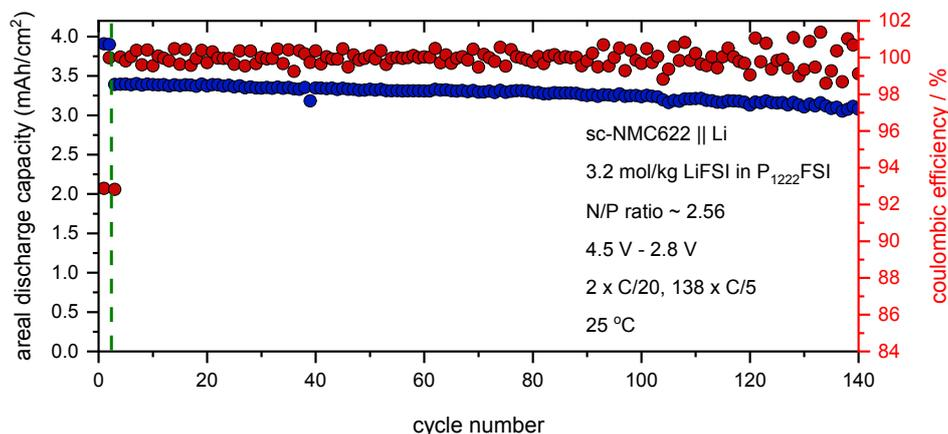
Figure S4: areal discharge capacity and coulombic efficiency for sc-NMC 622 || Li at 25 °C. Li foil thickness 50  $\mu\text{m}$ . The cells were cycled with 2 formation cycles at C/20 and C/5 for 138 cycles. Capacity retention 90.7% and average coulombic efficiency 99.92% (excluding formation cycles)
