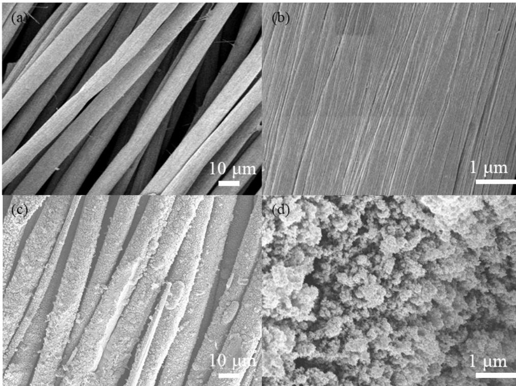
Figure S5. SEM images of carbon cloth before (a, b) and after (c, d) DLW under 20% laser power
