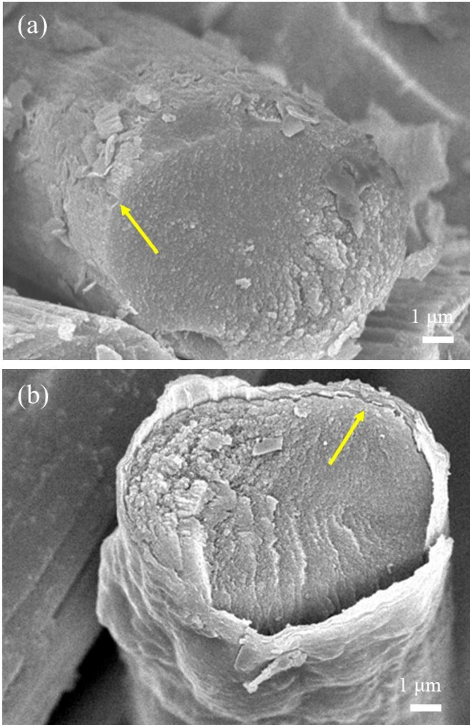
Fig.S6. The interfaces (LCE40) between carbon fiber and lignin-derived carbon (The carbon chips found on sample are caused by carbon fracture from scissors cutting).
