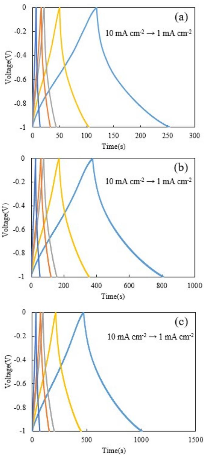
Figure S8. All plots are based on data from three-electrode system. GCD curves at 1, 2, 4, 5, 10  $\text{mA cm}^{-1}$  for LCE20 (a), LCE30 (b), and LCE50 (c).
