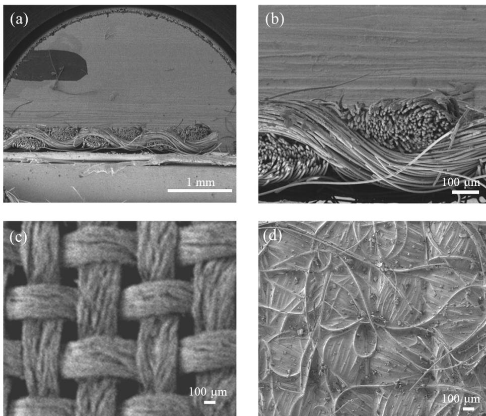
Figure S1. SEM images of (a, b) side view of original carbon cloth; (c) top view of original carbon cloth; (d) top view of carbon cloth after covering by molten lignin.
