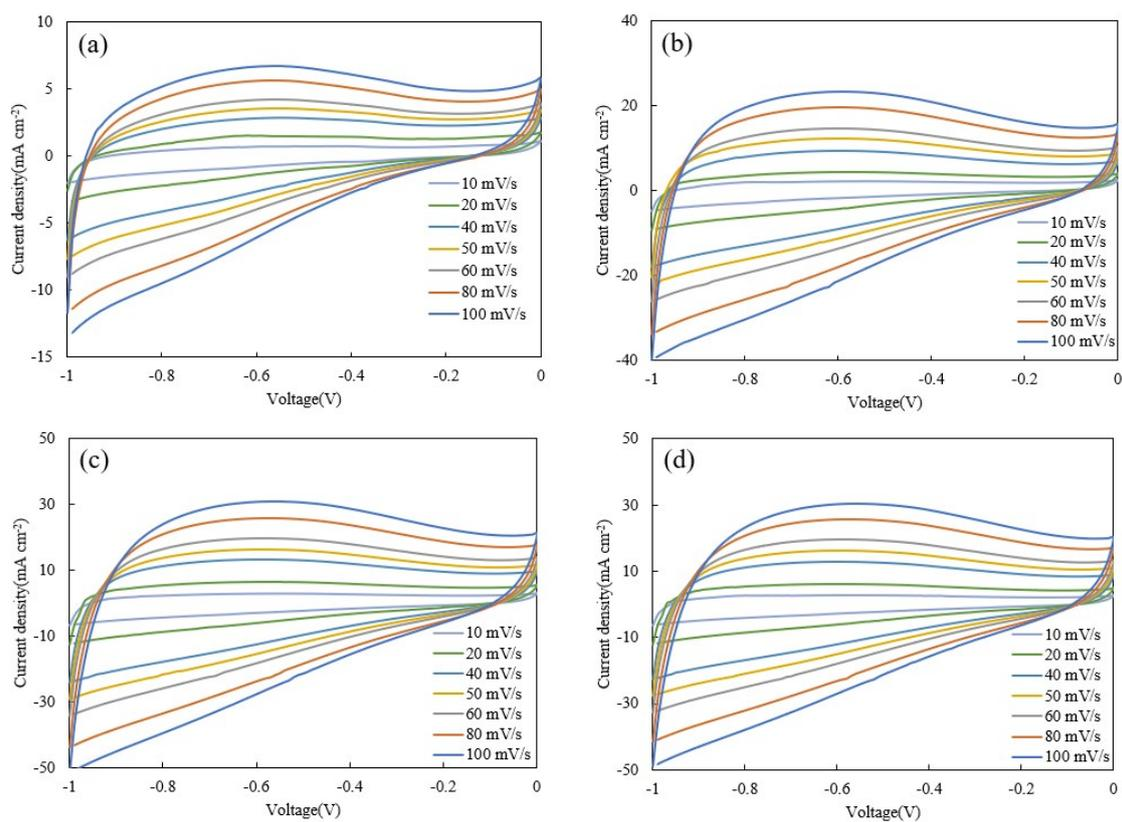
Figure S7. All plots are based on data from three-electrode system. CV curves at 10 - 100 mV s<sup>-1</sup> for (a) LCE20, (b) LCE30, (c) LCE40, and (d) LCE50.
