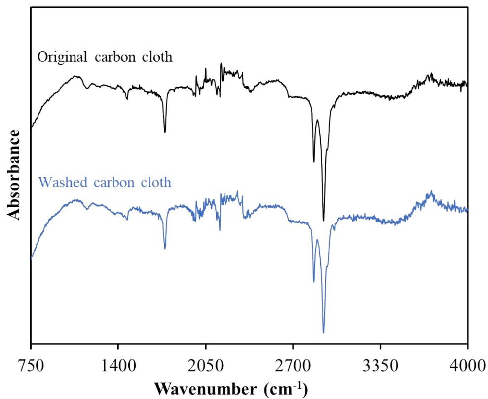
Figure S4. FTIR spectra of original carbon cloth and carbon cloth after melting of lignin and washing by 2M KOH solution.
