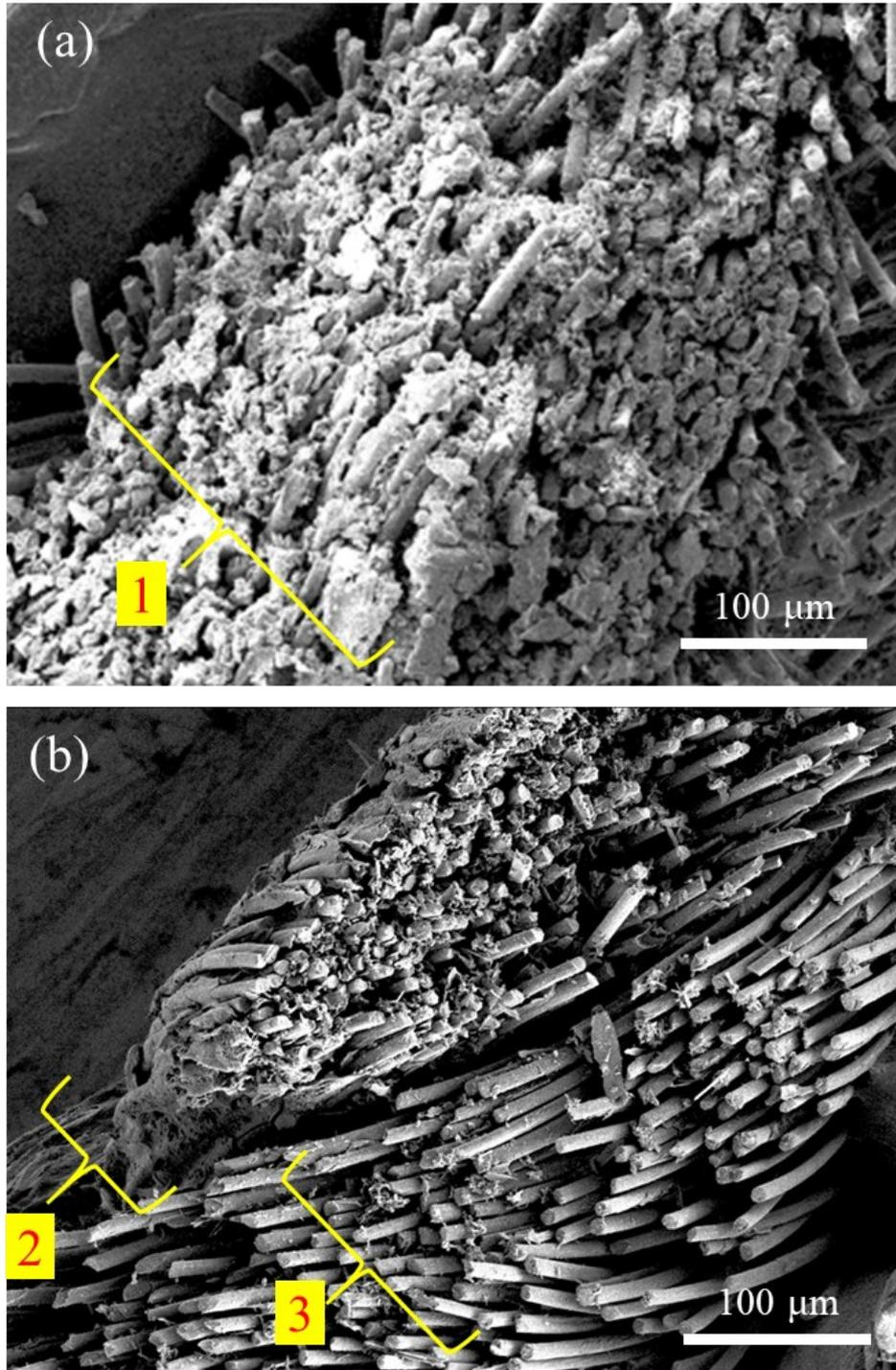
Fig.S3. Cross-section SEM images of (a) lignin melting on carbon cloth (it can be seen from region 1 that lignin melted and penetrated to the whole carbon cloth through the holes between carbon fibers); (b) LCE40 (it can be seen from region 2 that the lignin bonded on carbon cloth upon DLW and cannot be washed off, while region 3 stay untouched under DLW and the lignin was washed off).
