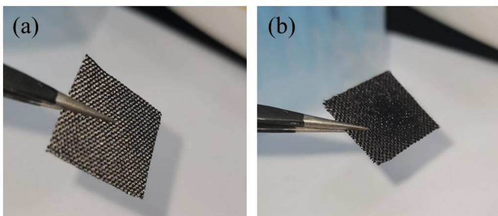
Figure S2. Photographs of (a) original carbon cloth; and (b) carbon cloth covering with melted lignin.
