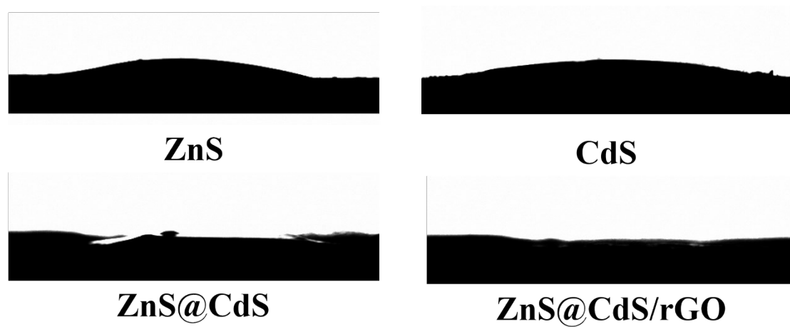
Fig. S5. Contact angle test of ZnS, CdS, ZnS@CdS and ZnS@CdS/rGO photocatalyst.
