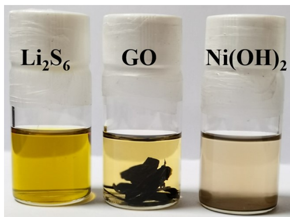
Fig. S9. Static adsorption experiments of Li 2 S 6 with pristine Ni(OH) 2 and GR.
