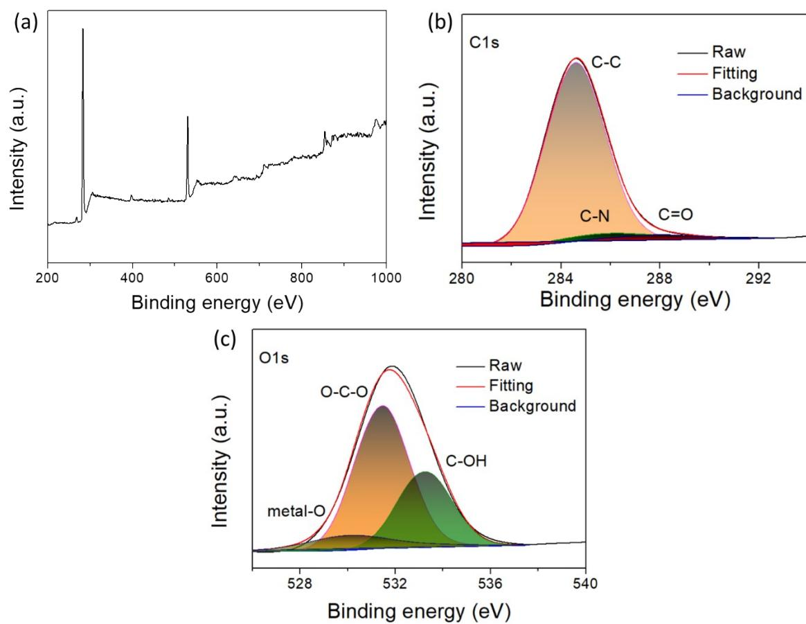
Figure S6. XPS spectra of the NF13 (a) survey scan, (b) C1s and (c) O1s.
