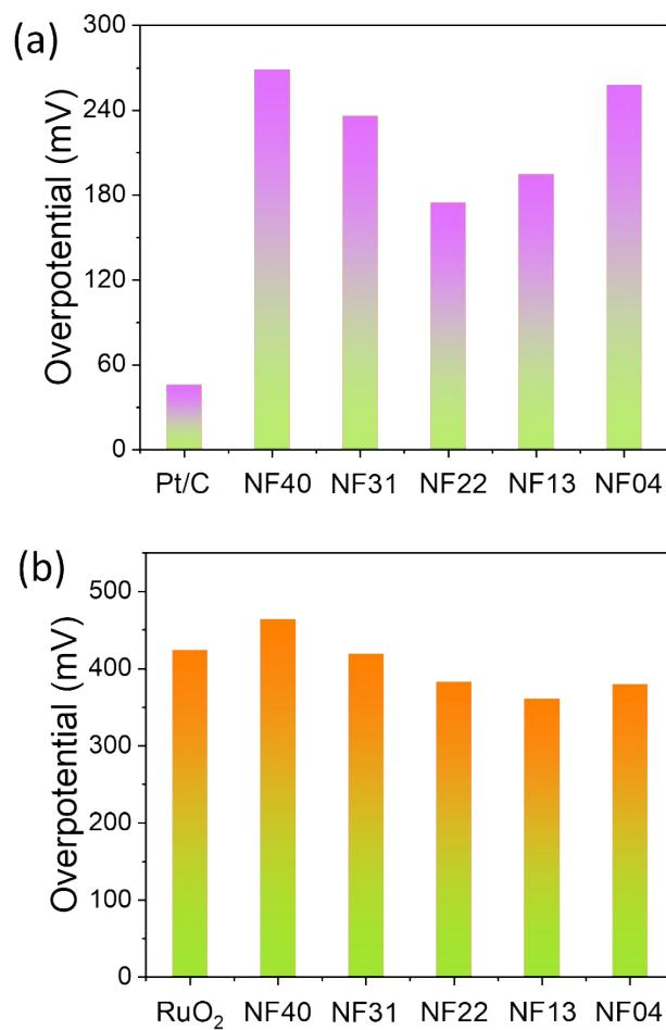
Figure S8. Overpotential of prepared samples and commercial catalysts at the current density of 20 mA/cm<sup>2</sup>.
