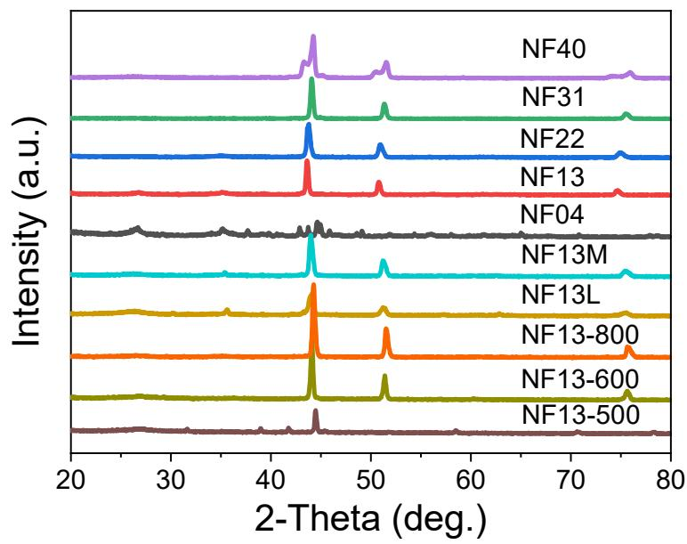
Figure S13. XRD patterns of all samples with different experimental conditions.
