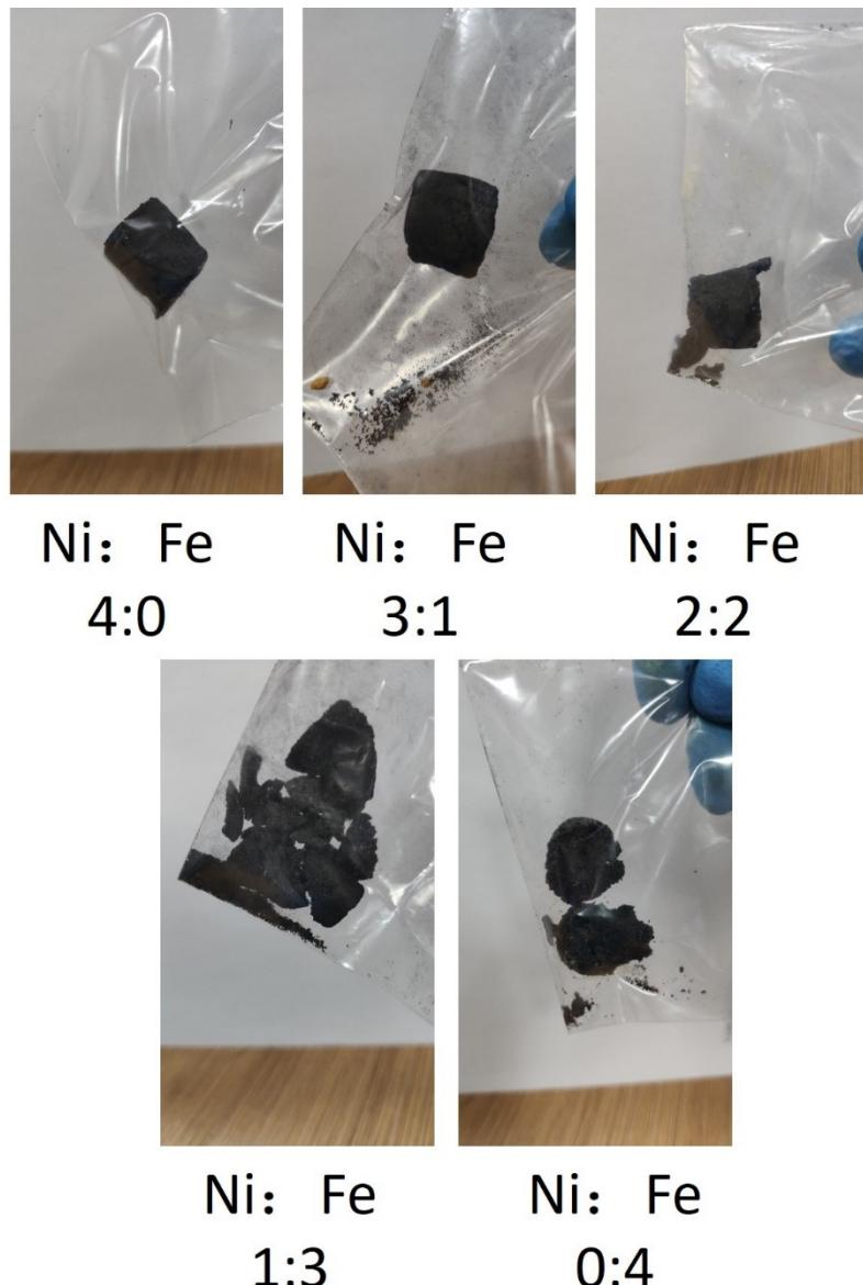
Figure S2. Optical photograph of carbon aerogels with different Ni/Fe ratio.
