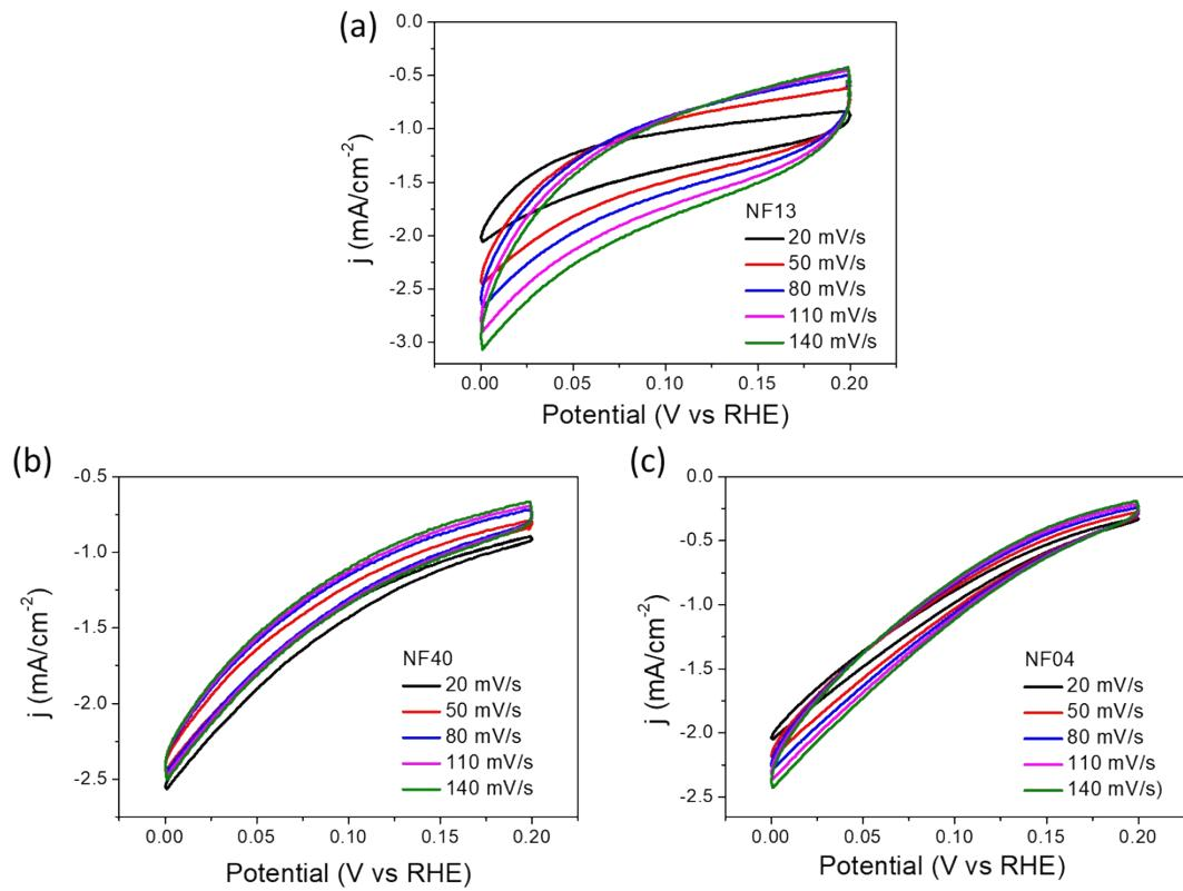
Figure S9. CV conducted at potential from 0 V to 0.2 V vs RHE at scan rates of 20 mV/s, 50 mV/s, 80 mV/s, 110 mV/s and 140 mV/s.
