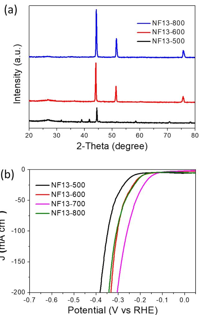
Figure S12. XRD (a) and HER performance (b) of samples with different carbonization temperatures.
