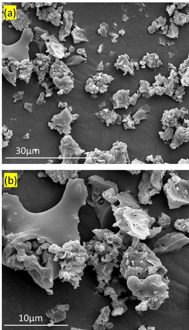
Figure S14. SEM images of catalyst after 100h long-term stability test.
