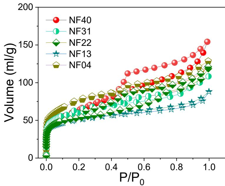
Figure S5. The nitrogen adsorption-desorption isotherms NF40, NF31, NF22, NF13 and NF04.
