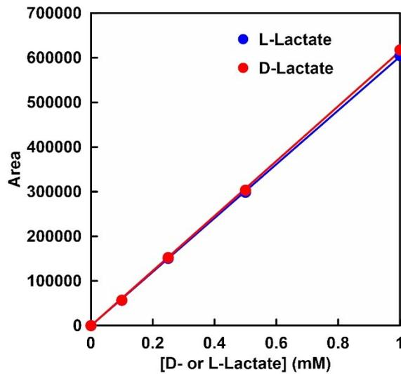
Figure S3. Relationship between the L- and D- lactate concentration and the detection peak area.
