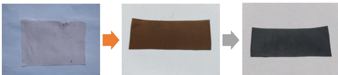
Figure S2. The photographs of the membrane after electrospun, presinter and further carbonization.
