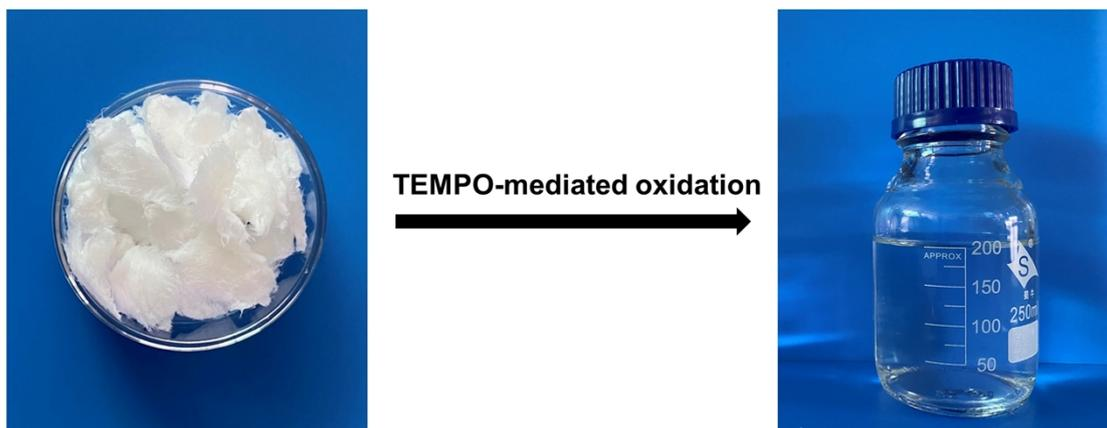
**Fig. S5.** Transparent CNF suspension deriving from bleached softwood pulp was prepared by TEMPO-mediated oxidation process.
