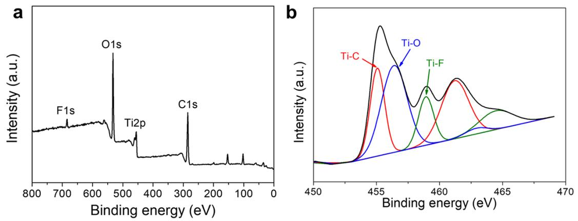
**Fig. S4.** X-ray photoelectron spectroscopy (XPS) characterization of MXene membrane. a) XPS survey spectrum and b) high-resolution Ti2p spectrum of MXene, which clearly show the presence of oxygen and fluorine, indicating the existence of -OH and -F surface groups.
