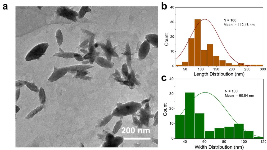
**Fig. S2.** (a)The Cryo-EM image of MXene nanosheets. The (b) length and (c) width of 100 MXene nanosheets were analyzed and counted according to Cryo-EM images.
