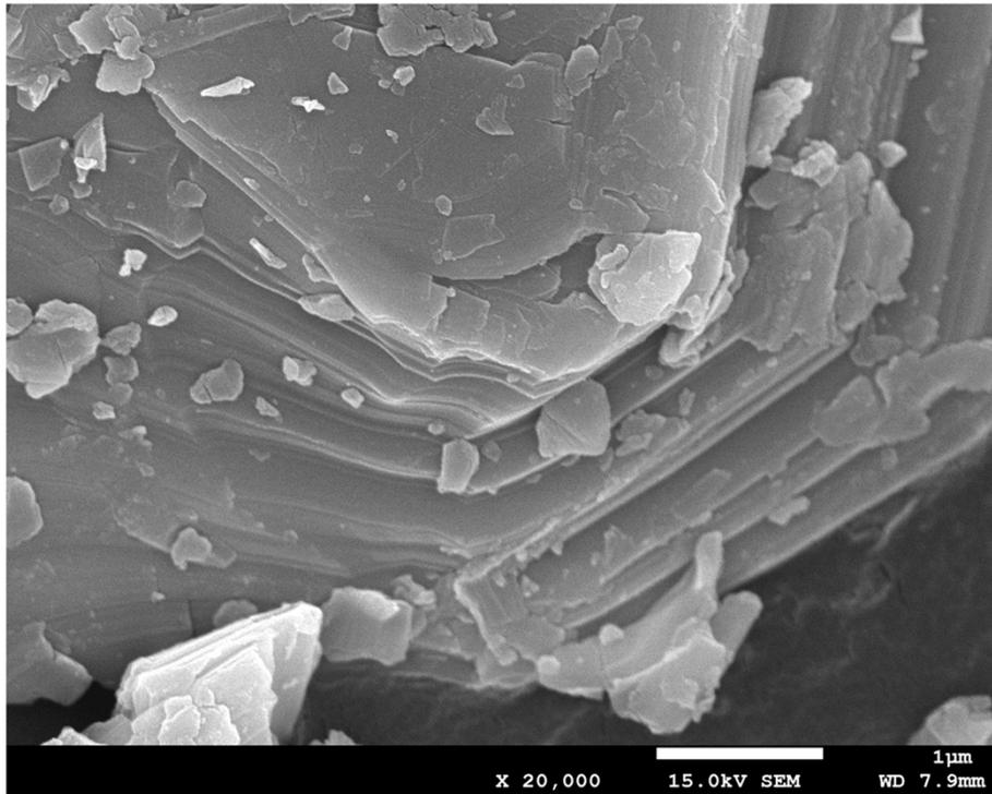
**Fig. S1.** The SEM image of MAX phase  $\text{Ti}_3\text{AlC}_2$  powder.
