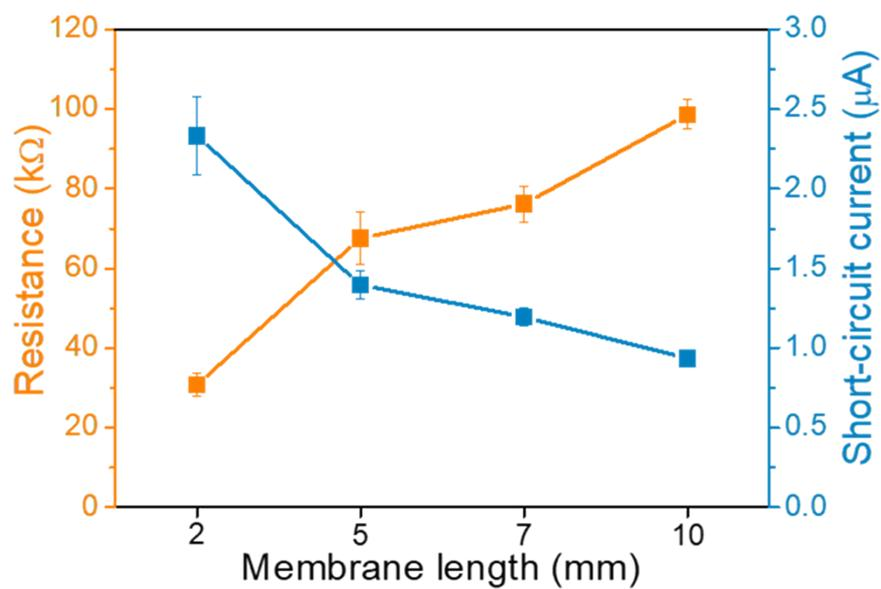
**Fig. S11.** Resistance and short-circuit current of membrane (50% CNF) with width of 5 mm and lengths of 2 mm, 5 mm, 7 mm and 10 mm under 1000-fold concentration gradient.
