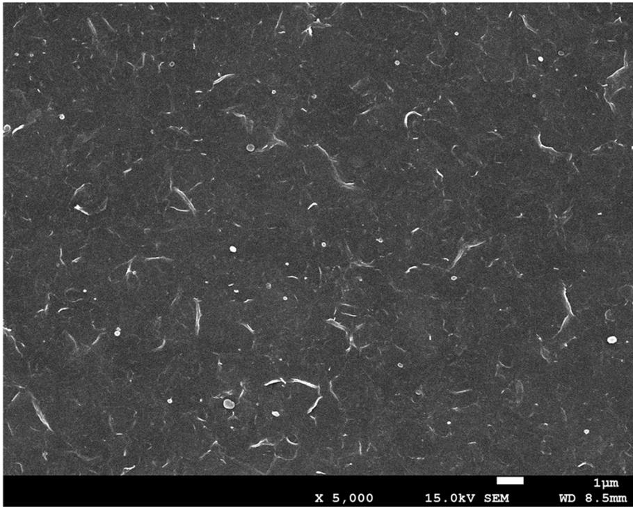
**Fig. S7.** The SEM image of MXene/CNF composite membrane surface.
