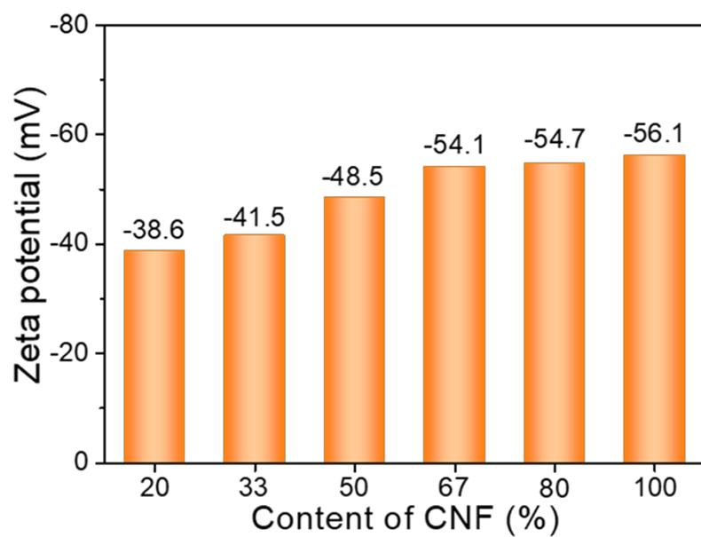
**Fig. S8.** The Zeta potential of the composite membrane with different CNF content.
