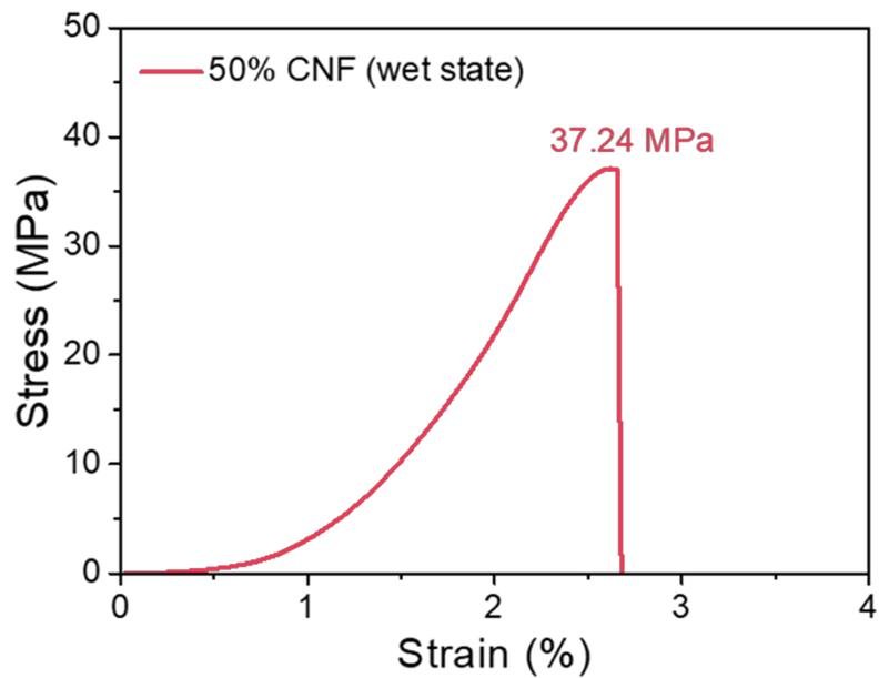
**Fig. S13.** Good mechanical strength of composite membrane (50% CNF) maintained from wet state.
