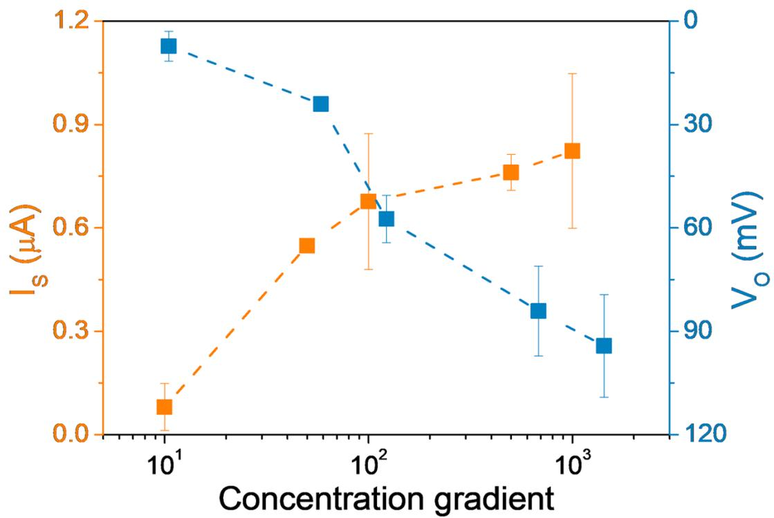
**Fig. S10.** The open circuit voltage ( $V_o$ ) and short circuit current ( $I_s$ ) of membrane (50% CNF) under a series of concentration gradients.
