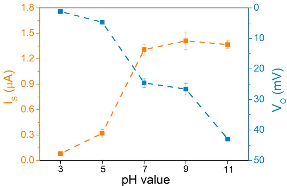
**Fig. S12.** The osmotic energy conversion performance of the composite membrane with CNF content of 50% over the pH range of 3-11. ( $C_H = 0.5$  M NaCl,  $C_L = 0.01$  M NaCl)
