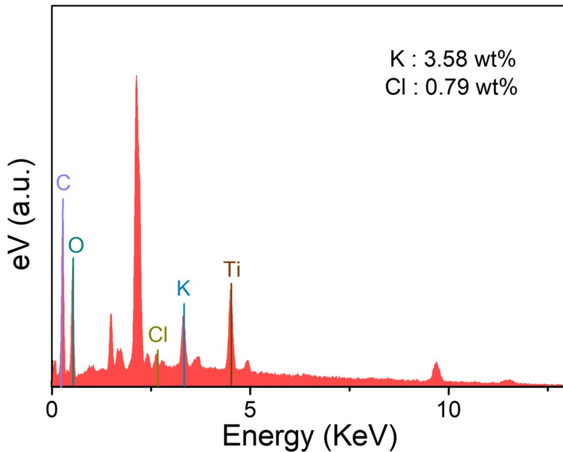
**Fig. S9.** The energy spectrum of the MXene/CNF composite membrane, in which the content of Cl<sup>-</sup> is 0.79 wt% and the content of K<sup>+</sup> is 3.58 wt%, indicates that the composite membrane transports K<sup>+</sup> first and has good cation selectivity.
