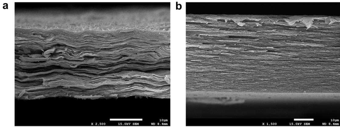
**Fig. S14.** Cross-sectional SEM images of (a) MXene and (b) CNF membrane after fracture.
