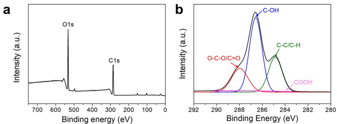
**Fig. S6.** (a) The XPS of CNF membrane. (b) C1s XPS spectra of the CNF, indicating the existence of surface functional carboxyl groups.
