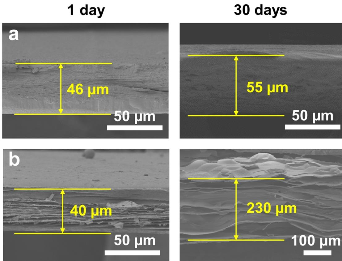
**Fig. S15.** Cross-sectional SEM images of the (a) composite membrane with 50% CNF and (b) pure CNF membrane before and after soaking in 1M KCl solution for 90 days.
