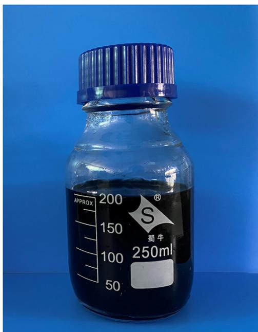
**Fig. S3.** Photograph of a MXene suspension with a concentration of  $0.5 \text{ mg}\cdot\text{mL}^{-1}$ .
