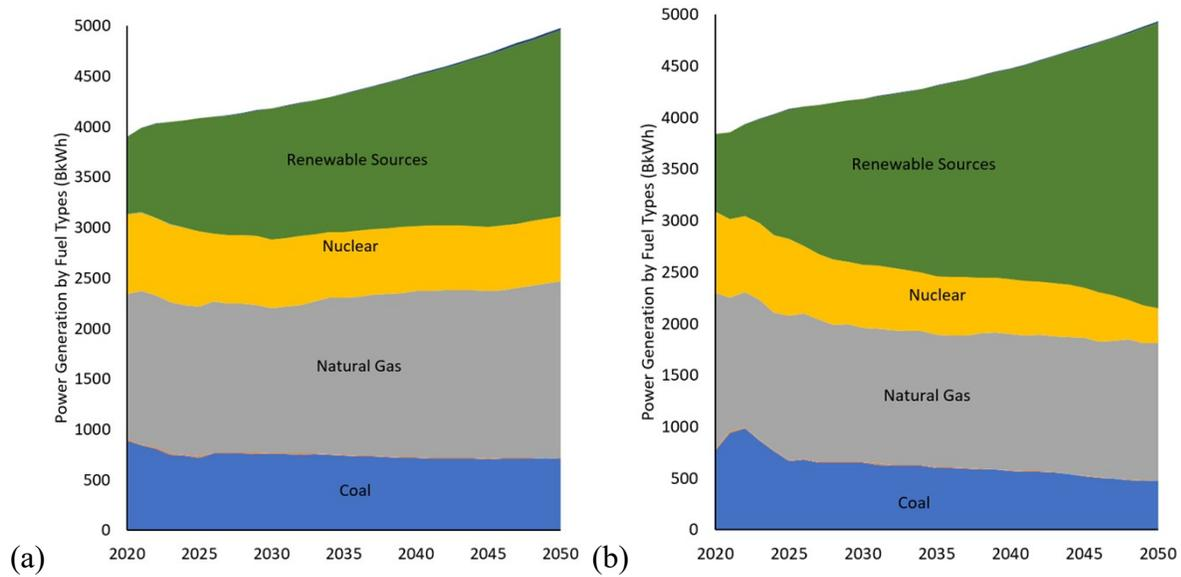
**Fig. S-26. Electricity generation mix (a) reference case; and (b) low renewable cost.**
