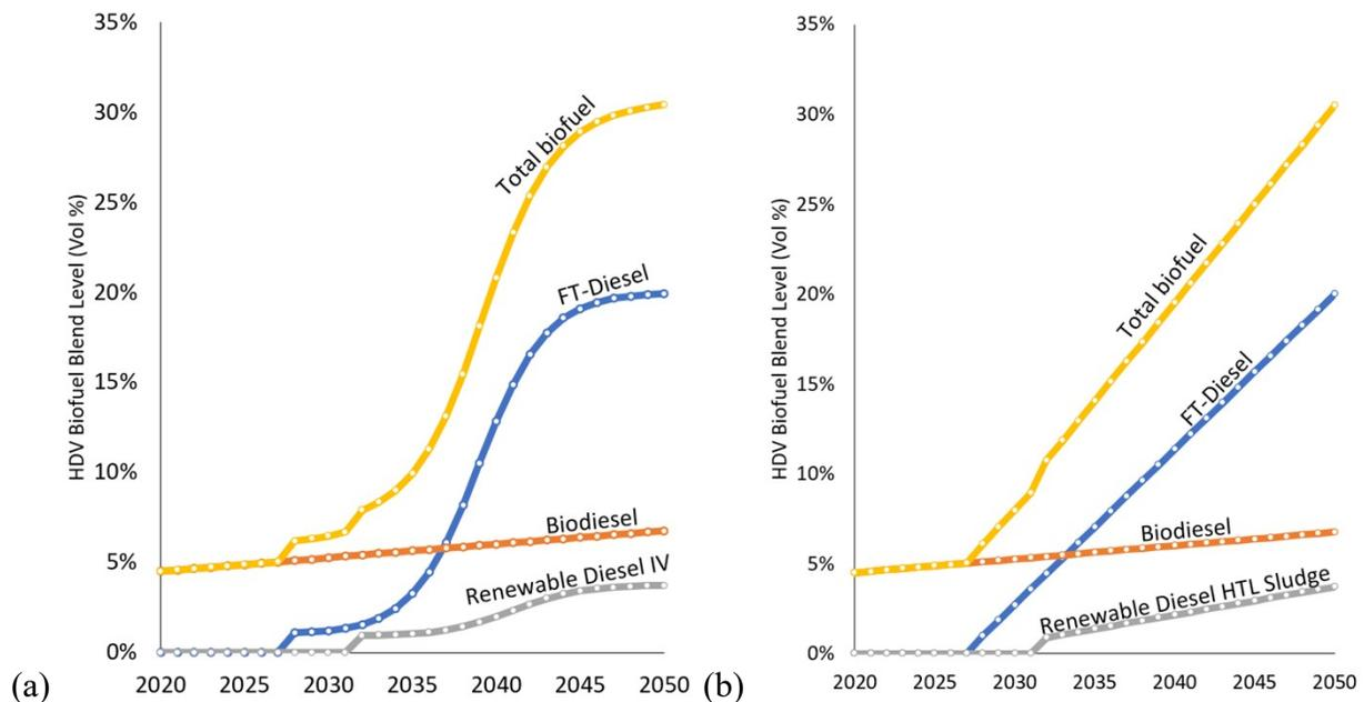
**Fig. S-15. Feasible biofuel level in the HD sector (a) adoption curve path (b) linear path.**
