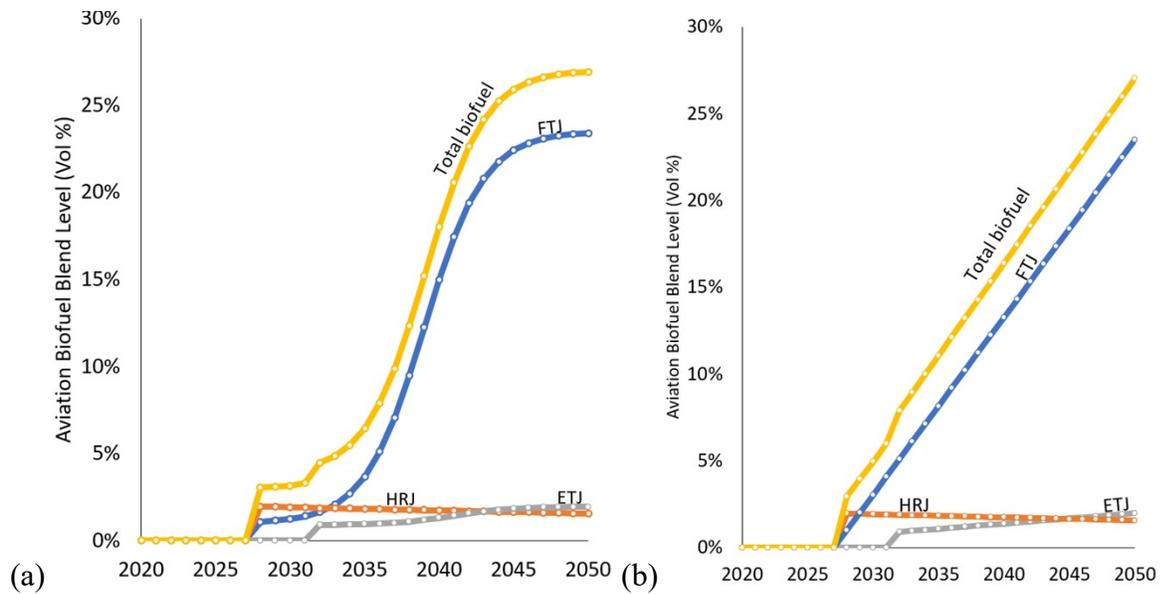
**Fig. S-14. Feasible biofuel level in the aviation sector (a) adoption curve path (b) linear path.**
