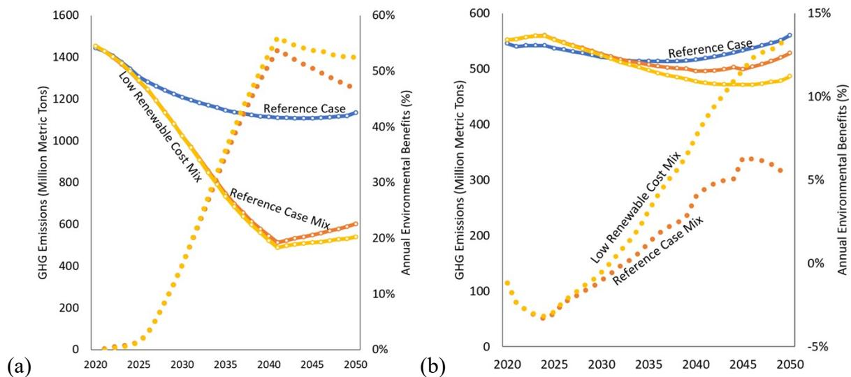
**Fig. S-27. Effect of grid mix on GHG emissions in the high electrification scenarios (a) light-duty; and (b) heavy-duty.**
