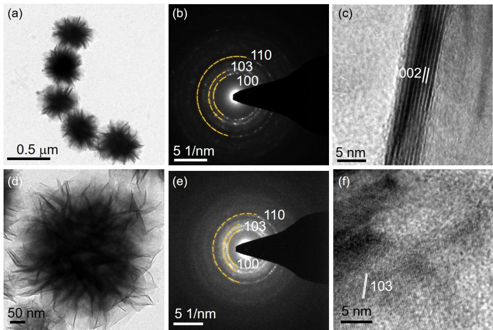
Fig. S4: Microstructural characterization of  $\text{MoSe}_2@\text{WSe}_2$  hierarchical nanostructure- Low-magnification bright-field TEM micrograph showing the sheets protruding from the core, SAED pattern showing the polycrystalline nature of nanoflowers and HRTEM image of  $\text{MoSe}_2@\text{WSe}_2$  of Composition A (a, b, and c) and Composition C (d, e, and f).
