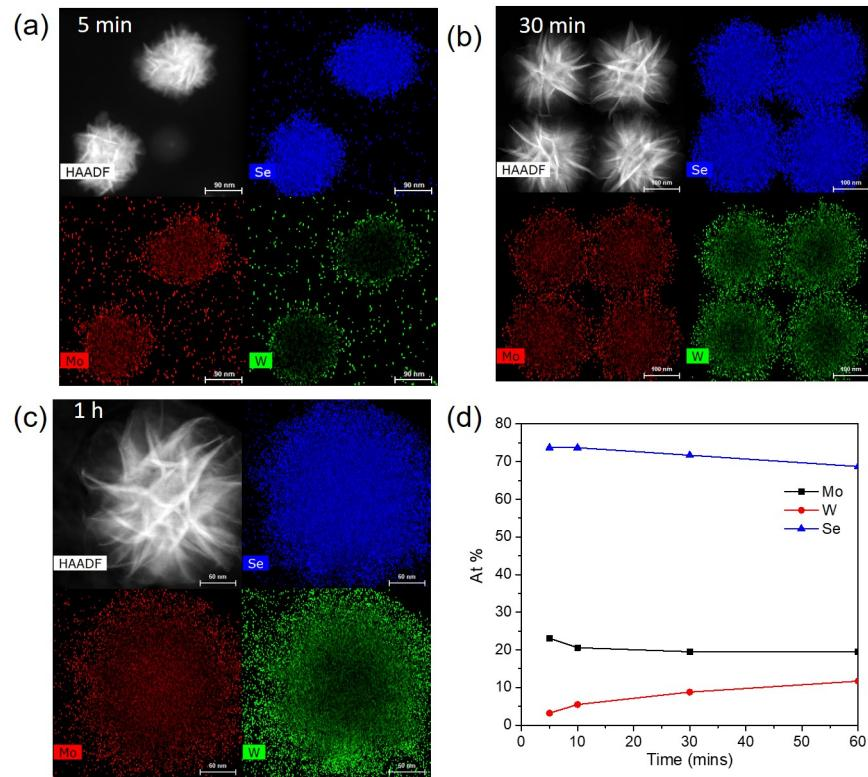
Fig. S7: HAADF-STEM image and EDS map of hierarchical nanostructure formation with 1:1 ratio of Mo:W (Composition B) after 5 mins, 30 mins and 1 h of the reaction, corresponding composition graph showing the overall composition of the product at aforementioned time interval of reaction.
