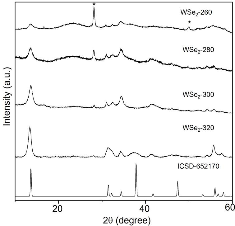
Fig. S2: XRD of  $\text{WSe}_2$  synthesized at different temperature, major impurity peaks of  $\text{WO}_3$  have been marked with \*. A reference XRD pattern of  $\text{WSe}_2$  (ICSD collection code: 652170) is shown in lower panel. At low temperature  $\text{WO}_3$  is the predominant product, with increase in temperature  $\text{WSe}_2$  fraction increases and at 320 °C  $\text{WSe}_2$  forms as predominant product.
