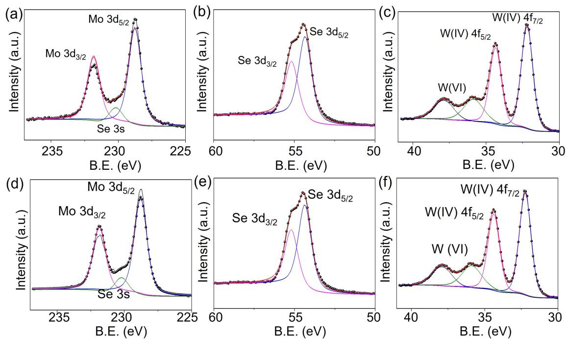
Fig. S14: (a, b, and c) HRXPS spectra of Mo 3d, Se 3d and W 4f post-OER, respectively; (d, e, and f) HRXPS spectra of Mo 3d, Se 3d and W 4f post-HER, respectively.
