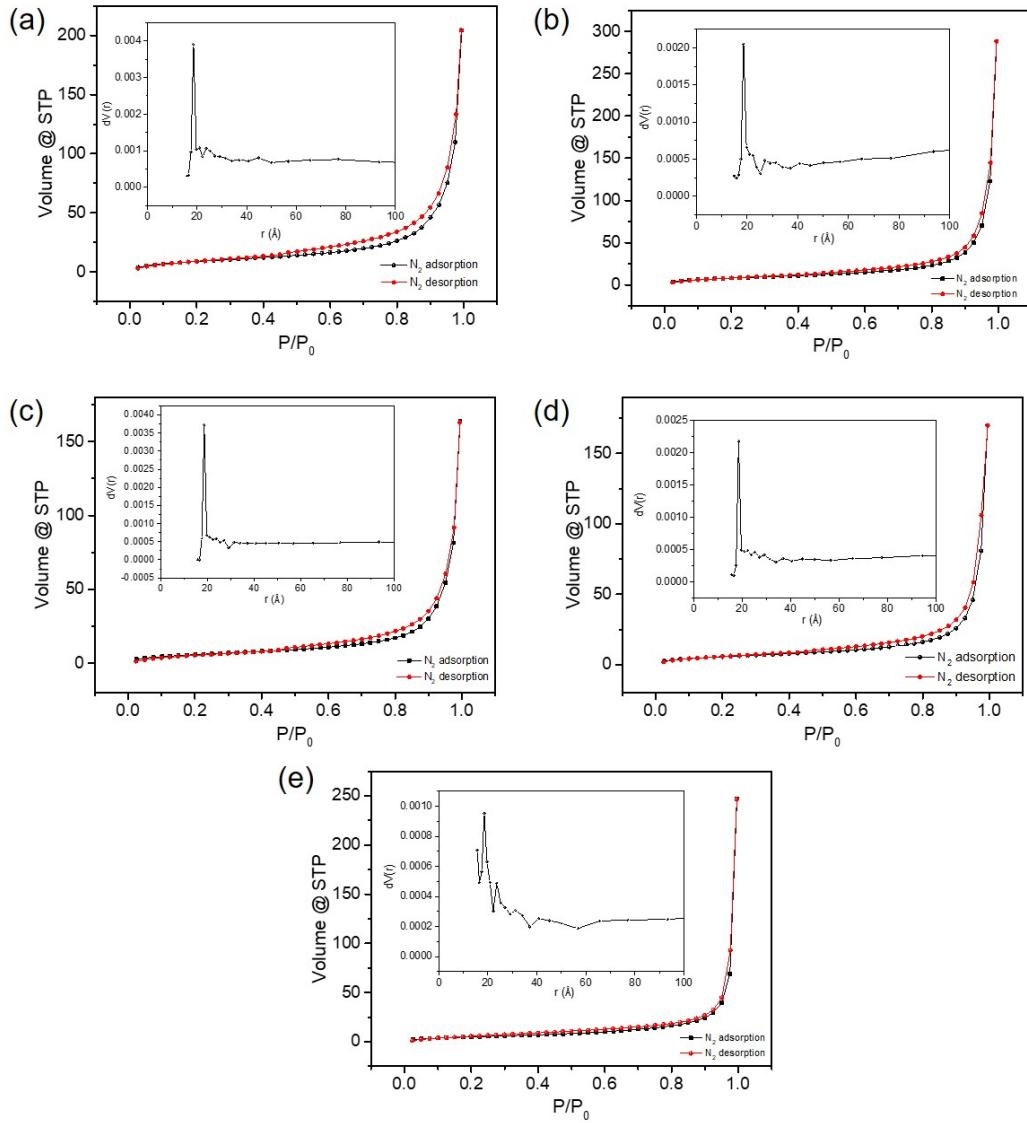
Fig. S10: N<sub>2</sub> adsorption-desorption isotherm (inset: average pore size distribution) of (a) MoSe<sub>2</sub>; (b) Composition A; (c) Composition B; (d) Composition C, and (e) WSe<sub>2</sub>.
