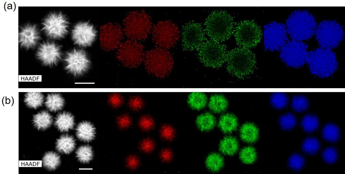
Fig. S5: HAADF-STEM image and elemental maps of Mo, W, and Se in hierarchical nanostructures of (a) Composition A and (b) Composition C. Scale bar shown in the image represent 200 nm.
