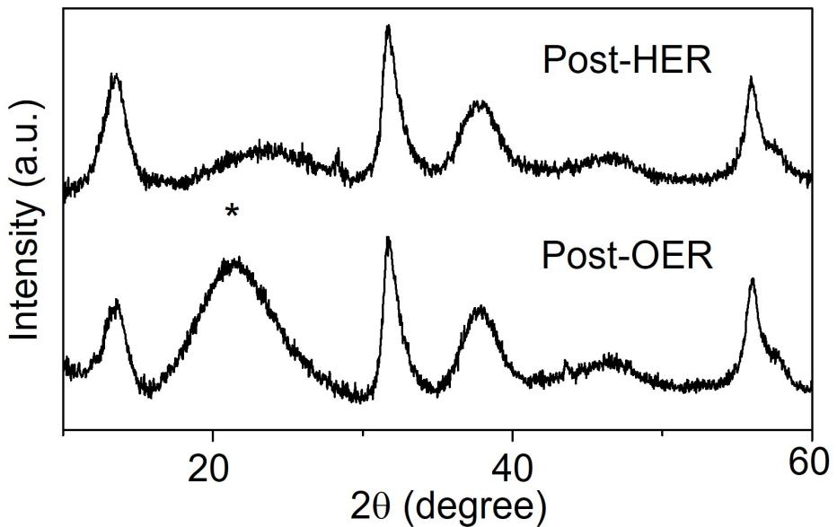
Fig. S13: XRD pattern of the catalysts after 20 h of water-splitting reaction; peak marked with \* corresponds to the carbon.
