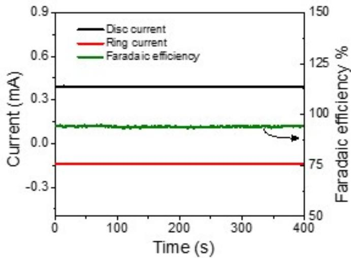
Fig. S18: Faradaic efficiency calculated using the RRDE method.
