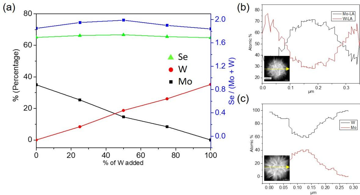
Fig. S6: (a) Overall composition of W, Mo and Se in as-synthesized nanostructures and hierarchical nanostructures. Composition profile of Mo and W along the line drawn across the nanostructures (b) Composition A, and (c) Composition C.
