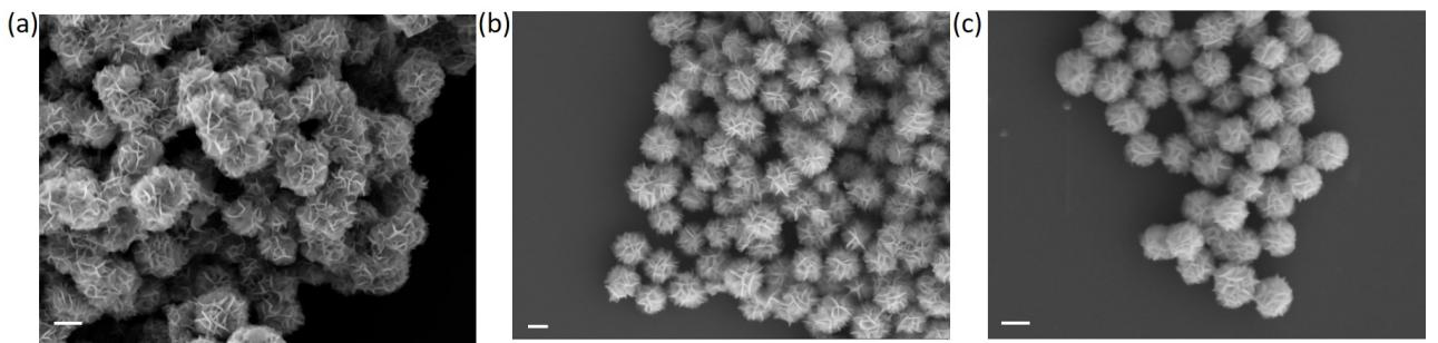
Fig. S3: SEM micrograph of as-synthesized hierarchical nanostructure with different ratio of Mo to W (a) Composition A; (b) Composition B, and (c) Composition C. Scale bar shown in the micrographs represent 200 nm.
