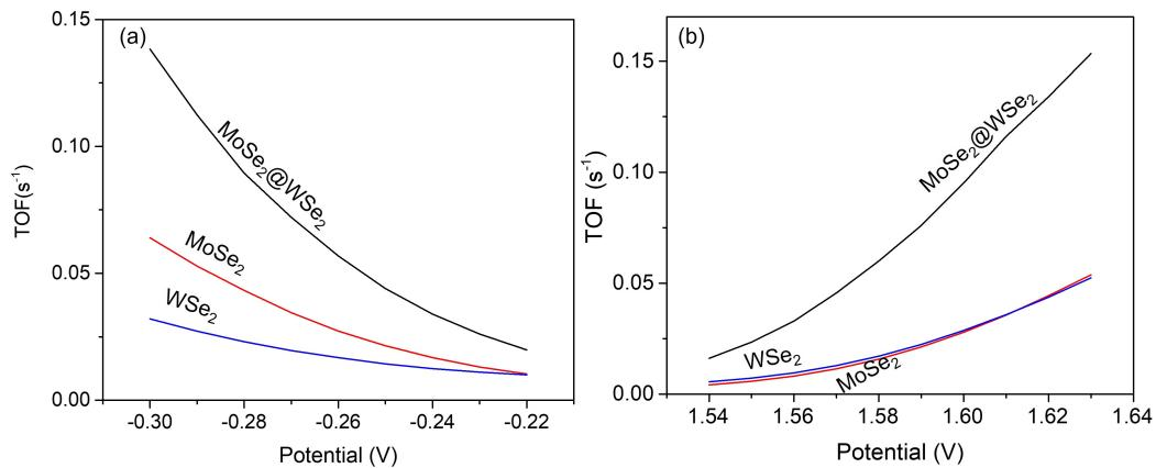
Fig. S19: TOF of as-synthesized catalysts in alkaline medium for (a)HER and (b) OER
