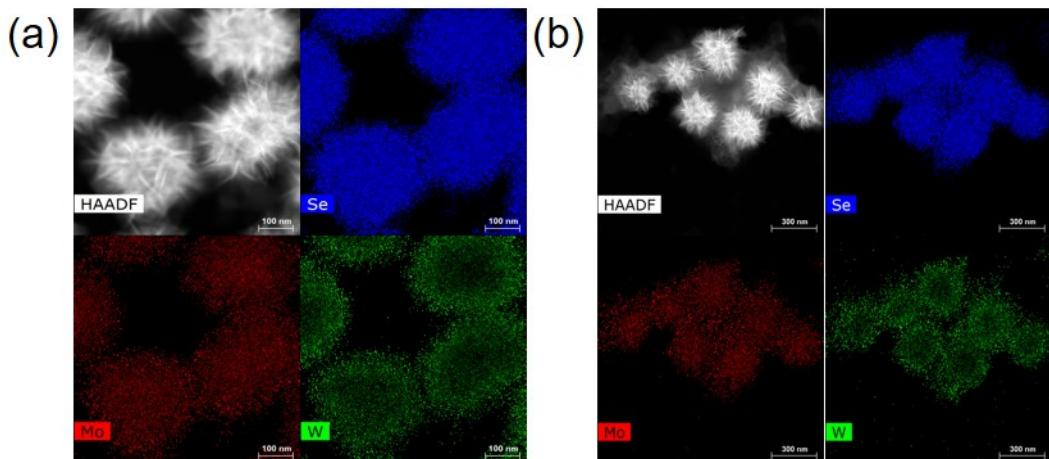
Fig. S16: STEM-EDS map showing the post-electrocatalysis elemental distribution of Mo, W and Se in  $\text{MoSe}_2@\text{WSe}_2$  (Composition B) nanostructure (a) HER and (b) OER.
