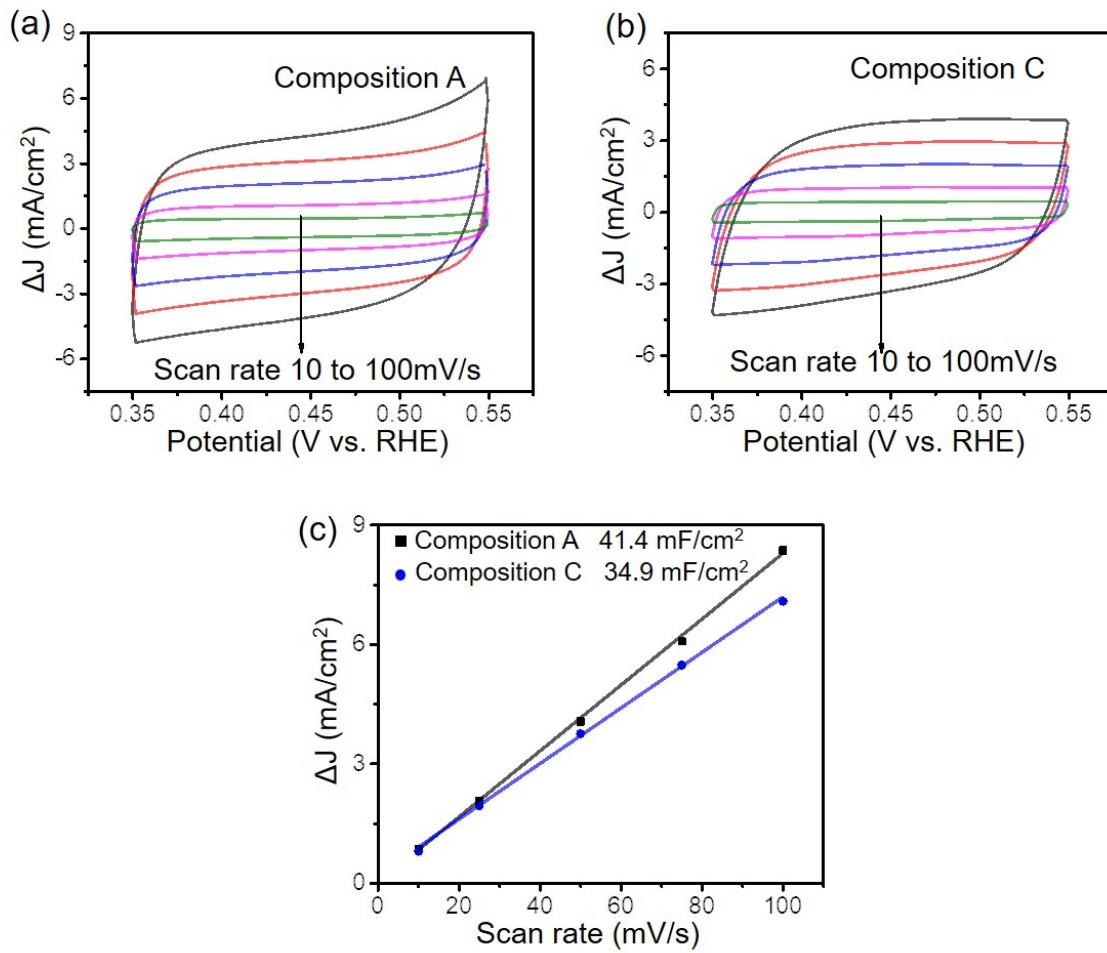
Fig. S11: CV in the faradaic region at different scan rates (10 to 100 mV/s) for (a) Composition A; (b) Composition C, and (c) corresponding  $C_{dl}$  plot
