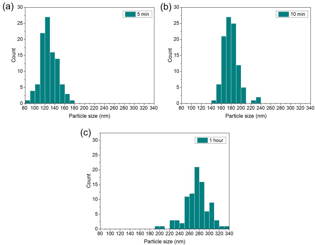
Fig. S8: Particle size distribution of time-dependent reaction product of composition B (a) 5 min; (b) 10 min, and (c) 1 h
