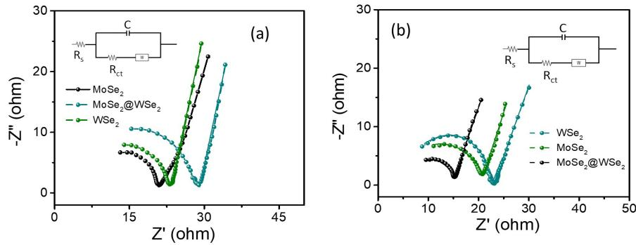
Fig. S17: Nyquist plots for the as-synthesized samples in alkaline media for (a) OER and (b) HER, inset, equivalent circuit model.
