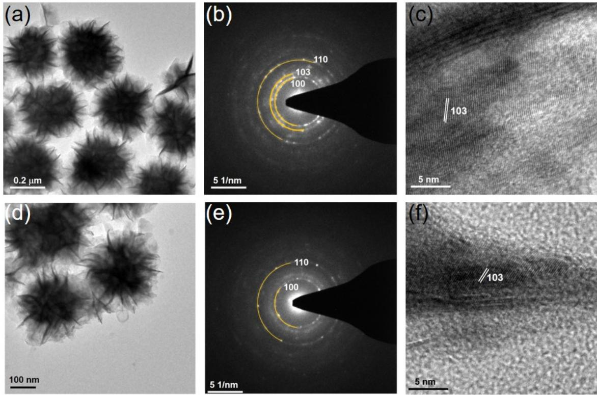
Fig. S15: Microstructural characterization of  $\text{MoSe}_2@\text{WSe}_2$  (Composition B) post-electrocatalysis, (a, b, and c) low-magnification bright-field TEM micrograph, corresponding SAED pattern and HRTEM micrograph of  $\text{MoSe}_2@\text{WSe}_2$  post-HER and (d, e, and f) low-magnification bright-field TEM micrograph, corresponding SAED pattern and HRTEM micrograph of  $\text{MoSe}_2@\text{WSe}_2$  post-OER respectively.
