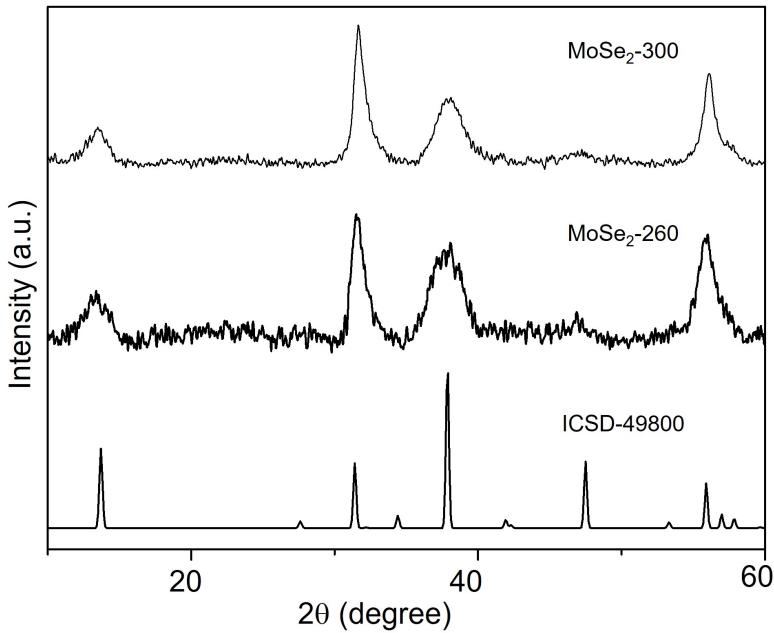
Fig. S1: XRD of  $\text{MoSe}_2$  synthesized at different temperature. A reference XRD pattern of  $\text{MoSe}_2$  (ICSD collection code: 49860) is shown in lower panel. Even at low-temperature such as 260 °C,  $\text{MoSe}_2$  forms as predominant product.
