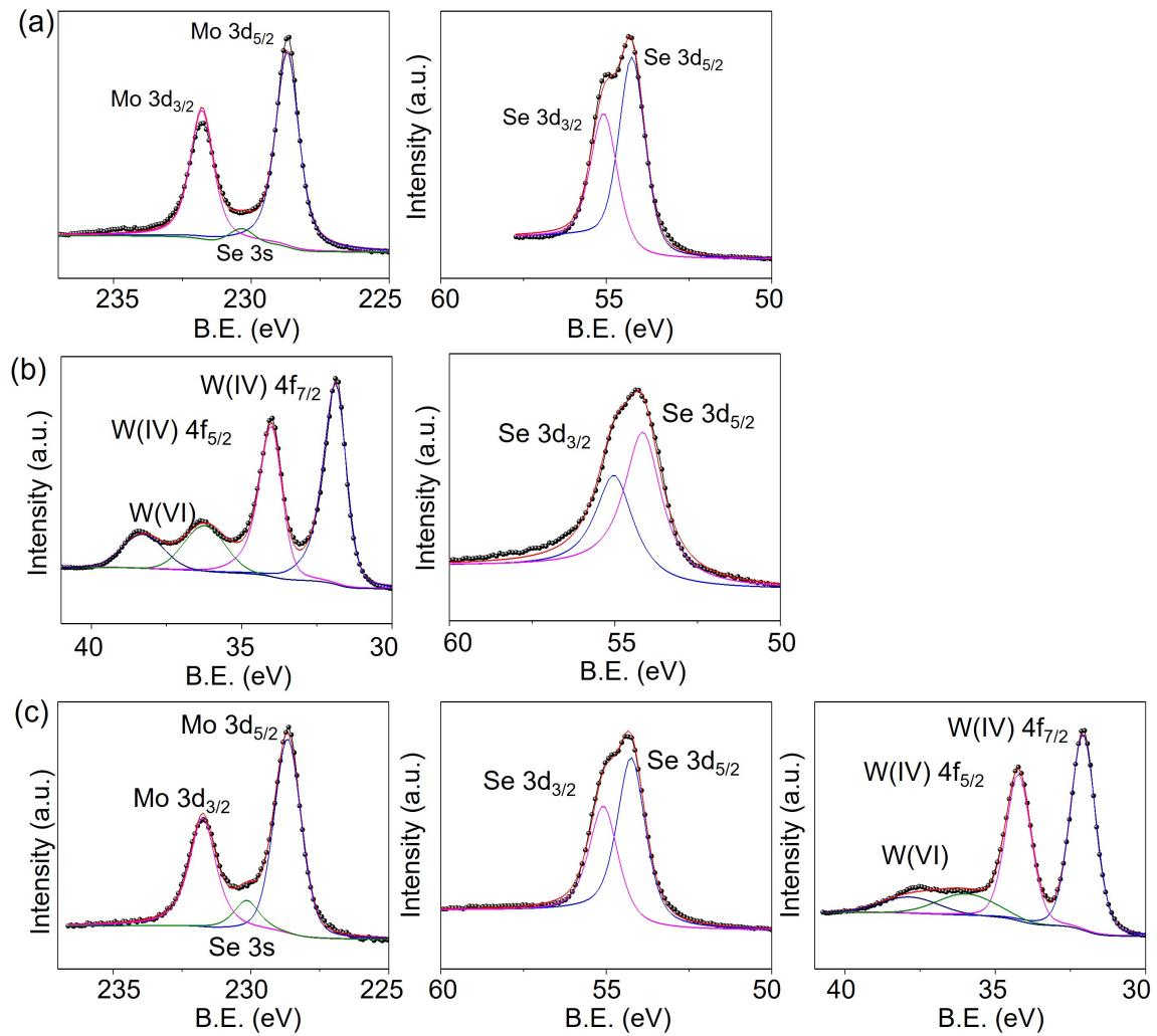
Fig. S9: HRXPS spectra of (a) MoSe<sub>2</sub>; (b) WSe<sub>2</sub>, and (c) MoSe<sub>2</sub>@WSe<sub>2</sub> (Composition B)
