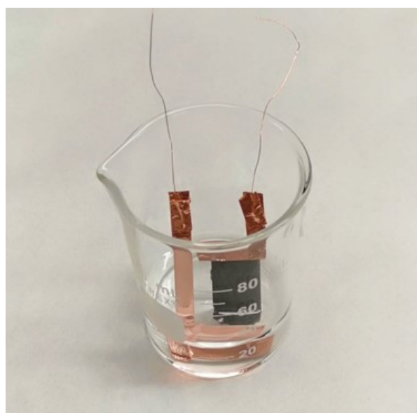
Figure S6. Digital image of FMWCNTs device kept in a 100 mL beaker covering 0.5 cm of bottom of the FMWCNTs device.
