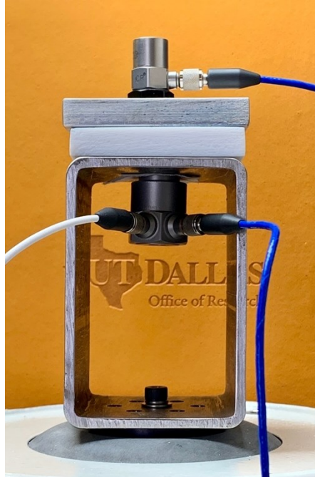
Figure S1: Test sample configuration for transmissibility measurements. The sample is sandwiched between two steel parts and the accelerations are measured using an impedance head at the bottom and an accelerometer at the top of the sample.
