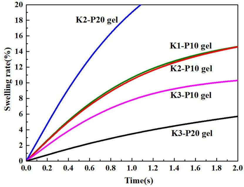
**Fig. S2** The swelling rate in the initial stage for different hydrogel samples.
