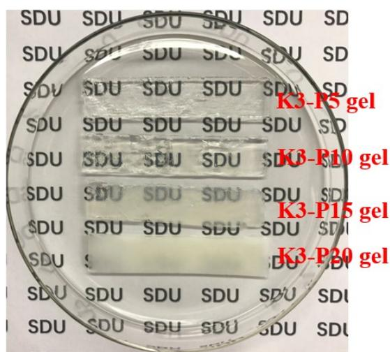
**Fig. S1** The appearance of obtained  $\kappa$ -carrageenan/PIL DN hydrogels.
