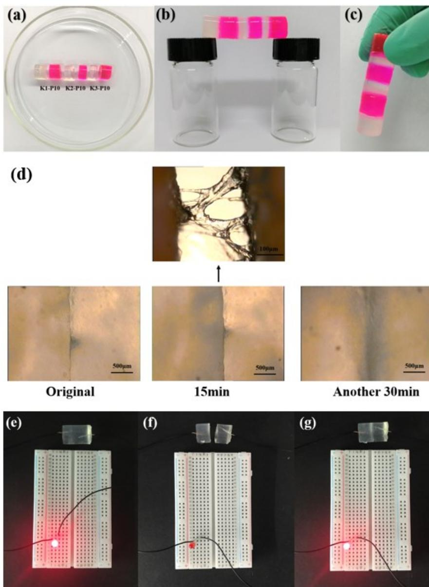
**Fig. S7** (a-c) Self-healing process of K1-P10, K2-P10, and K3-P10 hydrogels. (d) Self-healing process of 1-15 hydrogel under optical microscope. (e-g) Circuit comprises an LED indicator connected by (e)undamaged, (f)cut, and (g)self-healed K3-P10 hydrogel column.
