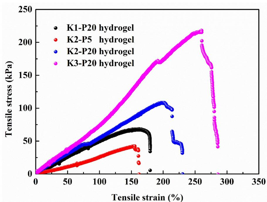
**Fig. S4** Strain stress-strain curves of different hydrogels.
