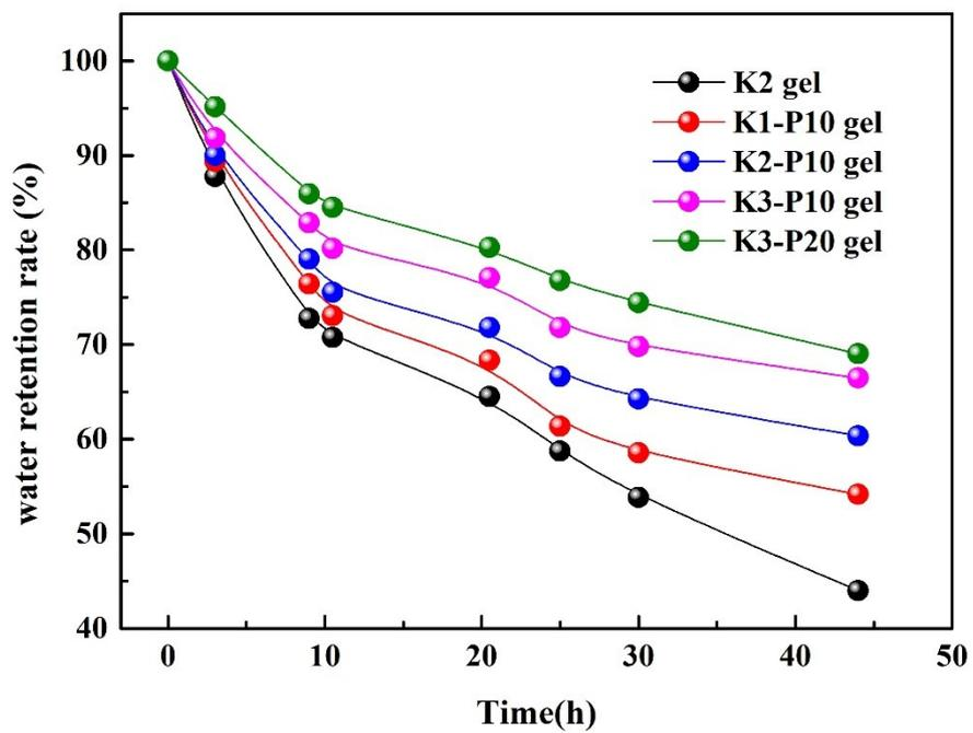
Fig. S6 Plot of water retention rate (%) versus time for different hydrogel samples.
