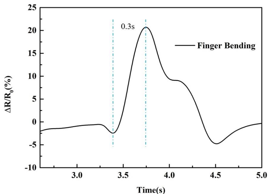
**Fig. S8** The response time of K3-P20 hydrogel to monitor the joint motion of fingers.
