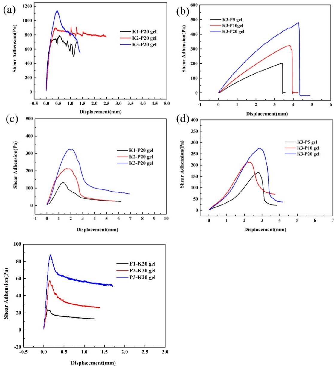
**Fig. S10** Adhesion strength of different hydrogels on various substrates (a)glass, (b) silicone, (c) plastic, (d) hogskin and (e) stainless steel.
