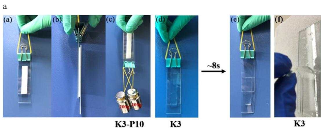
**Fig. S5** (a-c) Schematic of static shear test of the K3-P10 DN hydrogel adhesion on glass substrates and 400 g hanging weight. (d-e) Illustration of the K3 hydrogel adhesion on glass, and the glass slides will slide off without the weight hanging. (f) The K3 hydrogel is peeled from the glass plate with water left.
