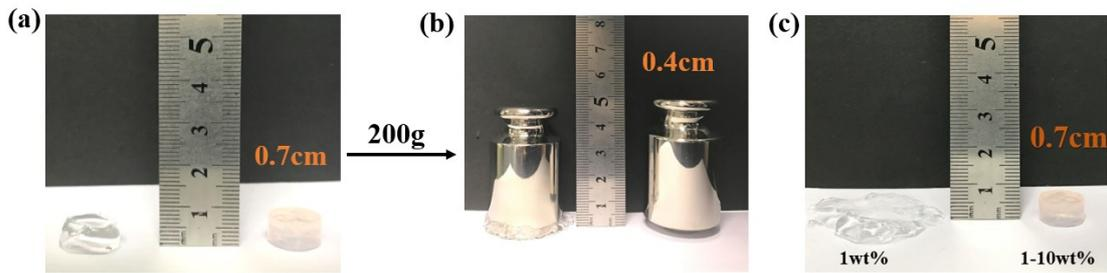
**Fig. S3** Load-bearing capacity tests of K1 and K1-P10 hydrogels (the weight is 200g).
