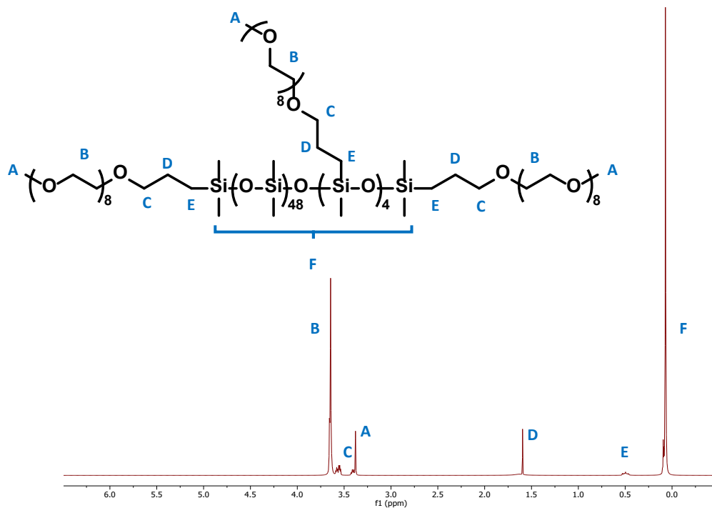
Figure S10. 1 H NMR of "Triblock [SGP]", (CDCl 3 ; δ, ppm): 0.03-0.26 (m, 312H, SiCH 3 ), 0.41-0.54 (m, 12H, SiCH 2 CH 2 CH 2 ), 1.51-1.66 (m, 12H, SiCH 2 CH 2 CH 2 ), 3.37 (s, 18H, OCH 3 ), 3.40 (t, J = 7.12 Hz, 12H, SiCH 2 CH 2 CH 2 ), 3.50-3.70 (m, 192H, CH 2 CH 2 O).
