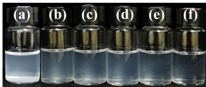
Fig. S1 Photographs of SDP (0.15 wt% or ~5 mM)/H 2 O mixtures (a) in the absence of GuSalts and (b–f) in the presence of 0.30 wt% (b) GuCl, (c) GuSO 4 , (d) GuSO 3 , (e) GuPO 4 , and (f) GuCO 3 . All samples were placed at 25.0 °C for at least 48 h before the observation.
