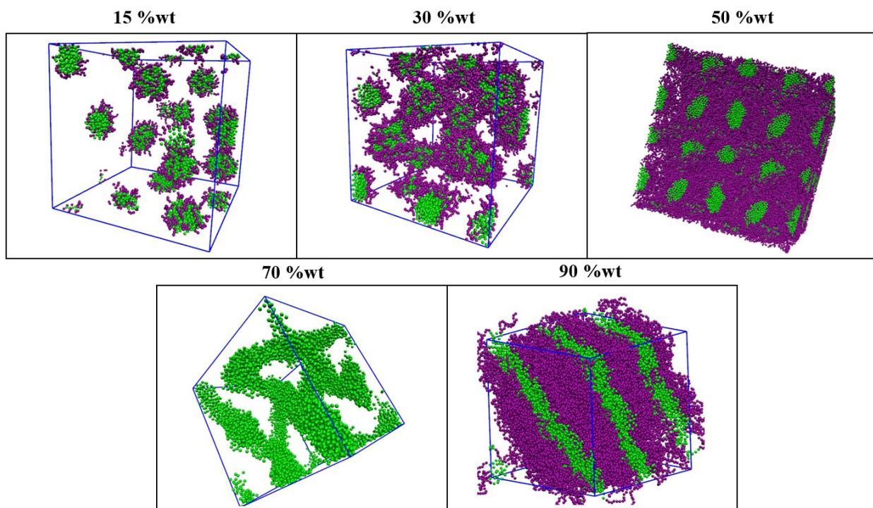
**Figure S9.** Final snapshots of the CG-MD simulations for the  $C_{16}E_{12}$ /water system at different concentrations. Colors as in Figure S2
