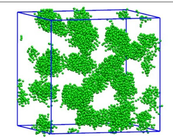
**Figure S7.** Final snapshots of the CG-MD simulations carried out for the system  $C_{12}E_{23}$ /water at different concentrations. For an easier visualization only the alkyl chains are represented.
