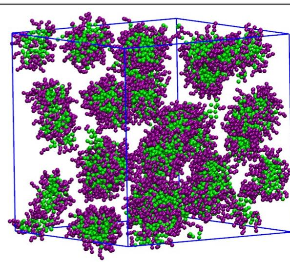
**Figure S3.** Final snapshots of the CG-MD simulations carried out for the system C<sub>8</sub>E<sub>6</sub>/water at 15 and 30%wt. Green is used to represent the alkyl tail beads, while purple represents the beads from the hydrophilic moiety. Water molecules are omitted to allow for an easier visualization.
