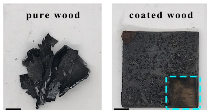
Fig. S6. Optical image of pure wood (left) and coated wood (right) after being subjected to butane flame for 30 s (scale bar: 1 cm). The highlighted area is the inner intact wood after eliminating the char.
