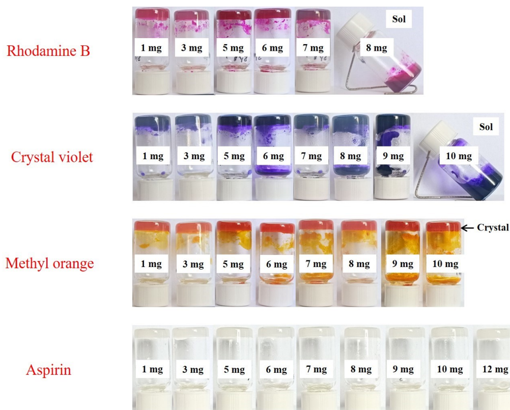
Figure S13. Photograph depicting the entrapment of rhodamine B, crystal violet, methyl orange and aspirin, respectively, in the BHTP gel (10 mg/mL).
