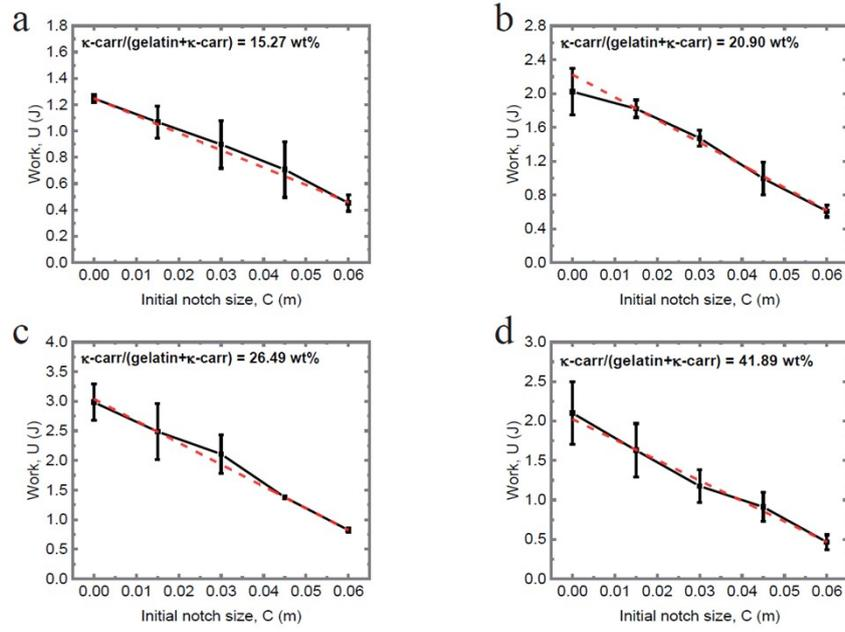
**Fig. S8** The work,  $U$ , done in deforming gelatin/ $\kappa$ -carrageenan/PAAm gel samples with various initial crack sizes with various fractions of  $\kappa$ -carrageenan to the total gum (a) 15.27 wt%, (b) 20.90 wt%, (c) 26.49 wt%, (d) 41.89 wt%.
