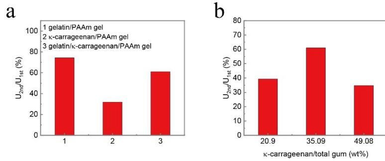
**Fig. S3** (a) Recovery percentage of gelatin/PAAm gel,  $\kappa$ -carrageenan/PAAm gel and gelatin/ $\kappa$ -carrageenan/PAAm gel. (b) Recovery percentage of gelatin/ $\kappa$ -carrageenan/PAAm gel of various fractions of  $\kappa$ -carrageenan to the total gum (20.9, 35.09, 49.08 wt%).
