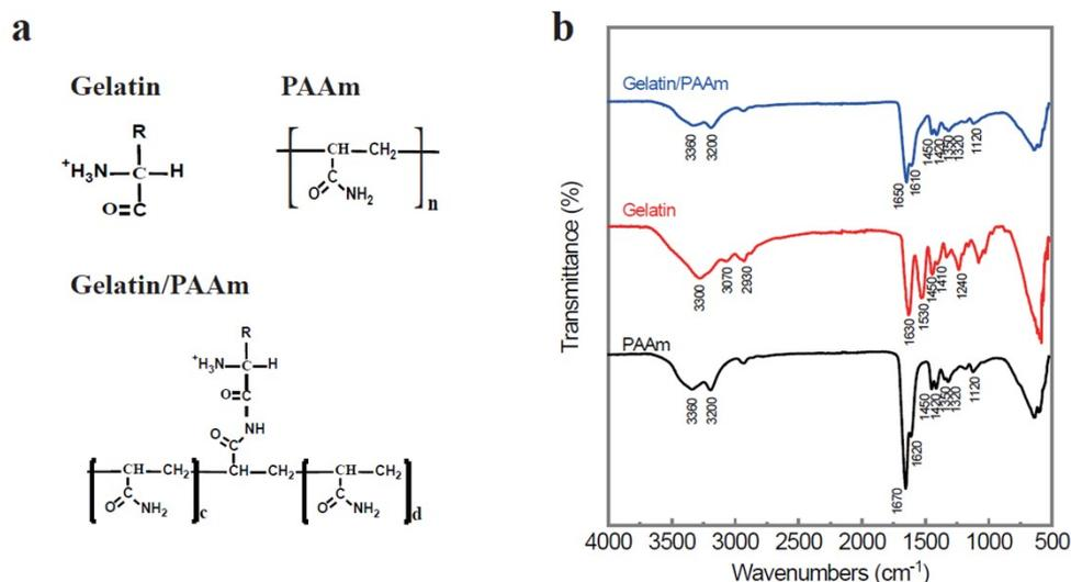
**Fig. S1** (a) Chemical structure of gelatin, PAAM and gelatin/PAAM. (b) ATR-IR spectra of PAAM, gelatin/PAAM, gelatin/ $\kappa$ -carrageenan/PAAM gels.
