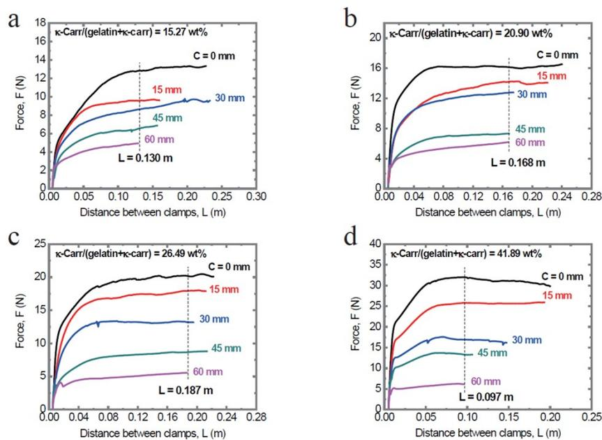
**Fig. S7** Force-extension curves for various initial crack sizes. An edge crack was introduced to gelatin/PAAM gel samples with various fractions of  $\kappa$ -carrageenan to the total gum (a) 15.27 wt%, (b) 20.90 wt%, (c) 26.49 wt%, (d) 41.89 wt%.
