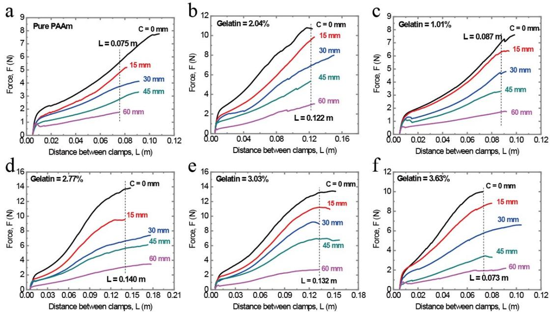
**Fig. S5** Force-extension curves for various initial crack sizes. An edge crack was introduced to gelatin-PAAm gel samples with various concentration of gelatin (w/v, v is the volume of water). (a) 0%, (b) 1.01%, (c) 2.04%, (d) 2.77%, (e) 3.03%, (f) 3.63%.
