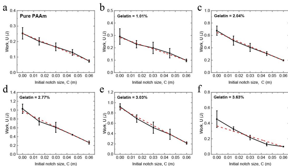
**Fig S6** The work,  $U$ , done in deforming gelatin/PAAM gel samples with various initial crack sizes with various concentration of gelatin (w/v, v is the volume of water). (a) 0%, (b) 1.01%, (c) 2.04%, (d) 2.77%, (e) 3.03%, (f) 3.63%.
