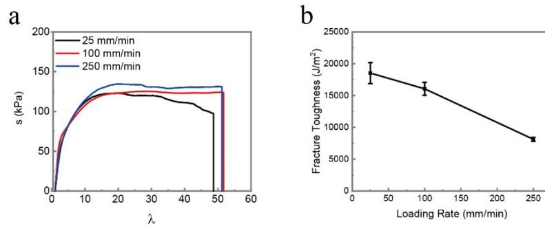
**Fig. S4** (a) Stress-stretch curves of gelatin/ $\kappa$ -carrageenan/PAAm gels at various loading rates. (b) Fracture toughness as a function of the loading rate.
