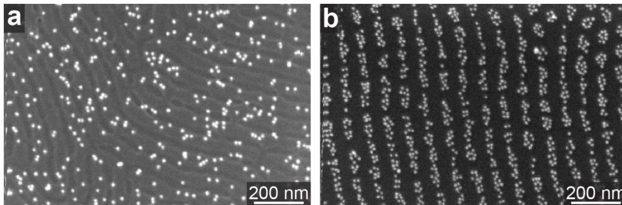
**Figure S2.** SEM images of: (a) a sample that underwent protonation with 1% HCl solution for 24 h, followed by NP deposition; (b) a sample that was treated with DIB as the first step, then dipped into 1% HCl solution for 24 h, followed by NP deposition.
