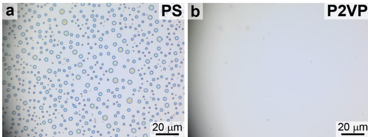
Figure S4. Optical microscopy images of 23-24 nm-thick films cast on hydrophilic SiOx substrates and annealed in chloroform vapour for 20 min, showing significant difference in wetting properties: (a) PS ( $M_n$ , 50 kDa) and (b) P2VP films ( $M_n$ , 50 kDa).
