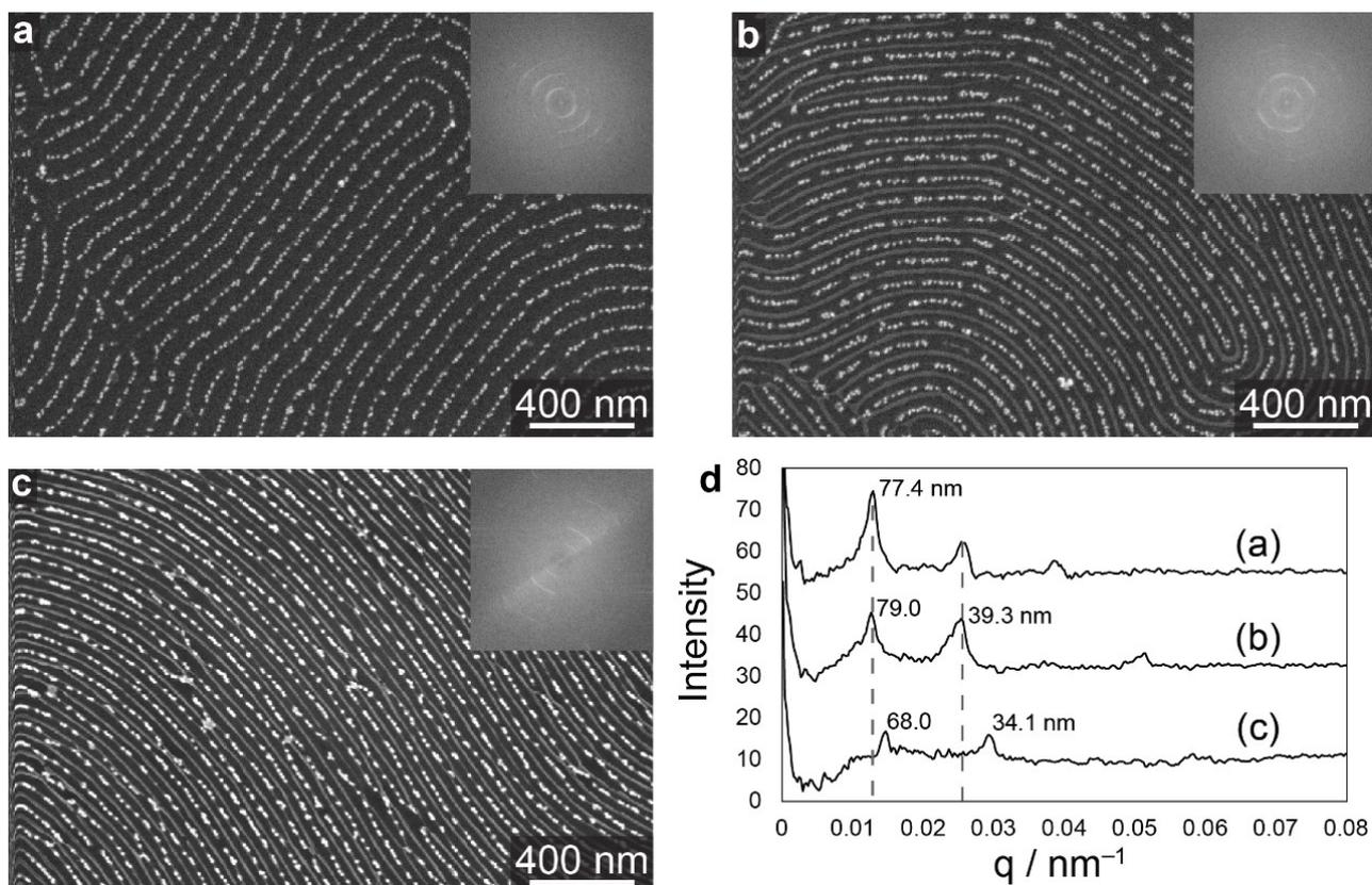
**Figure 56.** (a-c) SEM images of: (a) a periodic Au NP-decorated Pd NW array, and arrays of alternating bare and NP-decorated wires obtained in (b) 37 nm-thick film and (c) 60 nm-thick film. Insets represent FT analyses. (d) Radially integrated plots of the FT images after background subtraction. The lamellar periodicities are denoted next to the principal peaks. Dashed lines mark the principal periodicities in the thin films.
