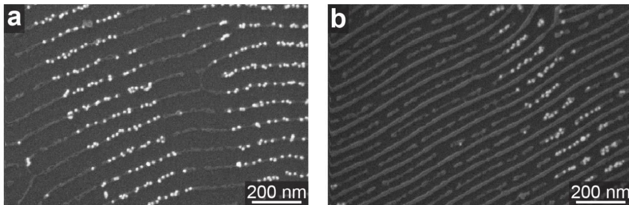
**Figure 57.** SEM images of a NW array with co-existing patterns originating from a 38 nm-thick film where some NPs were removed by a gentle scratch and exposed the underlying Pd NWs: (a) NP-decorated NW array originating from a region featuring a locally thin film; (b) alternating striped structure resulting from an area featuring a locally thick film.
