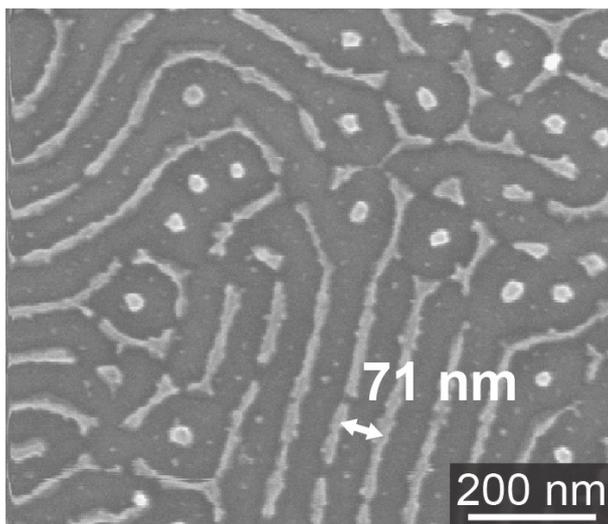
**Figure S8.** Top view SEM images of a Pd NW array resulting from impregnation under non-acidic conditions. The calculated periodicity of the array is denoted on the image.
