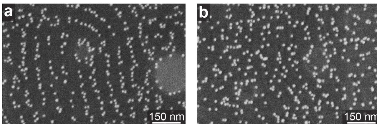
**Figure S3.** SEM images of Au NPs deposited on a PS-*b*-P2VP film: (a) with DIB crosslinking before NP deposition; (b) without DIB crosslinking.
