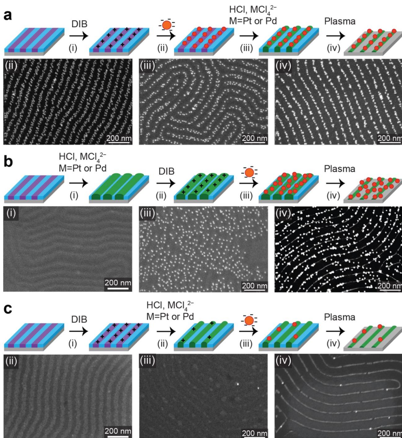
**Figure S1.** The influence of the sequence of the assembly/fabrication steps on the final result. (a) The optimized process; (b) a modified process, in which metal impregnation is the first step; (c) a modified process, in which metal impregnation is the second step.
