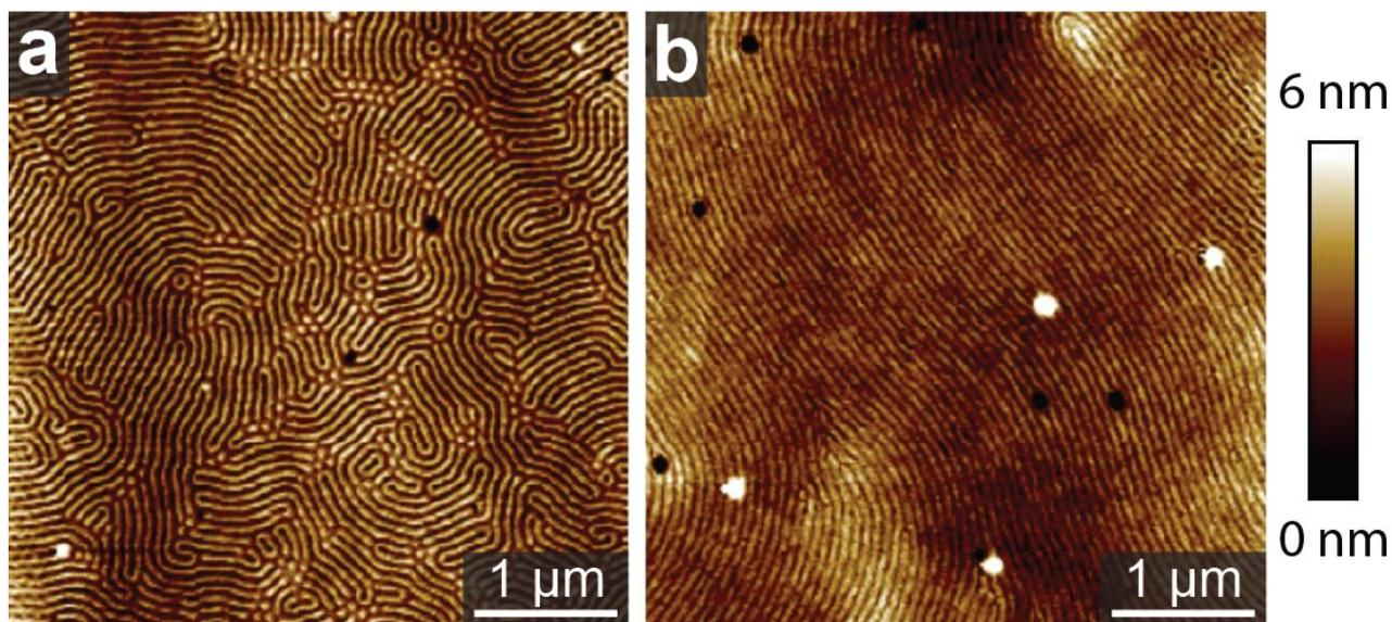
Figure S5. AFM images of cylindrical PS-*b*-P2VP films featuring: (a) a monolayer of P2VP cylinders (local film thickness 30 nm); (b) a bilayer of P2VP cylinders (local thickness 58 nm).
