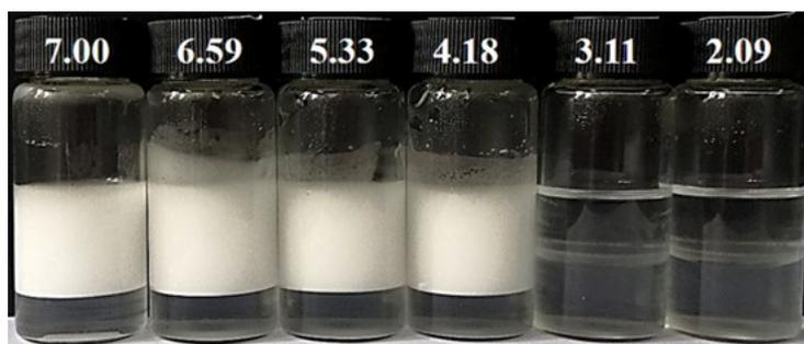
**Figure S17.** Digital photos of *n*-decane-in-water (7 mL/7 mL) oil-in-dispersion emulsions stabilized by 0.01 wt.% alumina nanoparticles and 0.06 mM N<sup>+</sup>-8P8-N at different pH, taken 24 h after preparation at 25 °C.
