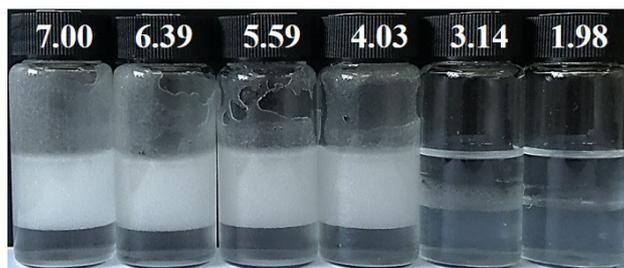
**Figure S13.** Digital photos of *n*-decane-in-water (7 mL/7 mL) Pickering emulsions stabilized by 0.1 wt.% silica nanoparticles and 0.1 mM N<sup>+</sup>-8P8-N at different pH at 25 °C, taken 24 h after preparation.
