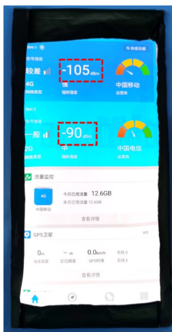
Fig. S17 The photographs of the signal intensities of the mobile phone coated with the commercial graphene film.
