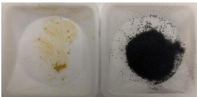
**Figure S2.** Visual appearance of (left) Ni-MOF-74 as prepared and (right) Ni-MOF-74 after testing at 300 °C. The catalyst presented after testing is still mixed with clear glass beads.
