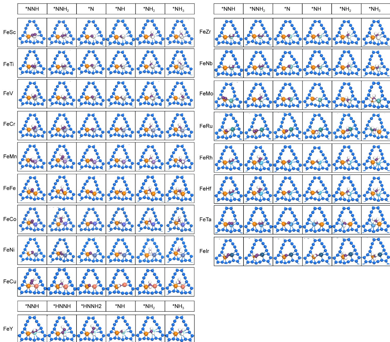
Fig. S9 The optimized adsorption configurations of each intermediate in eNRR on FeM-GDYs (M = Sc, Ti, V, Cr, Mn, Fe, Co, Ni, Cu, Y, Zr, Nb, Mo, Ru, Rh, Hf, Ta, and Ir).
