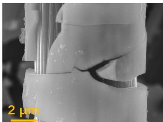
**Fig. S4.** SEM image for CoMoOF/GF after sonication in 1.0 M KOH for 2 h.
