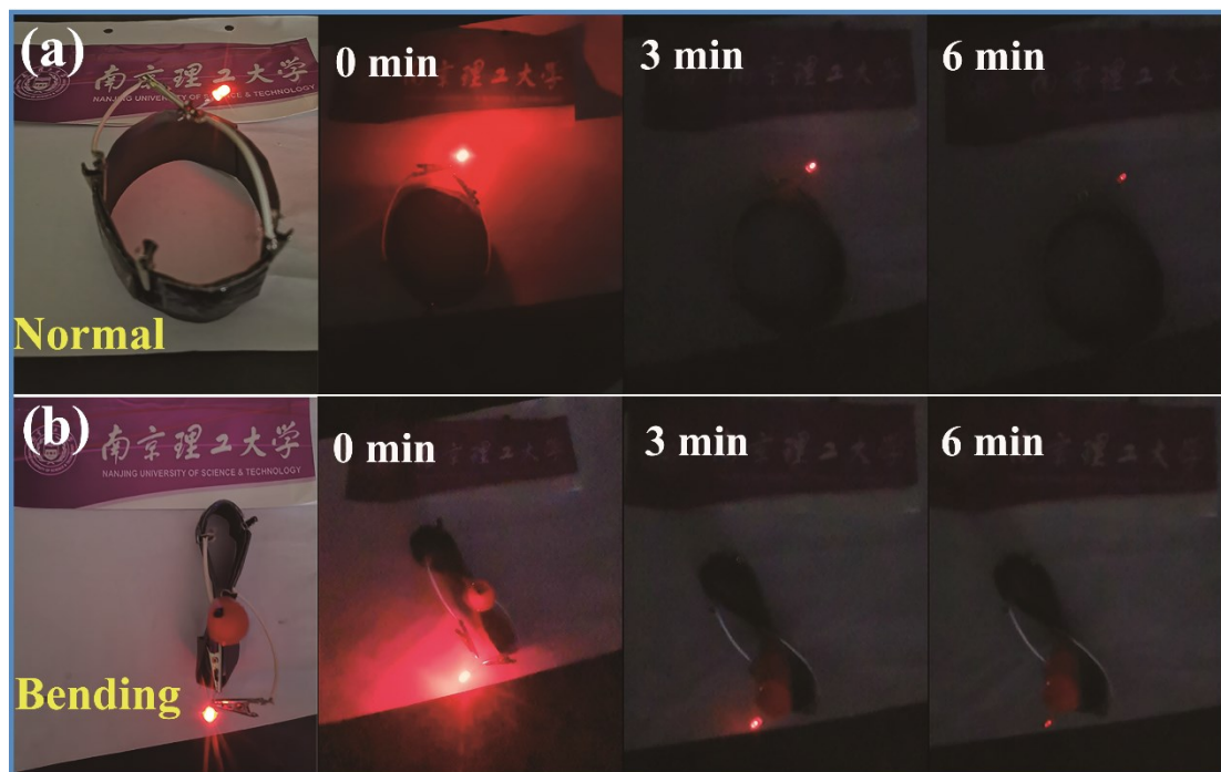
Fig. S12. Two assembled FASSAS devices connected in series light up the red LED indicator for 6 minutes under (a) normal and (b) bending conditions.
