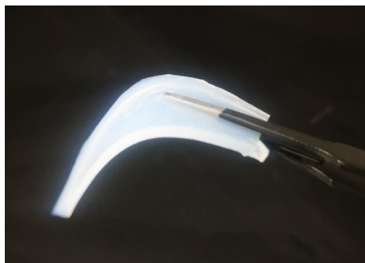
Fig. S18 A digital image of the as-prepared flexible PVA gel film.
