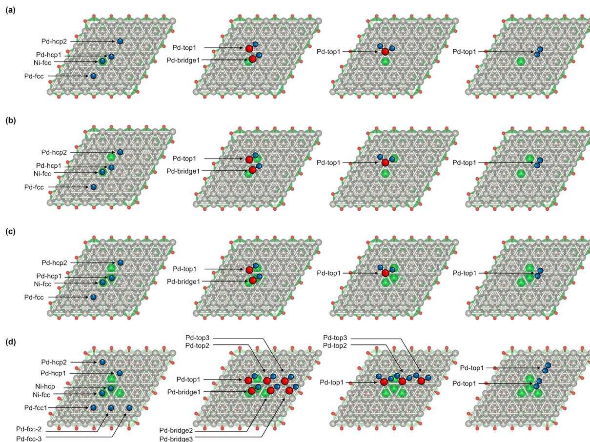
**Figure S3.** Top view atomic adsorption structures of H\*, OH, H<sub>2</sub>O and H<sub>2</sub> (panels from left to right) at different adsorption sites on the (a) NiO<sub>2</sub>-Ni<sub>1</sub>-Pd, (b) NiO<sub>2</sub>-Ni<sub>2</sub>-Pd, (c) NiO<sub>2</sub>-Ni<sub>3</sub>-Pd and (d) NiO<sub>2</sub>-Ni<sub>4</sub>-Pd surface models. For clarity, the grey, green, red and blue spheres stand for Pd, Ni, O and H atoms, respectively.
