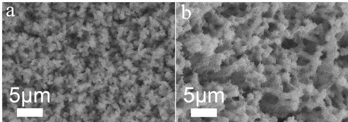
Fig. S18. The SEM images of (a)  $\text{Co}_x\text{O}_y/\text{Cu}_x\text{O}/\text{Cu}$  and (b)  $\text{Ni}_x\text{O}_y/\text{Cu}_x\text{O}/\text{Cu}$ .
