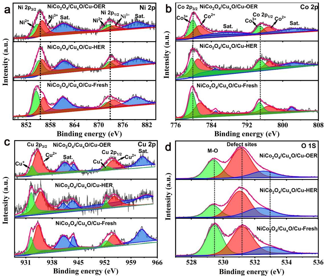
Fig. S25 High-resolution XPS spectra of (a) Ni 2p, (b) Co 2p, (c) Cu 2p, and (d) O 1s of  $\text{NiCo}_2\text{O}_4/\text{Cu}_x\text{O}/\text{Cu}$  after HER for 150 h and OER for 125 h in KOH (1 M) solution.
