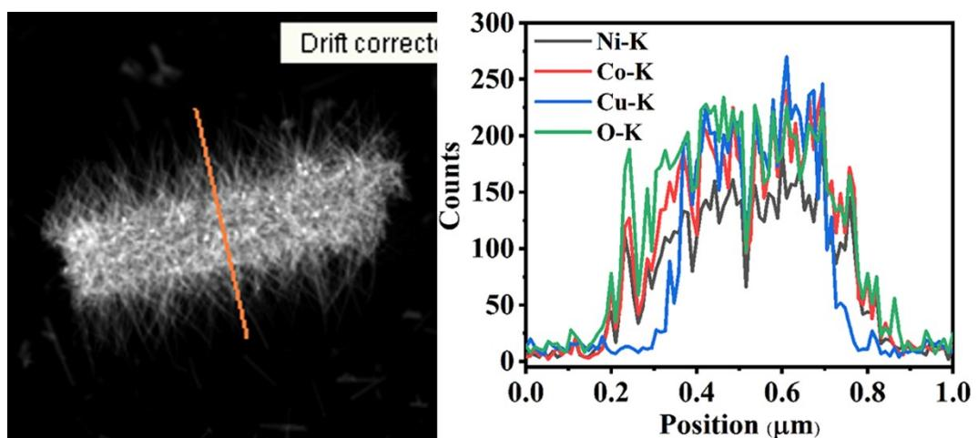
Fig. S9 HAADF images and the corresponding line-scan elemental distribution curves of  $\text{NiCo}_2\text{O}_4/\text{Cu}_x\text{O}$ .
