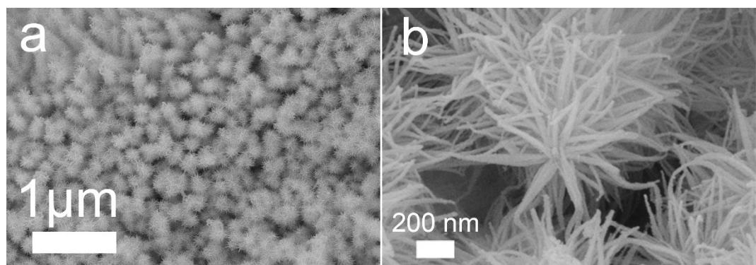
Fig. S21 (a) Low and (b) high magnification SEM images of  $\text{NiCo}_2\text{O}_4/\text{Cu}_x\text{O}/\text{Cu}$  after overall water splitting reaction in KOH (1 M) solution for 30 h.
