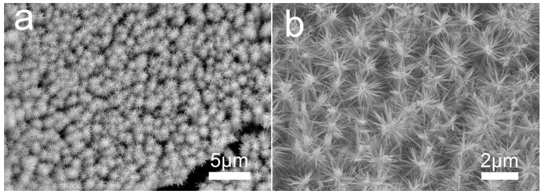
Fig. S5 (a) Low and (b) high magnification SEM images of NiCo-precursor/Cu(OH)<sub>2</sub>/Cu.
