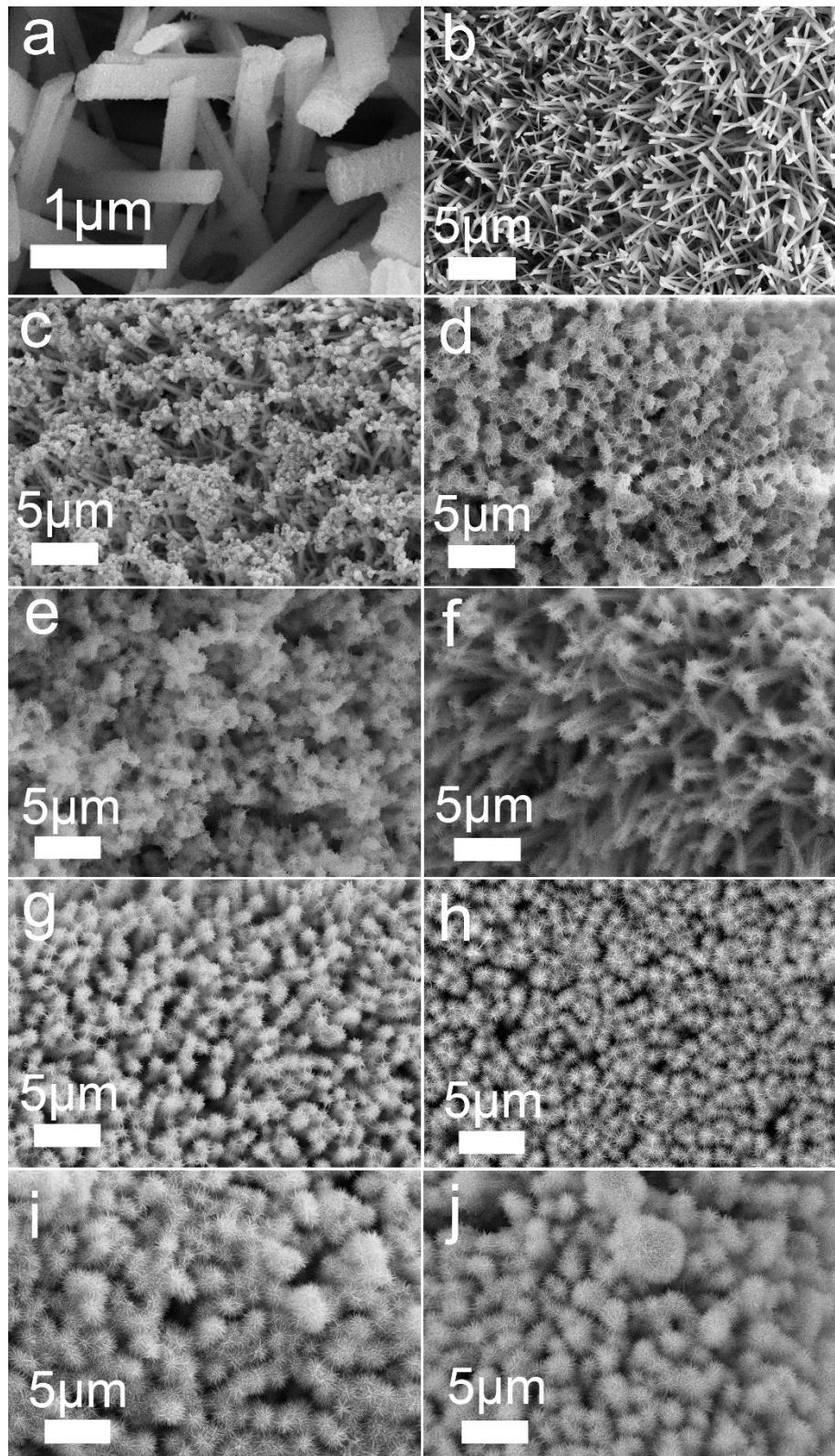
Fig. S7 SEM images of NiCo-precursor/ $\text{Cu}(\text{OH})_2/\text{Cu}$  prepared with different hydrothermal reaction time: (a, b) 0.5 h, (c) 1 h, (d) 2 h, (e) 3 h, (f) 4 h, (g) 5 h, (h) 6 h, (i) 7 h, (j) 8 h.
