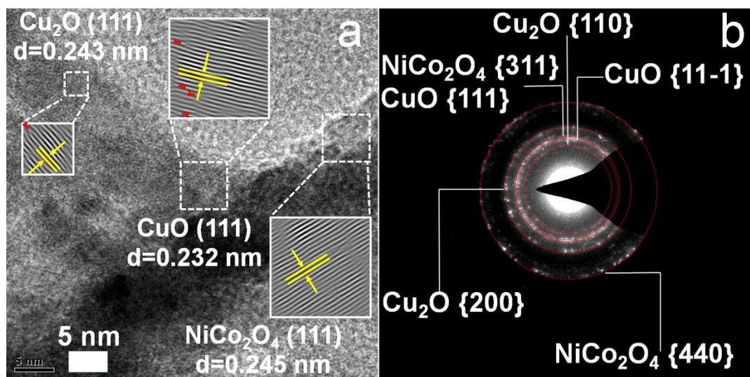
Fig. S23 (a) HRTEM image and (b) SAED pattern of  $\text{NiCo}_2\text{O}_4/\text{Cu}_x\text{O}/\text{Cu}$  after overall water splitting reaction in KOH (1 M) solution for 30 h.
