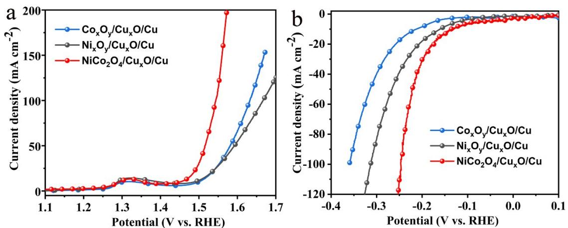
Fig. S19. LSV curves of (a) OER and (b) HER for  $\text{NiCo}_2\text{O}_4/\text{Cu}_x\text{O}/\text{Cu}$ ,  $\text{Co}_x\text{O}_y/\text{Cu}_x\text{O}/\text{Cu}$ , and  $\text{Ni}_x\text{O}_y/\text{Cu}_x\text{O}/\text{Cu}$ .
