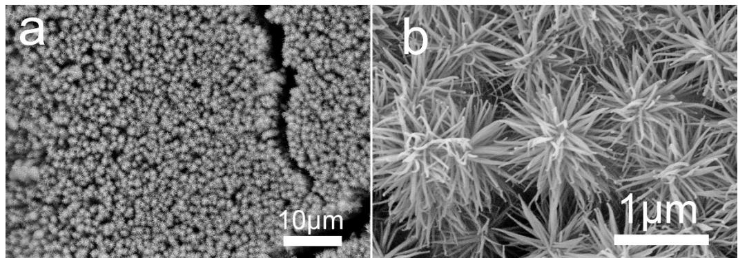
Fig. S6 (a) Low and (b) high magnification SEM images of NiCo<sub>2</sub>O<sub>4</sub>/Cu<sub>x</sub>O/Cu.
