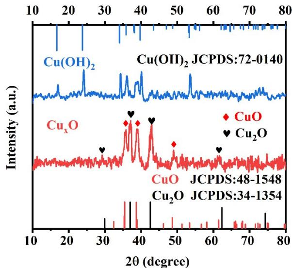
Fig. S10 The XRD patterns of the  $\text{Cu}(\text{OH})_2$  and  $\text{Cu}_x\text{O}$  scraped off the substrate carefully.
