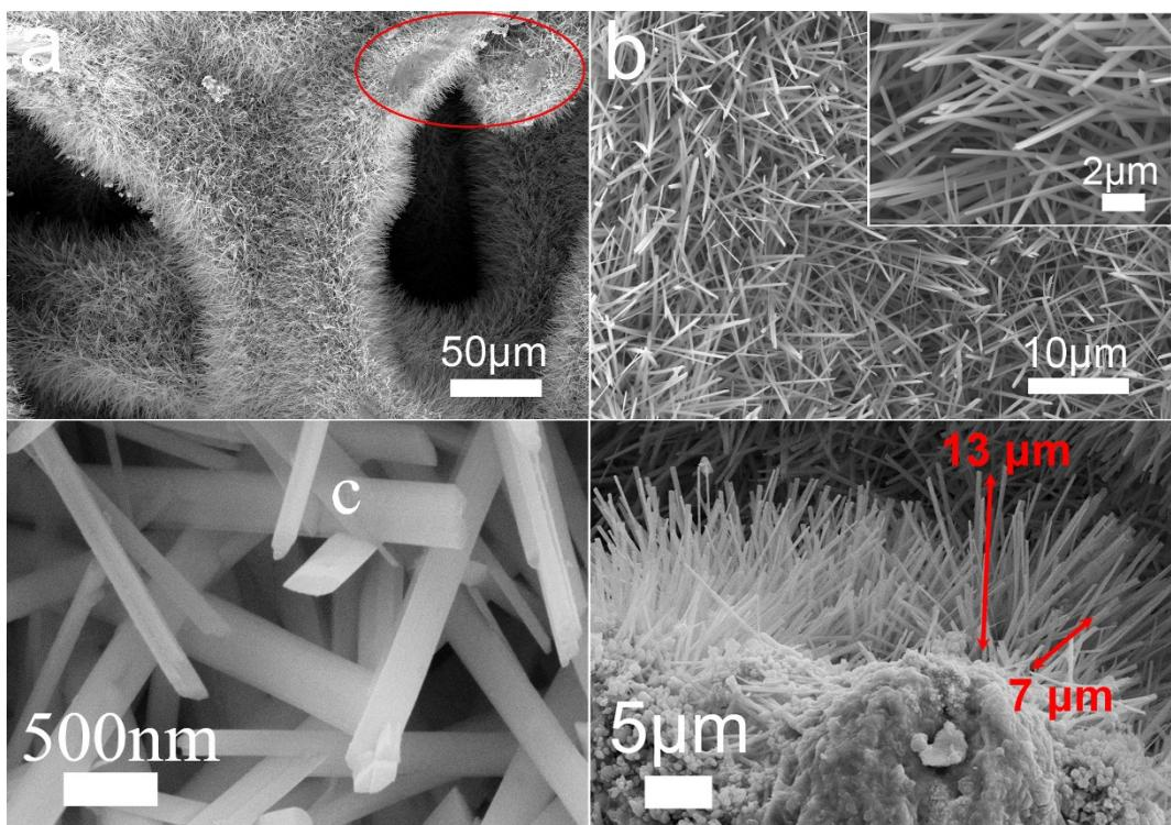
Fig. S1 (a-b) Low, (c) high magnification SEM images and (d) cross-section SEM image. of  $\text{Cu}(\text{OH})_2/\text{Cu}$ . The region enclosed by the red circles is made by pressing  $\text{Cu}(\text{OH})_2/\text{Cu}$  on the conductive adhesive with tweezers.
