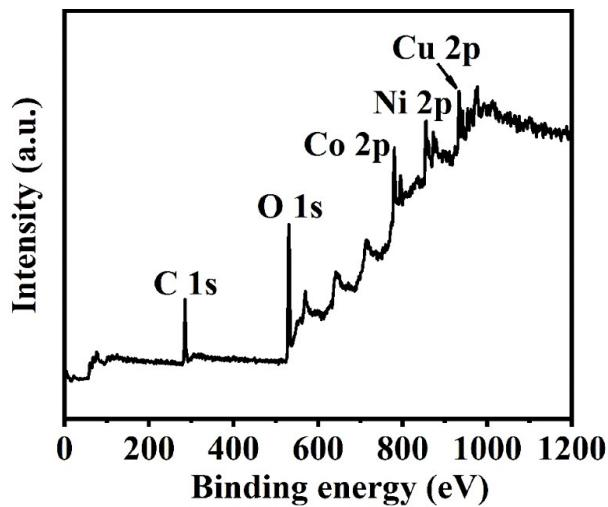
Fig. S12 Survey XPS spectra of  $\text{NiCo}_2\text{O}_4/\text{Cu}_x\text{O}/\text{Cu}$ .
