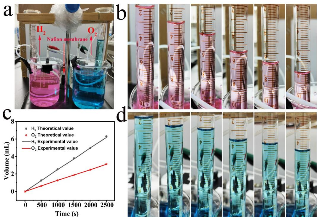
Fig. S16 Faradaic efficiency evaluated by the drainage method: (a) Device of drainage method. (b)  $H_2$  and (d)  $O_2$  collected at 0, 500, 1000, 1500, 2000, 2500 s. (c) The volume of  $H_2$  and  $O_2$  as a function of time.
