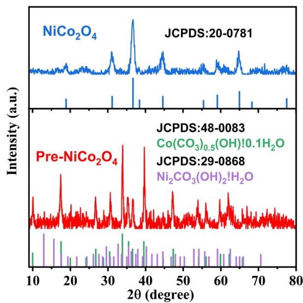
Fig. S11 The XRD patterns of the NiCo-precursor and  $\text{NiCo}_2\text{O}_4$  scraped off the substrate carefully.
