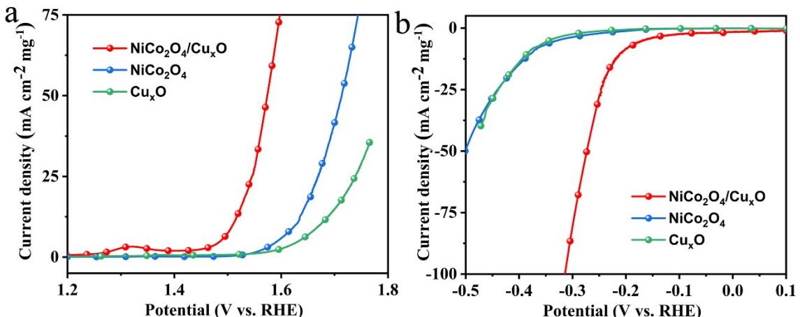
Fig. S14 The mass activity of the catalysts: (a) OER and (b) HER. The mass loadings are 4.10  $\text{mg cm}^{-2}$  for  $\text{NiCo}_2\text{O}_4/\text{Cu}_x\text{O}/\text{Cu}$ , 2.90  $\text{mg cm}^{-2}$  for  $\text{NiCo}_2\text{O}_4/\text{Cu}$ , and 3.57  $\text{mg cm}^{-2}$  for  $\text{Cu}_x\text{O}/\text{Cu}$ , respectively.
