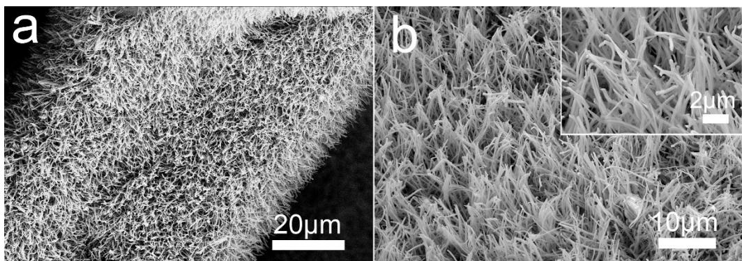
Fig. S2 (a) Low and (b) high magnification SEM images of  $\text{Cu}_x\text{O}/\text{Cu}$ .
