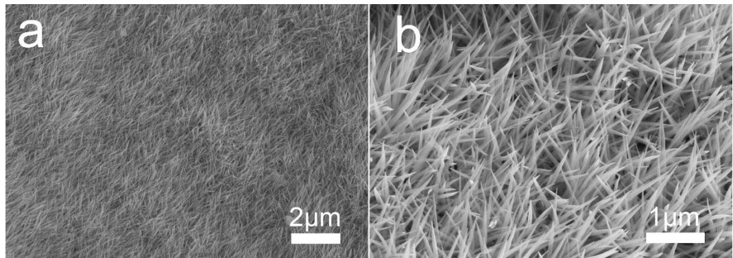
Fig. S4 (a) Low and (b) high magnification SEM images of NiCo<sub>2</sub>O<sub>4</sub>/Cu.
