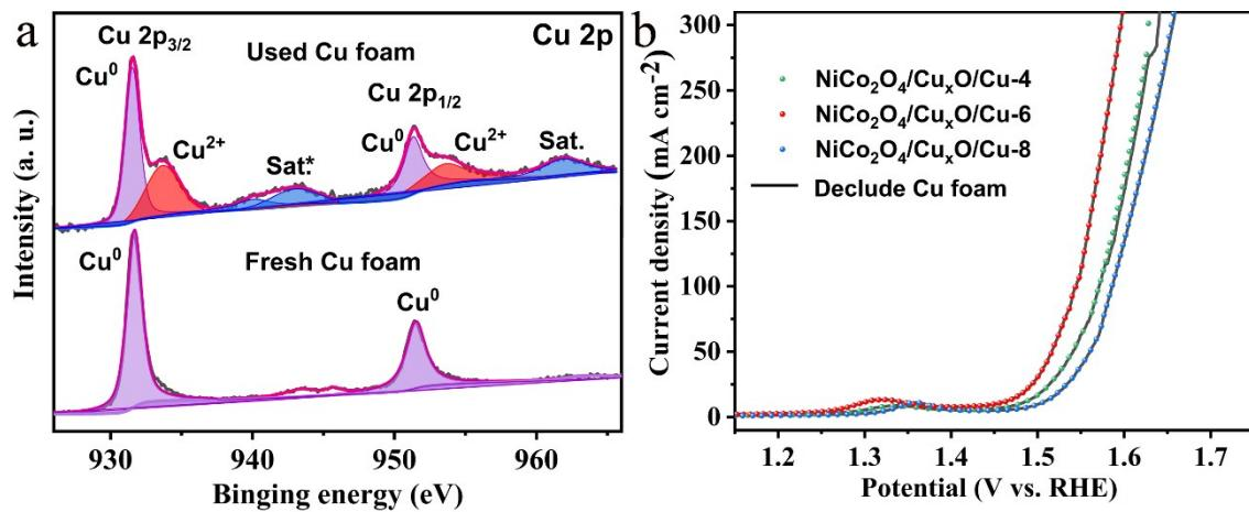
Fig. S13 (a) High-resolution XPS spectra of Cu 2p of Cu foam before and after i~t test (1.65 V vs. RHE) for 1 h. (b) LSV curves of  $\text{NiCo}_2\text{O}_4/\text{Cu}_x\text{O}/\text{Cu}-4/6/8$  before and after deducting the current of Cu foam.
