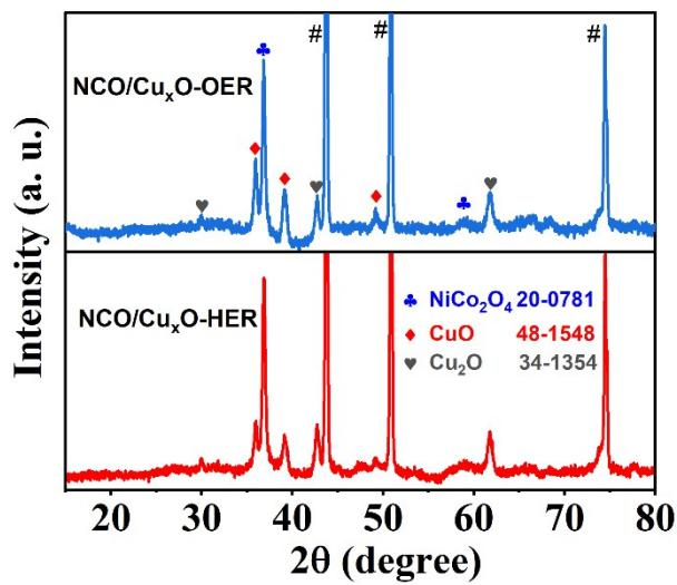
Fig. S24 XRD patterns of NiCo<sub>2</sub>O<sub>4</sub>/Cu<sub>x</sub>O/Cu after HER for 150 h and OER for 125 h in KOH (1 M) solution.
