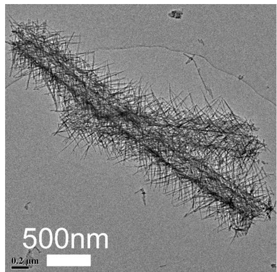
Fig. S22 TEM image of  $\text{NiCo}_2\text{O}_4/\text{Cu}_x\text{O}$  after overall water splitting reaction in KOH (1 M) solution for 30 h.
