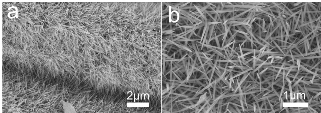
Fig. S3 (a) Low and (b) high magnification SEM images of NiCo-precursor/Cu.
