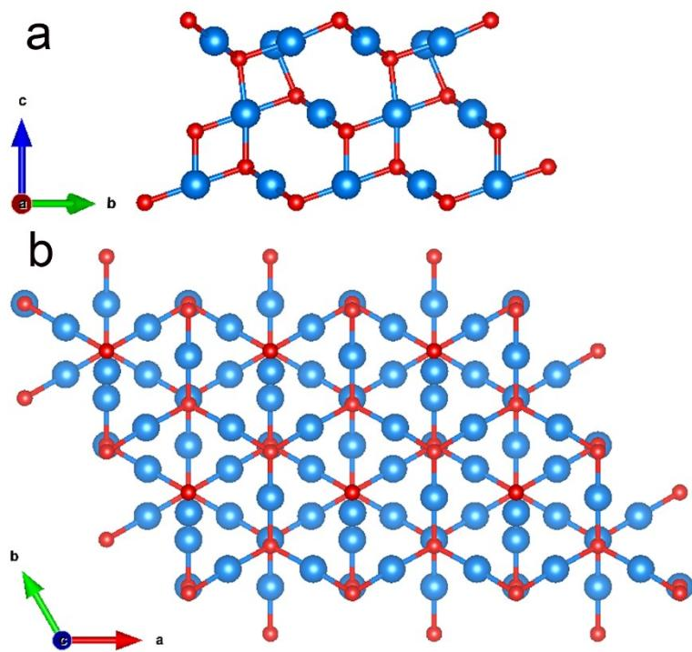
Fig. S29 DFT-optimized structure of Cu<sub>2</sub>O (111) in (a) the main view and (b) top view.
