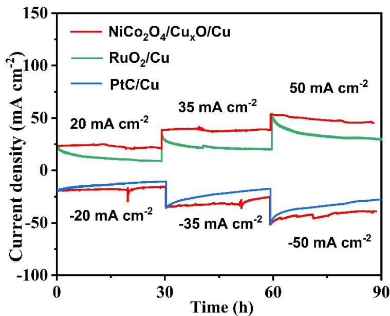
Fig. S20 Multipotentiometry measurement for catalysts in KOH (1 M) solution. The two current fluctuations of  $\text{NiCo}_2\text{O}_4/\text{Cu}_x\text{O}/\text{Cu}$  in HER (~20 h and ~51 h) are caused by the replenishment of the internal filling solution of the reference electrode.
