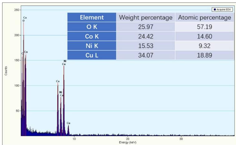
Fig. S8 EDS spectrum of  $\text{NiCo}_2\text{O}_4/\text{Cu}_x\text{O}$ . C is attributed to the carbon support film in the copper mesh.
