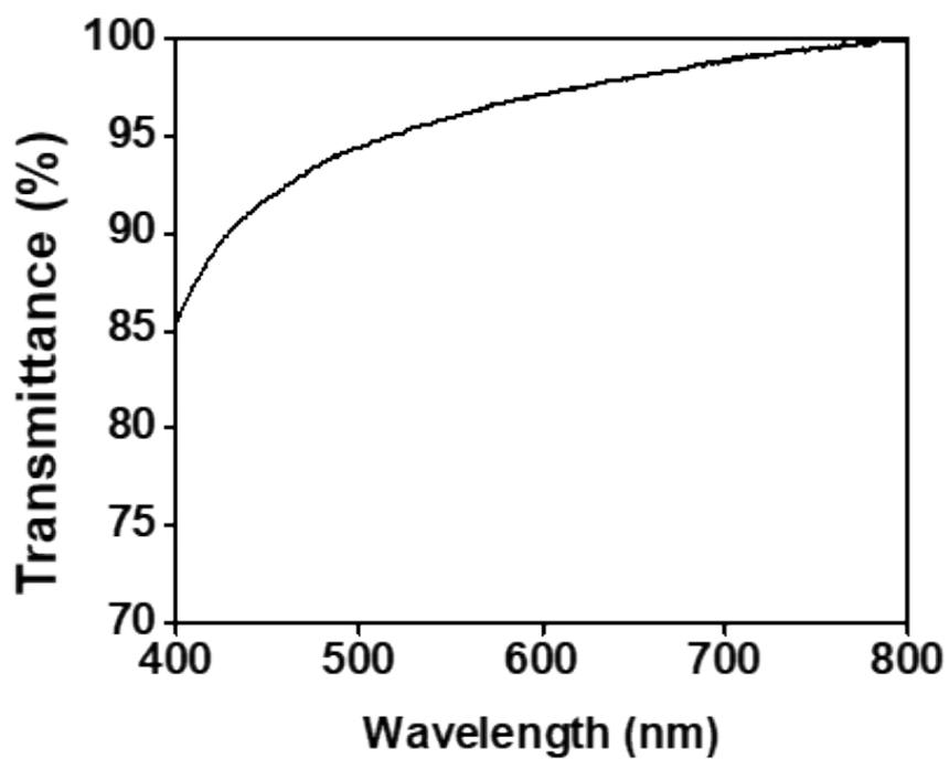
**Fig. S3** UV-vis transmission spectrum of NCB-PUU coatings without underlying substrate.
