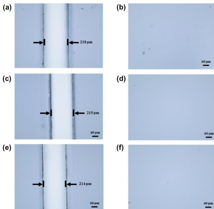
**Fig. S10** Optical microscope images of the NCB-PUU sheet during three cycles of cutting/healing process.
