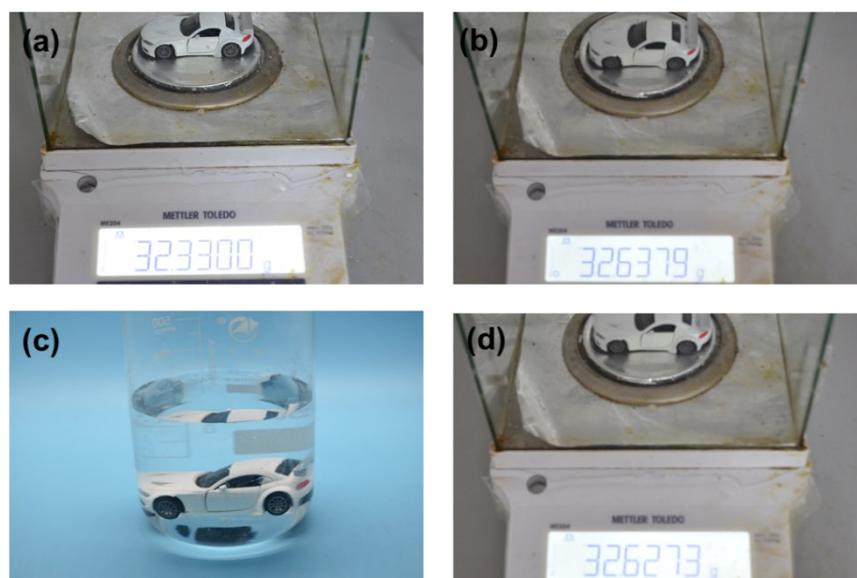
**Fig. S13** Mass change of NCB-PUU coating deposited on a model car. (a) As-prepared coating. (b) Immersed in water for 24 h. (c) After immersion in water and being dried.
