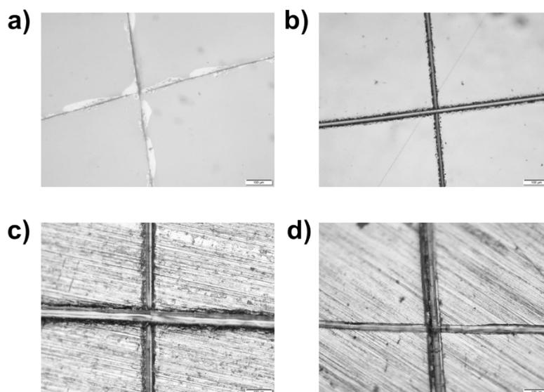
**Fig. S9** Optical microscope images of the NCB-PUU coatings after adhesion test on different substrates. (a) glass, (b) stainless steel, (c) aluminum and (d) copper.
