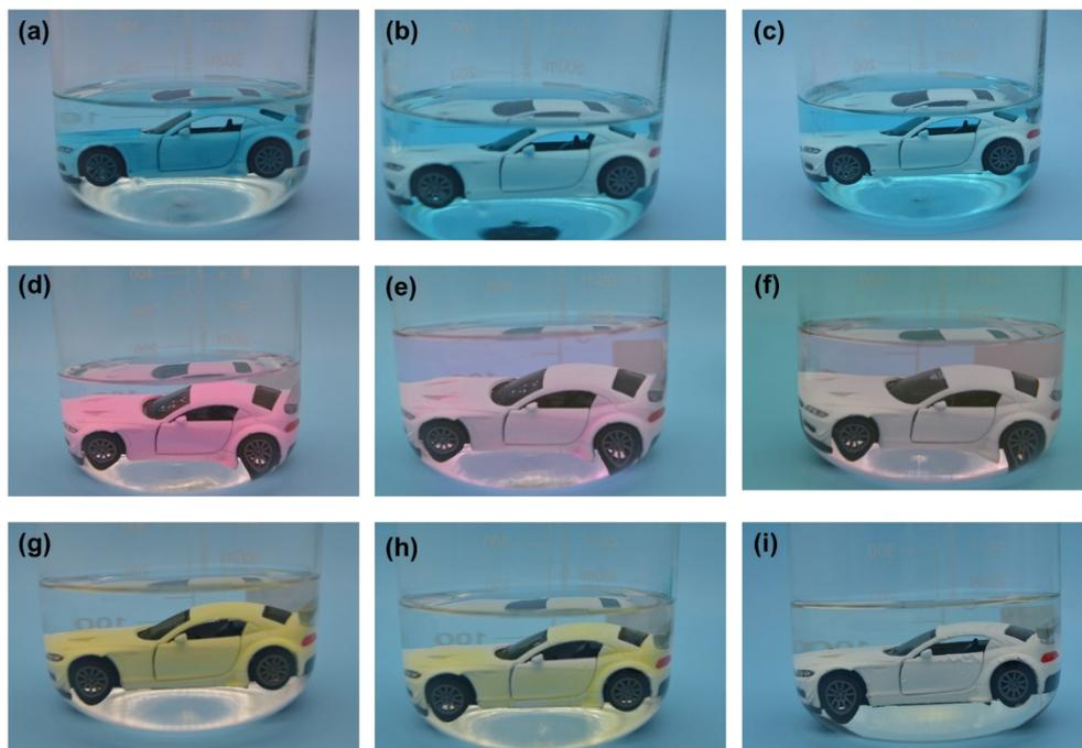
**Fig. S12** Digital images of the model car with different colored NCB-PUU coating which was immersed in ethanol for 0 h (a, d, g), 3 h (b, e, h) and 6 h (c, f, i).
