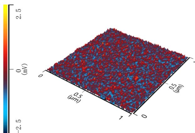
**Fig. S7** AFM-IR chemical image shows the distribution of the C=O groups in the separated microphases (red). The AFM-IR image was collected at 1711  $\text{cm}^{-1}$ .
