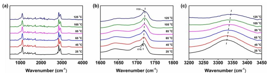
**Fig. S6** Variable temperature FT-IR spectra of NCB-PUU in the ranges of 500-4000  $\text{cm}^{-1}$  (a), 1600-1800  $\text{cm}^{-1}$  (b), and 3200-3450  $\text{cm}^{-1}$  (c).
