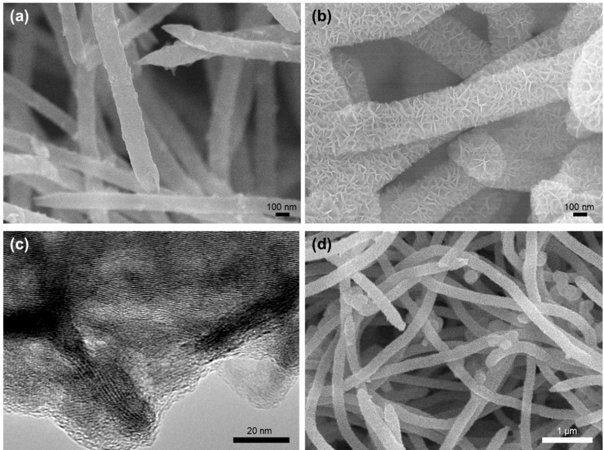
**Figure S2.** SEM image of (a) P-CNT and (b) MO-CNT, (c) TEM image of MO-CNT showing graphitic layer of CNT and polycrystalline grains of MnO<sub>2</sub>, (d) SEM image of MO-CNT showing porous features after MnO<sub>2</sub> decoration on CNT.
