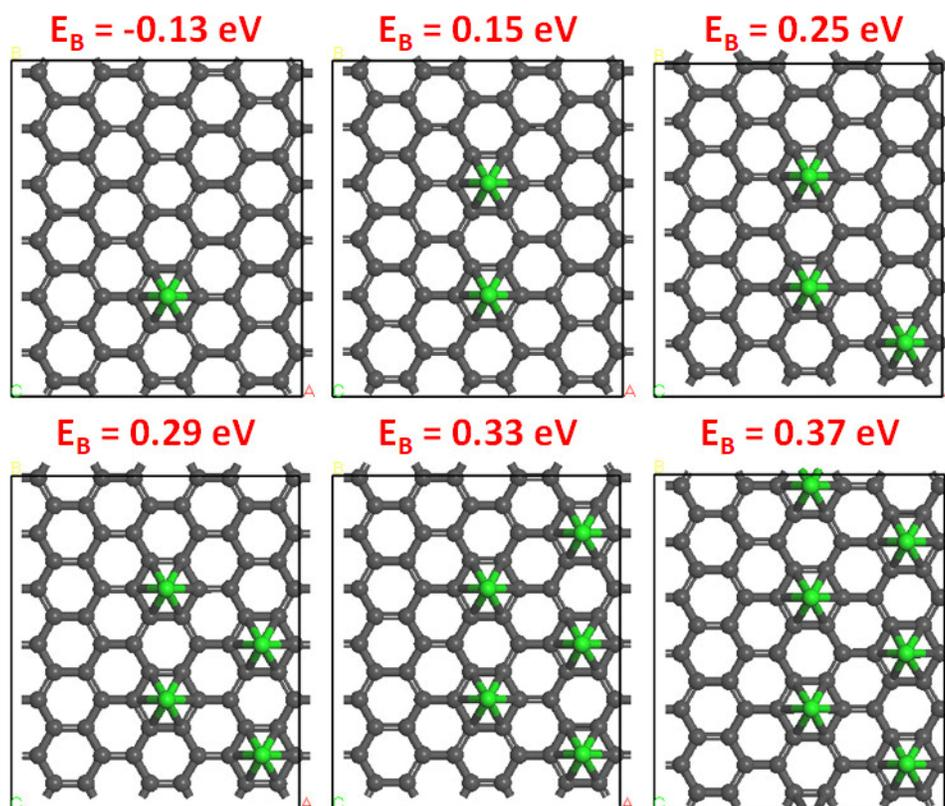
**Figure S11.** The optimized geometry and binding energy ( $E_B$ ) of six Li atoms deposited on a bare graphene structure. Color code: black and green spheres represent C and Li atoms, respectively.
