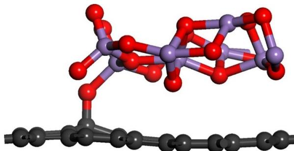
**Figure S4.** Geometry optimization of the CNT/MnO<sub>2</sub> system according to density functional theory (DFT) calculations at 0 K. Color code: black, red, and purple spheres represent C, O and Mn atoms, respectively.
