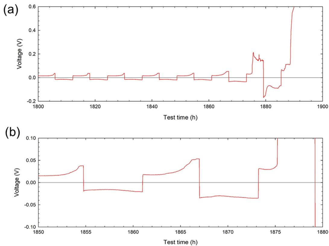
**Figure S7.** Voltage profiles of MO-CNT (vs Li metal counter electrode) near the failure cycles.
