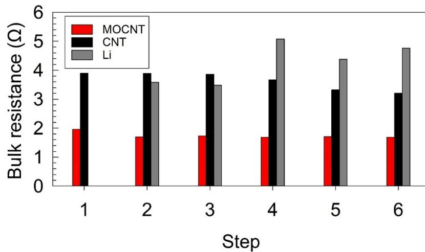
**Figure S9.** Bulk resistance at the stages of (1) before lithiation, (2) after full lithiation, (3) plating of Li up to 8 mAh/cm<sup>2</sup>, after a stripping/plating cycle with capacities of (4) 1 mAh/cm<sup>2</sup>, (5) 3 mAh/cm<sup>2</sup>, and (6) 6 mAh/cm<sup>2</sup>.
