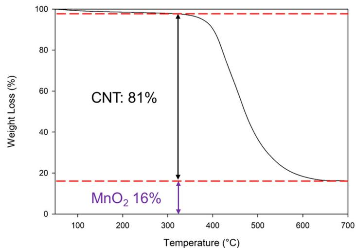
**Figure S3.** Thermogravimetric analysis (TGA) result of MO-CNT.
