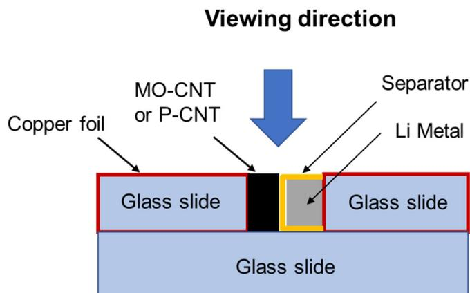
**Figure S5.** Schematic of the in-operando pouch cell setup.
