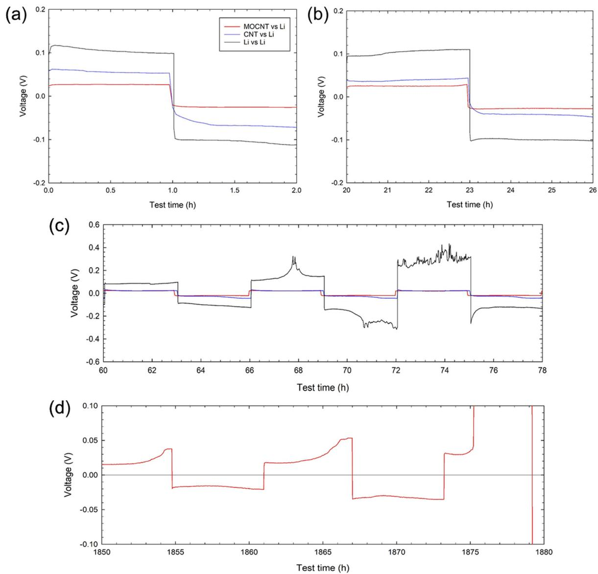
**Figure S6.** Voltage profiles of MO-CNT, P-CNT, and Li metal (with Li metal counter electrodes).
