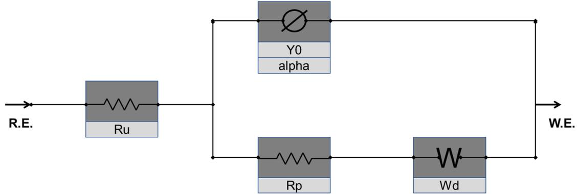
**Figure S1.** Equivalent circuit for EIS data.
