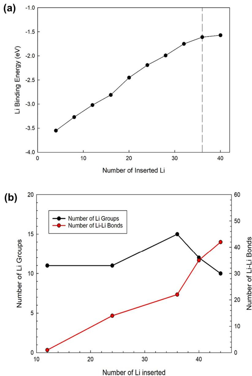
**Figure S10.** (a) Binding energy (eV) profile of the sequential Li insertion in the CNT/MnO<sub>2</sub> system. (b) Number of isolated Li groups and number of Li-Li bonds as a function of Li inserted in the system.
