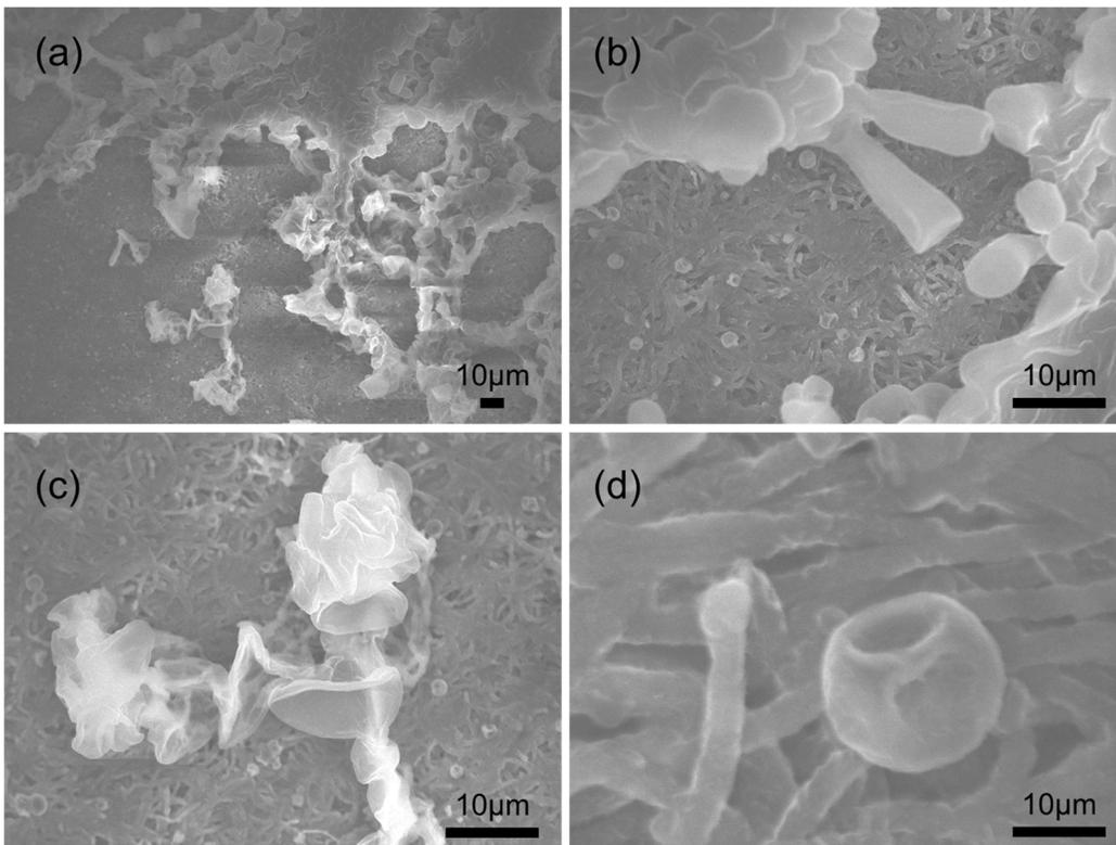
**Figure S13.** SEM images of Li dendrites deposited on P-CNT surface.
