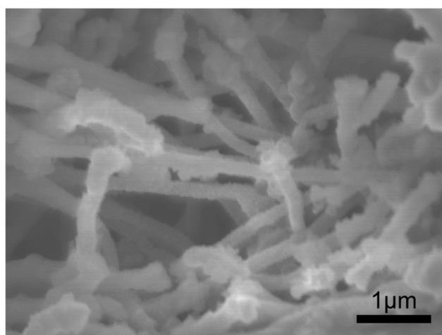
**Figure S12.** A SEM image of a cross-section of MO-CNT electrode after cycling.
