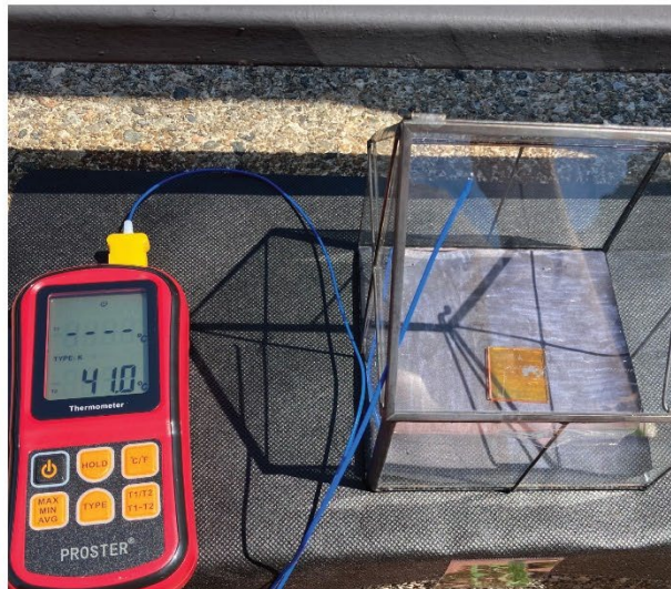
Fig. S5 (a) Surface temperature measurement of the greenhouse. Ambient temperature was 28 °C, and the temperature measured on black and white area was 40.2 °C and 35.5 °C, respectively. (b) Another measurement showing the surface temperature inside the greenhouse. Ambient temperature was 31 °C, and the temperature measured on the black surface was 41 °C. The film of 1-E melted in the greenhouse.
