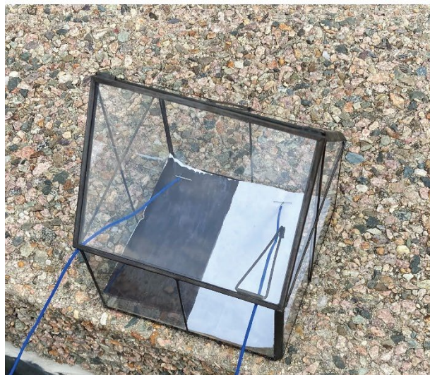
Fig. S5 (a) Surface temperature measurement of the greenhouse. Ambient temperature was 28 °C, and the temperature measured on black and white area was 40.2 °C and 35.5 °C, respectively. (b) Another measurement showing the surface temperature inside the greenhouse. Ambient temperature was 31 °C, and the temperature measured on the black surface was 41 °C. The film of 1-E melted in the greenhouse.
